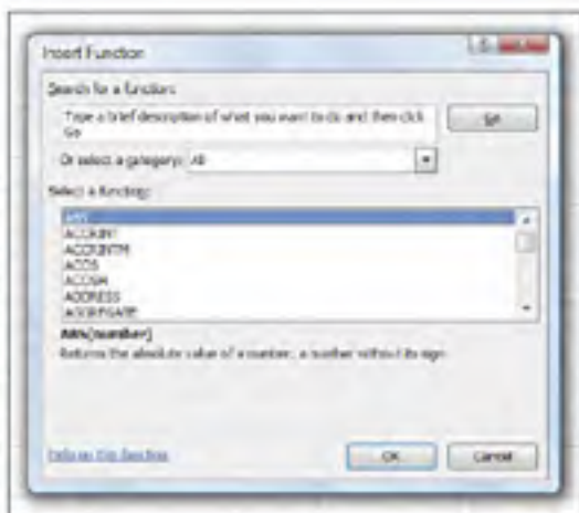
Figure 2-1: Use the Insert Function dialog box to easily enter func- tions in a worksheet.
