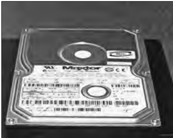
Figure 6-1: The classic magnetic- media hard drive.
