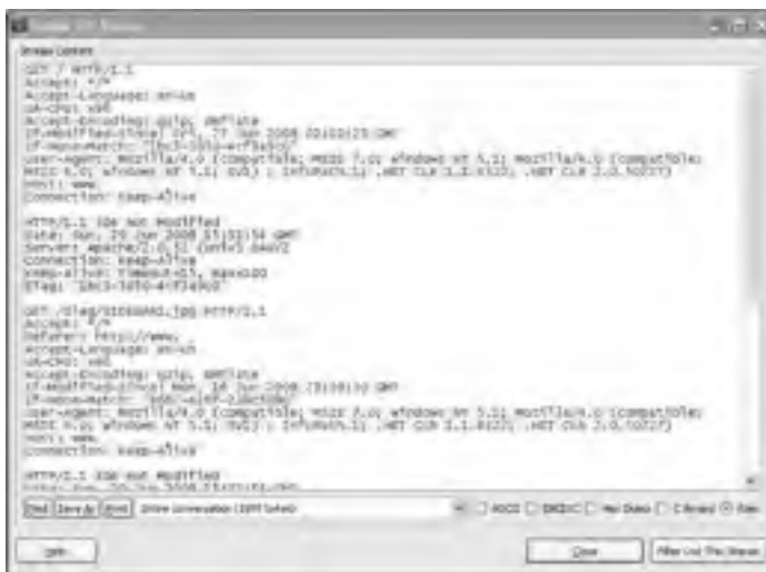
Figure 13-10: Reassembled data stream based on protocols and sequence numbers.
