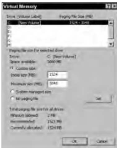
Figure 9-10: Virtual memory control settings in Microsoft Windows.
