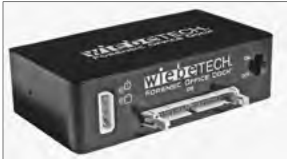
Figure 6-9: Desktop write block device.
