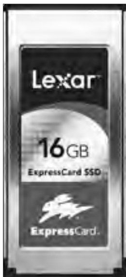
Figure 6-2: A solid-state drive.
