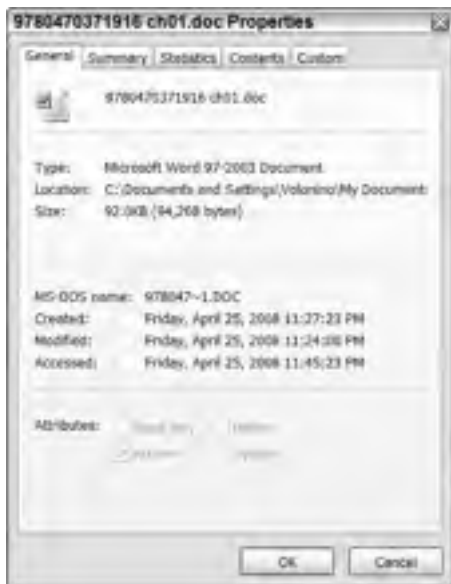
Figure 1-2: Metadata created automatically by Word software.
