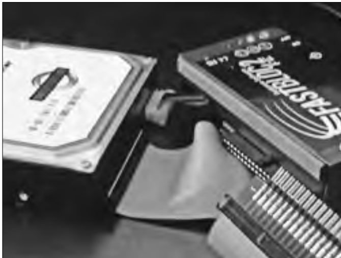
Figure 6-11: Data cable and power cable connected to the acquisition hard drive.
