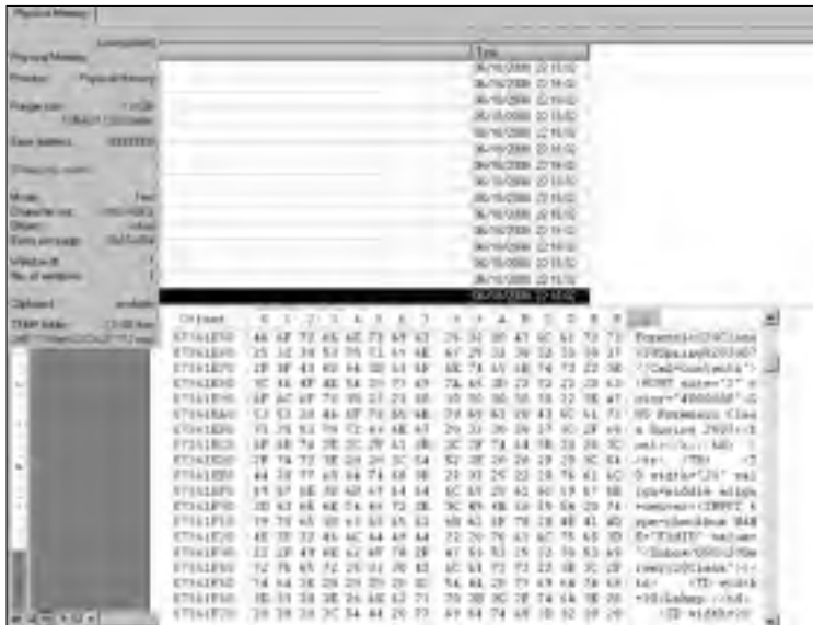
Figure 10-10: Contents of RAM found after a RAM dump.
