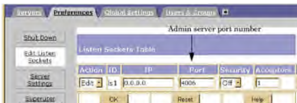
Figure 5.6. Administration server listener port.
