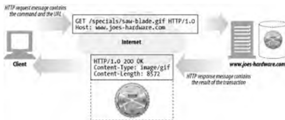
Figure 3-4. An HTTP transaction has request and response messages
