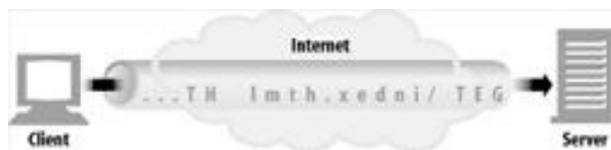
Figure 4-2. TCP carries HTTP data in order, and without corruption
