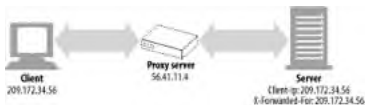
Figure 11-1. Proxies can add extension headers to pass along the original client IP address
