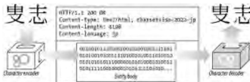
Figure 16-7. Character encoding scheme encodes character codes into bits and back again
