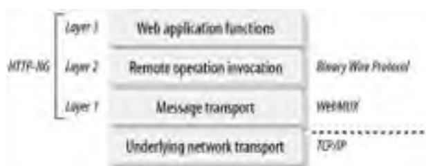
Figure 10-1. HTTP-NG separates functions into layers
