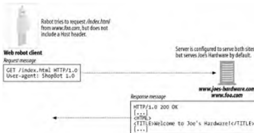
Figure 9-5. Example of virtual docroots causing trouble if no Host header is sent with the request
