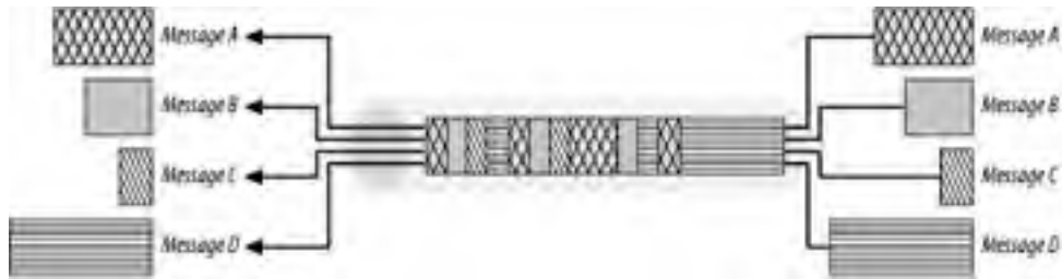
Figure 10-2. WebMUX can multiplex multiple messages over a single connection
