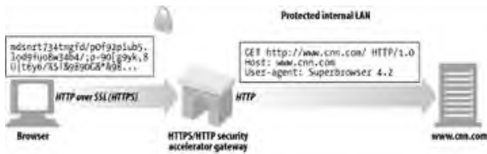
Figure 8-7. HTTPS/HTTP security accelerator gateway
