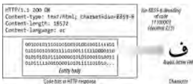
Figure 16-1. The charset parameter tells the client how to go from bits to characters
