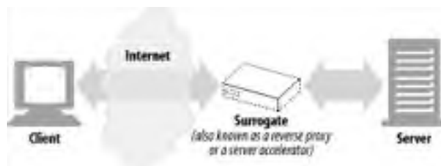
Figure 6-7. Proxy application example: surrogate (in a server accelerator deployment)
