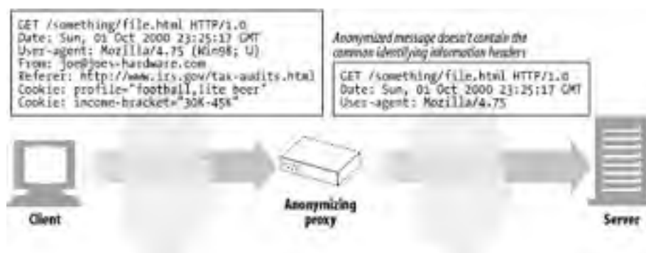
Figure 6-10. Proxy application example: anonymizer
