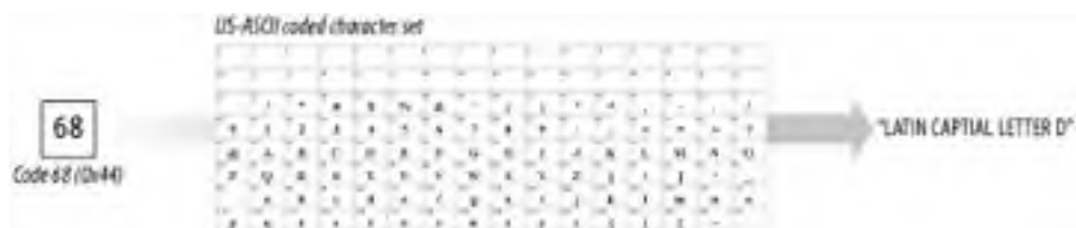
Figure 16-6. Coded character sets can be thought of as arrays that map numeric codes to characters
