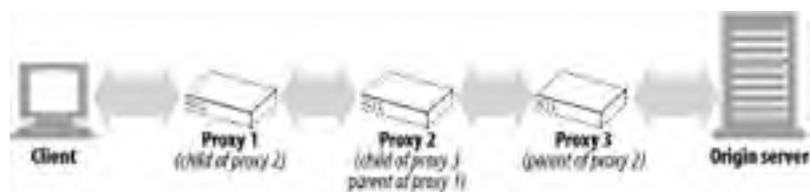
Figure 6-12. Three-level proxy hierarchy
