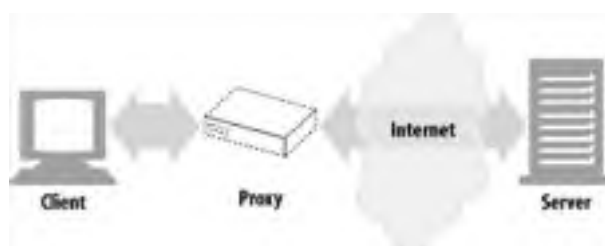
Figure 1-11. Proxies relay traffic between client and server
