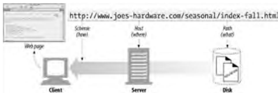
Figure 2-1. How URLs relate to browser, machine, server, and location on the server's filesystem
