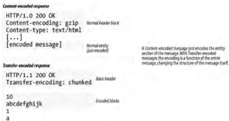
Figure 15-5. Content encodings versus transfer encodings
