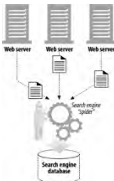
Figure 1-15. Automated search engine "spiders" are agents, fetching web pages around the world
