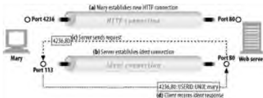
Figure 5-4. Using the ident protocol to determine HTTP client username
