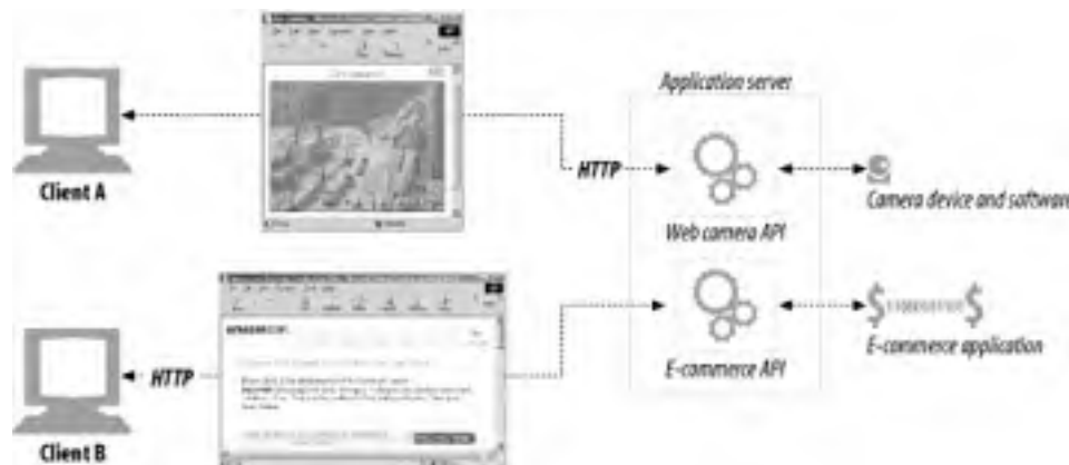
Figure 8-8. An application server connects HTTP clients to arbitrary backend applications
