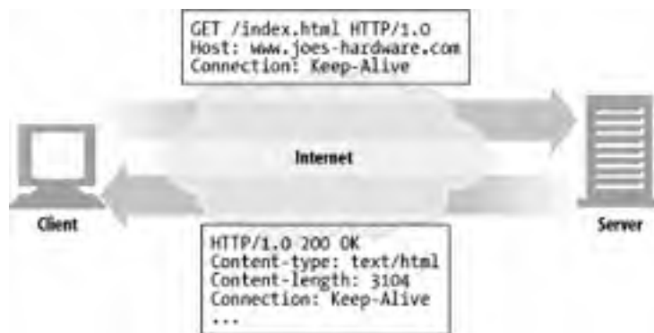
Figure 4-14. HTTP/1.0 keep-alive transaction header handshake
