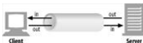
Figure 4-19. TCP connections are bidirectional
