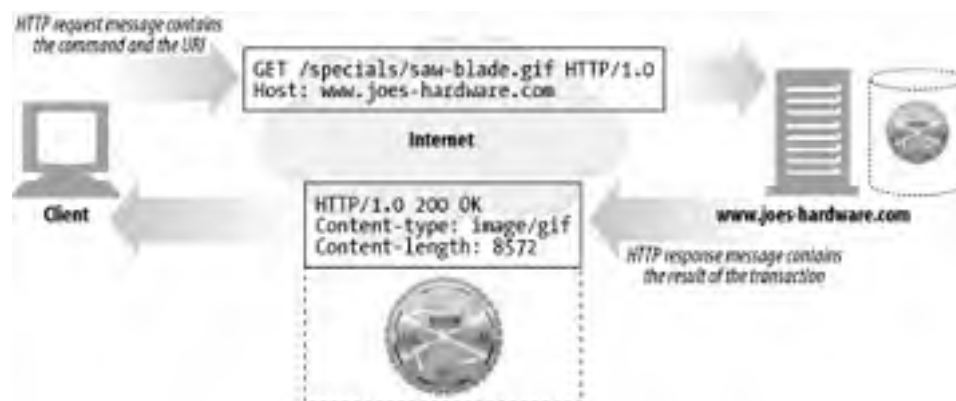
Figure 1-5. HTTP transactions consist of request and response messages
