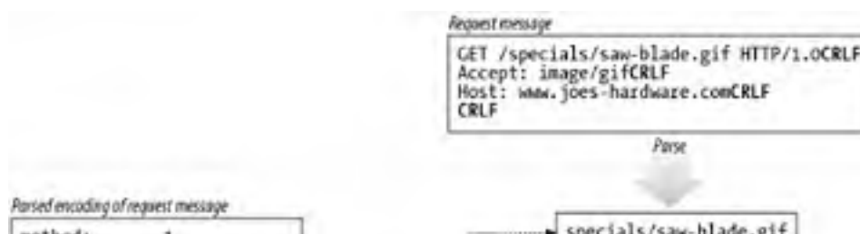
Figure 5-6. Parsing a request message into a convenient internal representation
