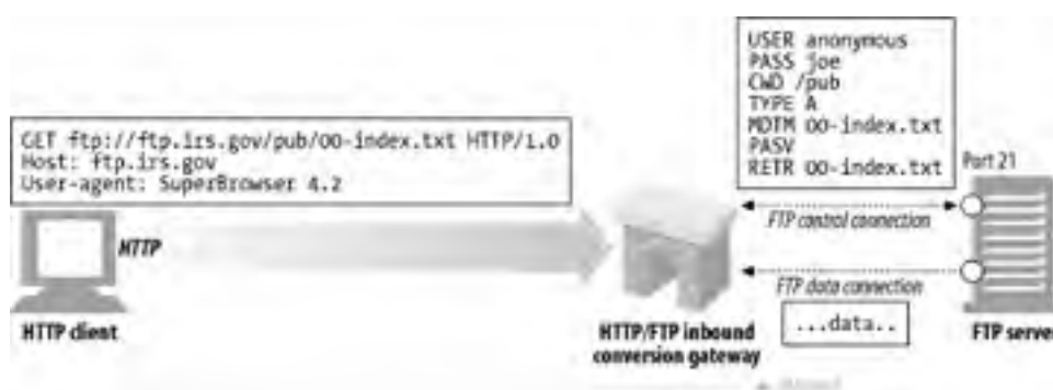
Figure 8-5. The HTTP/FTP gateway translates HTTP request into FTP requests
