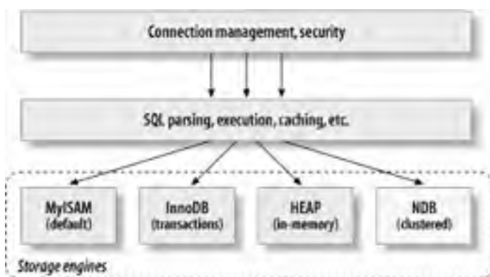
Figure 2-1. A logical view of MySQL's architecture
