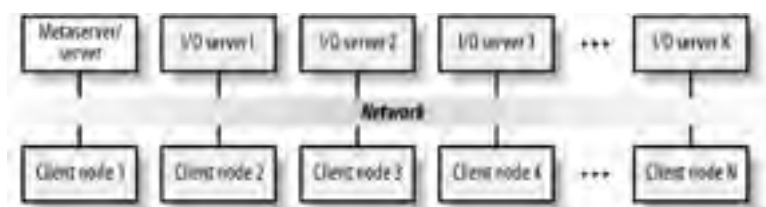
Figure 12-1. Internal cluster architecture
