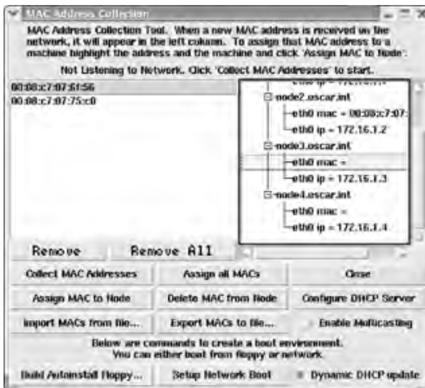
Figure 6-12. Setting up networking
