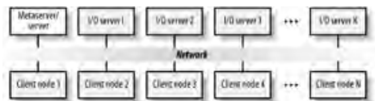
Figure 12-1. Internal cluster architecture
