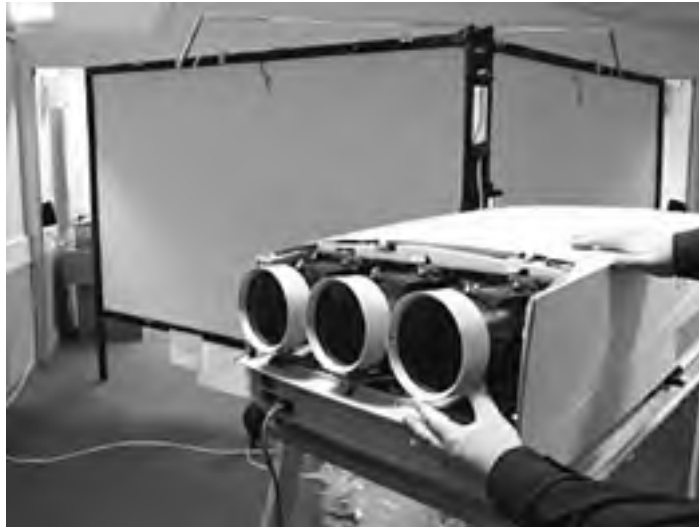
Figure 10.4. Torus Treadmill. (Photo courtesy of Dr. Hiroo Iwata, University of Tsukuba, Japan)
