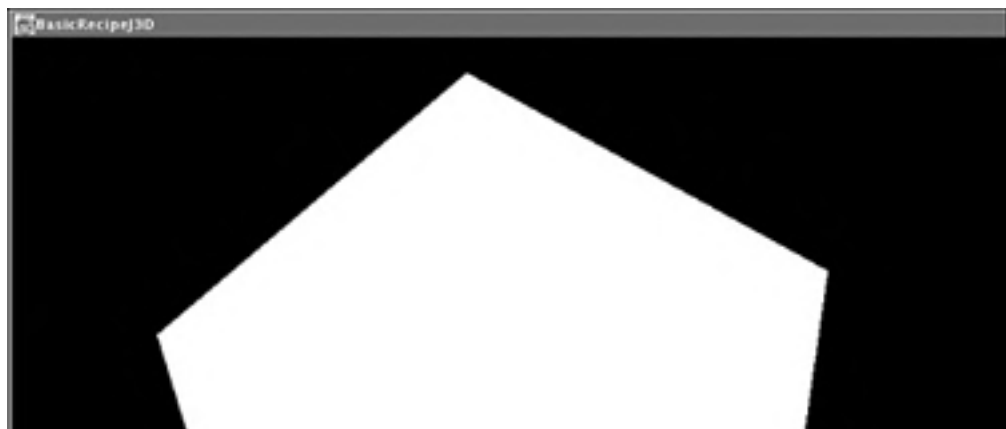
Figure 11.4. Screenshot from the application after adding and translating a second box using a TransformGroup .
