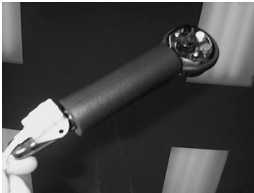
Figure 10.2. Haptic wand. (Photo courtesy of Jerry Roll, Michigan State University MIND Lab)
