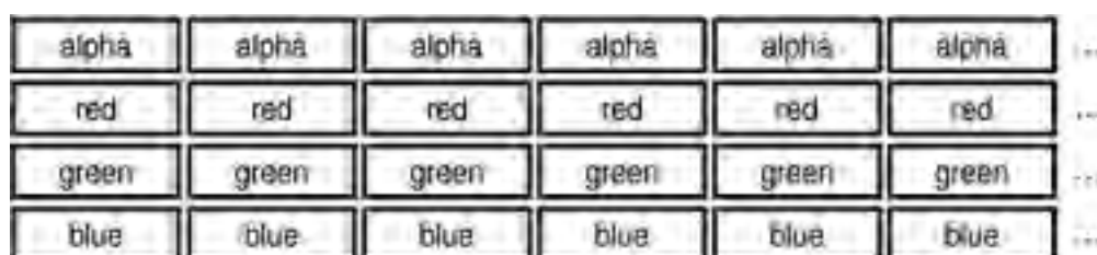
Figure 4.5. In the top byte array, each element represents the alpha sample from a different pixel. The red, green, and blue samples are held in three other arrays.
