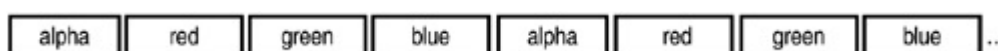
Figure 4.6. In this byte array, the different samples alternate within a single array.
