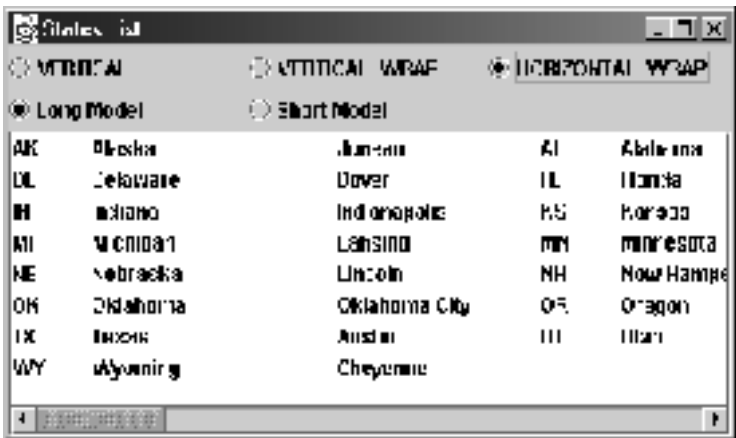
Figure 10.4 Long model and HORIZONTAL_WRAP cell layout
