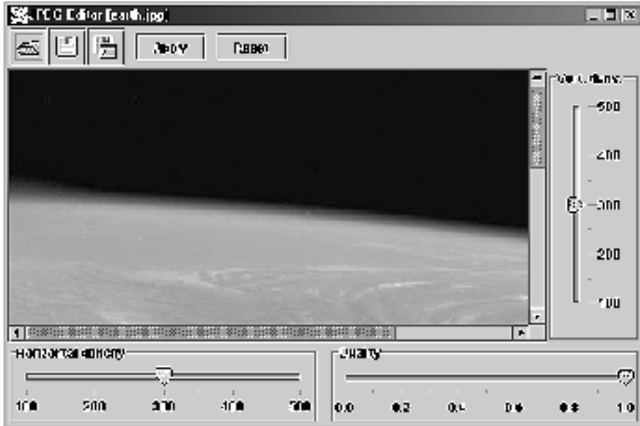
Figure 13.5 JPEGEditor showing a high-quality image of Earth (using JSliders with the “isFilled” client property)
