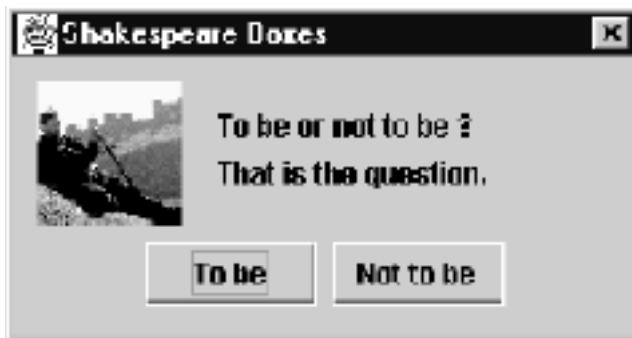
Figure 14.9 A JOptionPane with custom icon, message, and option button strings in a JDialog
