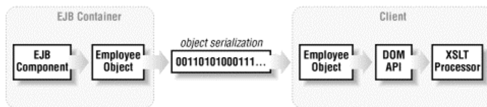
Figure 9-10. Generating XML on the client tier
