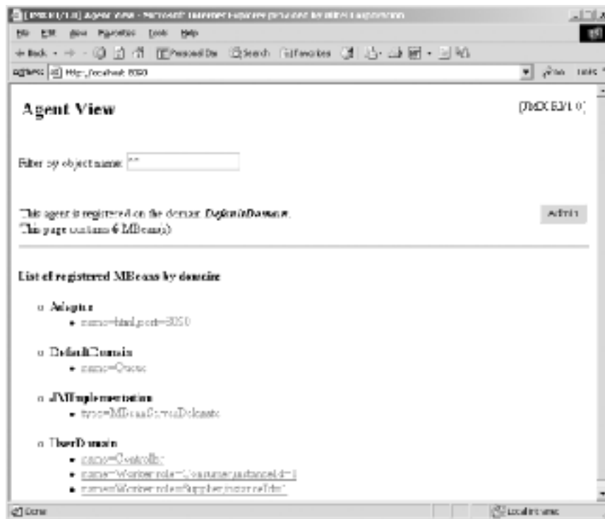
Figure 6-1. The management view of the MBean server when the no-argument version of createMBeanServer() is used
