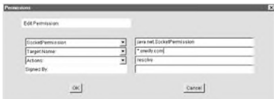
Figure 6-1. Using the Policy Tool to grant DNS resolution permission to all applets
