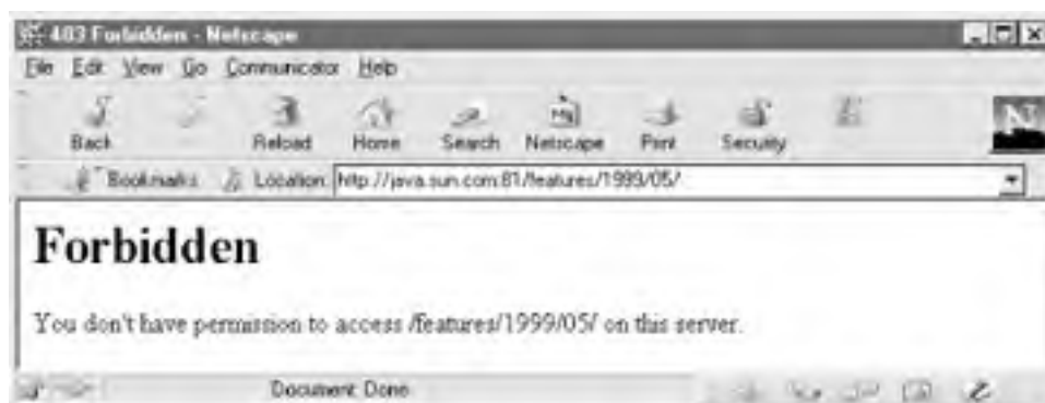
Figure 3-2. A web server configured to send a 403 error when no index file exists
