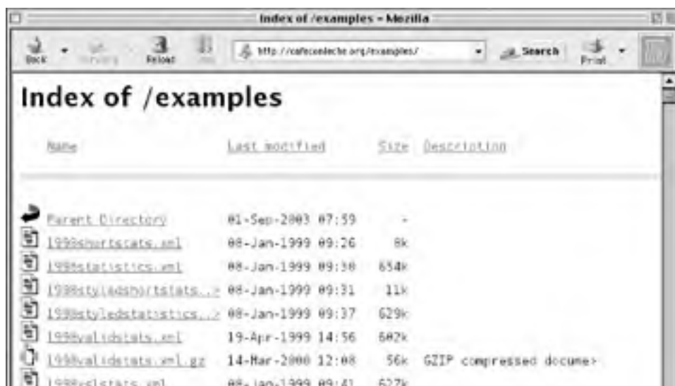
Figure 3-1. A web server configured to send a directory list when no index file exists
