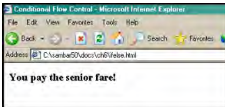
Figure 6.2. If the age was entered was greater than 55, this message is displayed.
