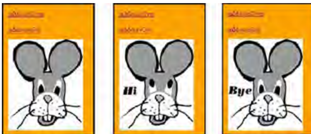
Figure 12.10. Original display (left), as the mouse moves over the link (middle), and as the mouse moves away from the link (right).
