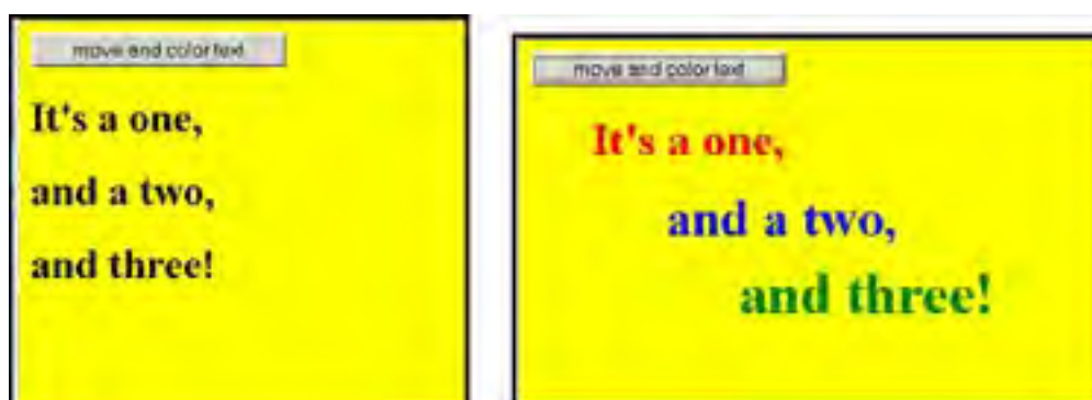
Figure 15.34. The initial appearance of the document (left); after clicking the button, the color, position, and size of the text is changed (right).
