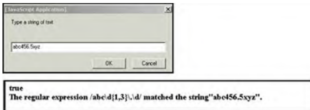
Figure 13.21. The user entered abc followed by between one and three numbers, followed by a literal period, and xyz (top); the entered string matched true (bottom).
