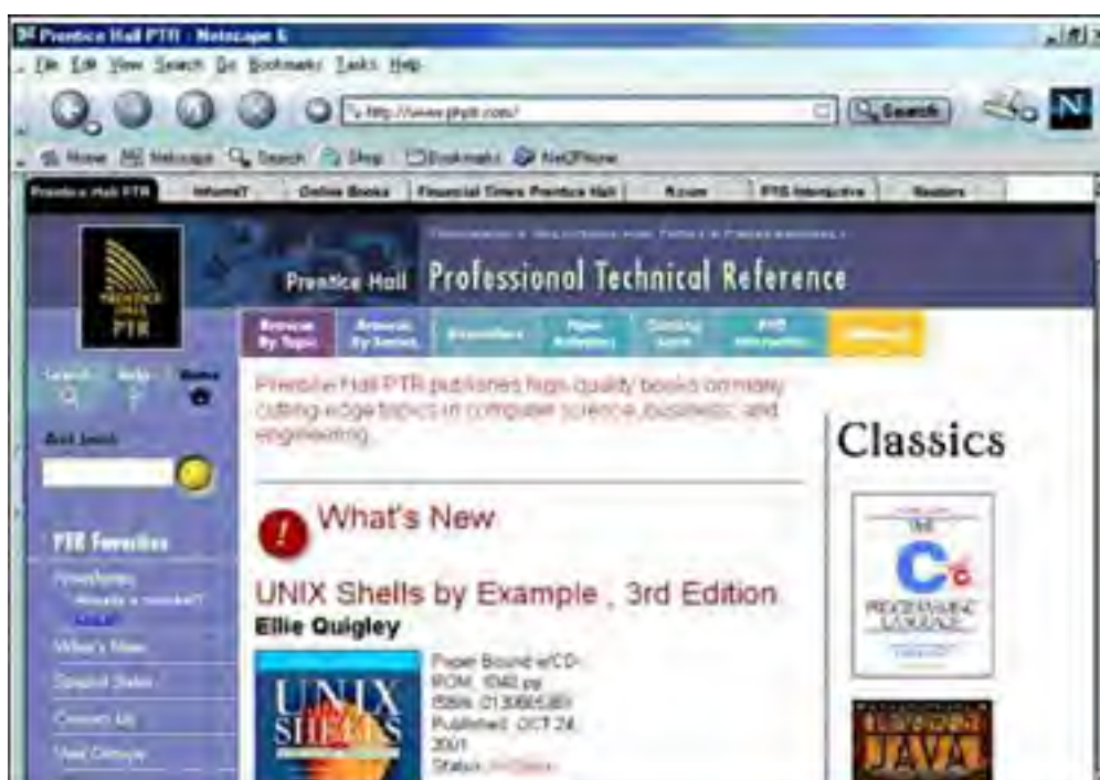
Figure 1.1. A dynamic Web page using JavaScript to give it life. For example, if the user rolls his mouse over any of the links or items in the navigation bars, those items will change color.
