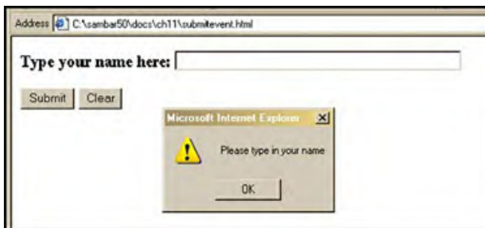
Figure 12.4. Using the onSubmit event and return values. If the return value is true the form is submitted; otherwise, it is stopped.
