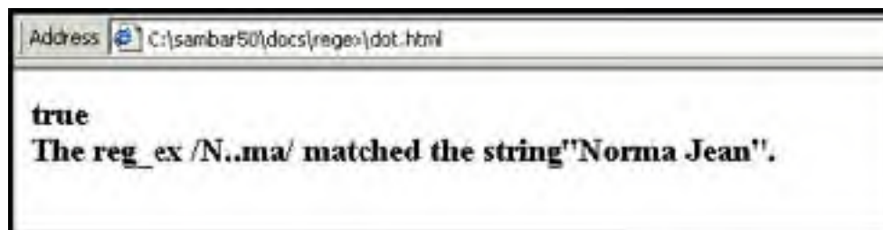
Figure 13.9. The user entered Norma Jean , an N followed by any 2 characters, and ma .
