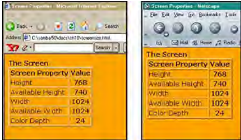
Figure 10.31. Tables showing properties of the screen object in Internet Explorer (left) and Netscape (right).
