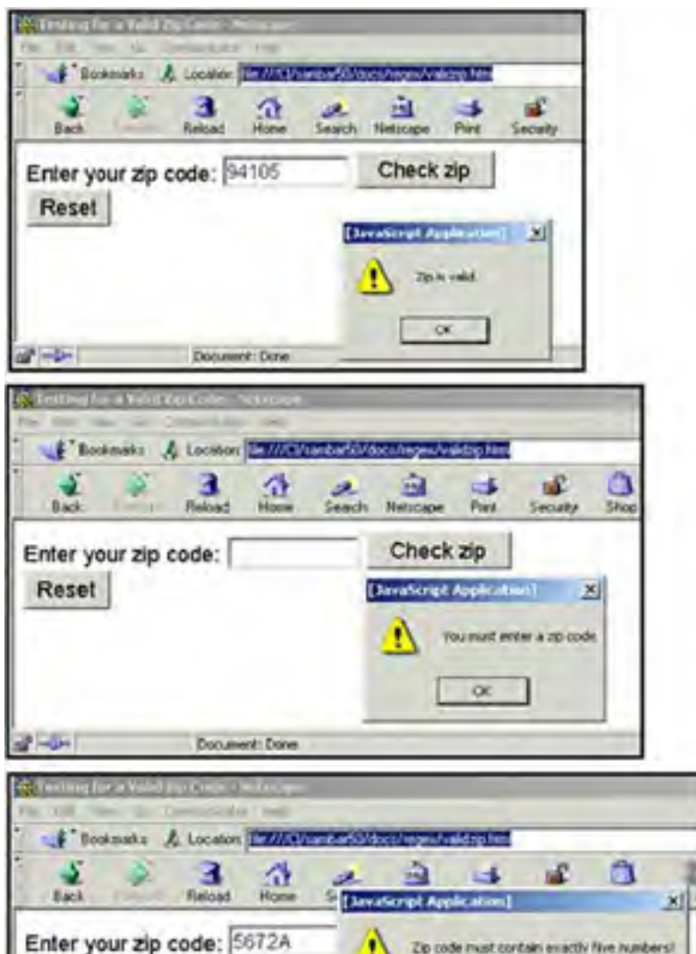
Figure 13.37. The user enters a five-digit zip code (top); the user enters nothing (middle); the user enters 4 digits and 1 letter (bottom).
