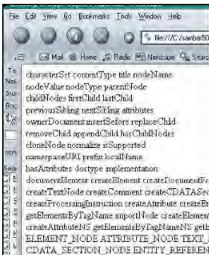
Figure 11.2. Using the for/in loop to display the properties of the document object.
