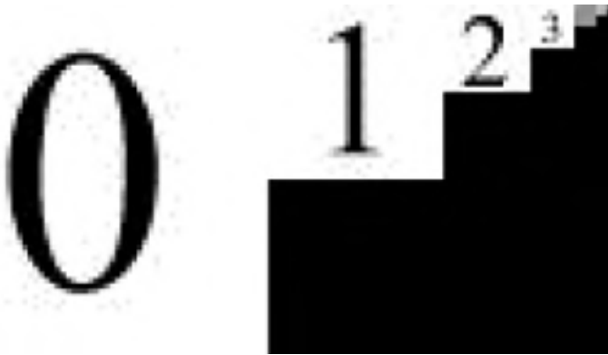
Figure 14.13 The seven texture images used in the AppearanceTest example to illustrate Java 3D MIPMAP support—64 x 64 pixels down to 1 x 1 pixels
