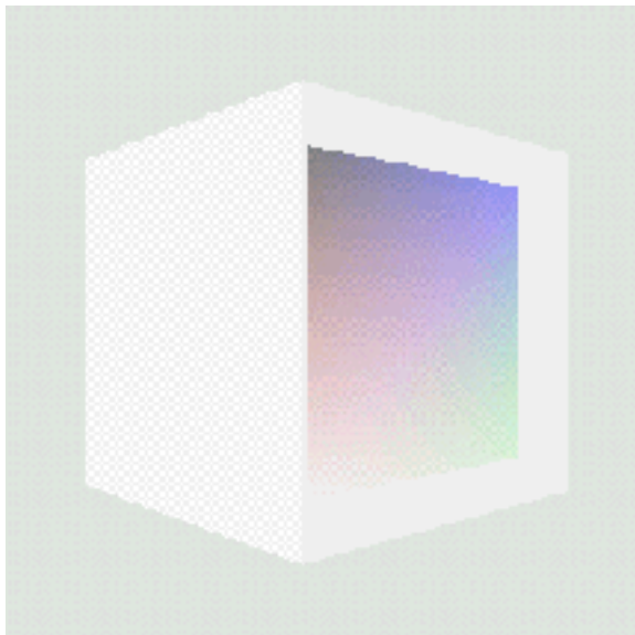
Figure 9.24 Coloring = null, Material = null. Transparency = 0.5—NICEST. When the Box is semitransparent, the problem with rendering order is not apparent because you can see the QuadArray through the Box
