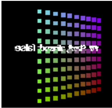
Figure 9.11 When rotated, nonantialiased points appear as squares aligned with the viewer
