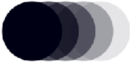
Figure 9.18 Five Sphere primitives with varying transparency, from left to right 100%, 70%, 50%, 30%, and 10%. All of the Spheres have the same color (black)
