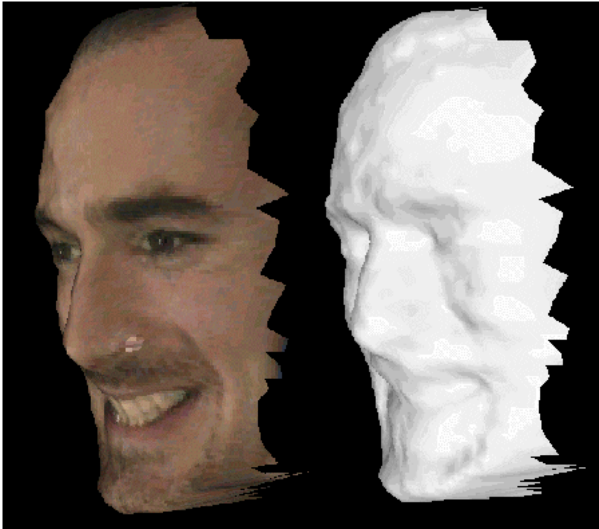
Figure 14.1 By applying a bitmap to the geometric model (left), very realistic results can be achieved even with a fairly coarse geometric mesh
