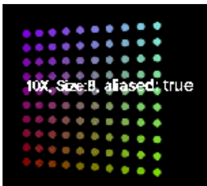
Figure 9.10 When rotated, antialiased points appear as spheres
