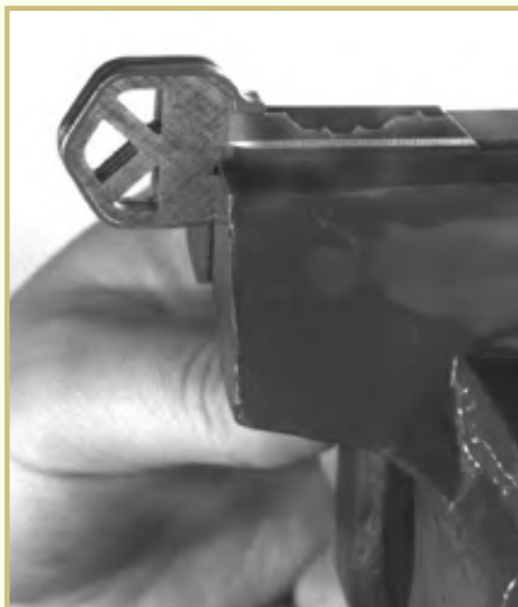
FIGURE 8 —Holding the duplicate and sample keys even in a vise is very important during key duplication.
