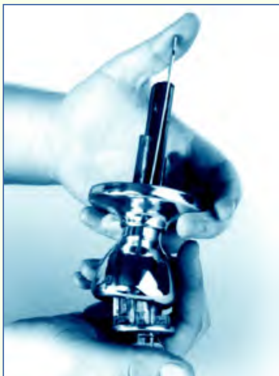
FIGURE 44 —Press the tool in as far as it will go, and push hard.
