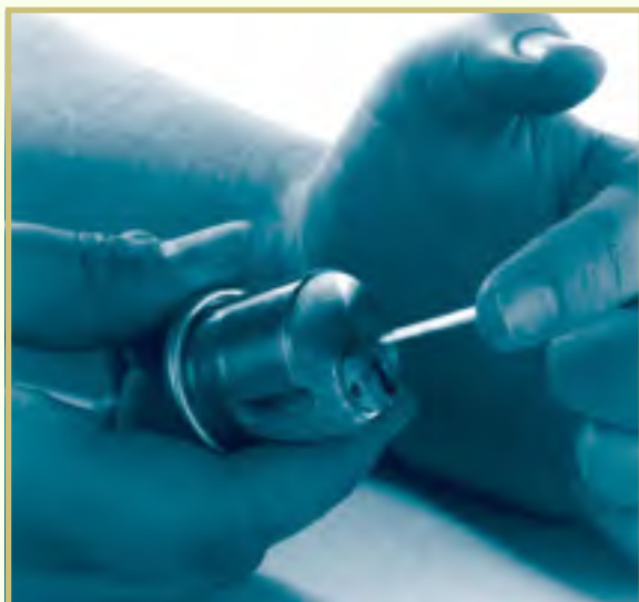
FIGURE 15 —The shim is placed in the rear of the cylinder.
