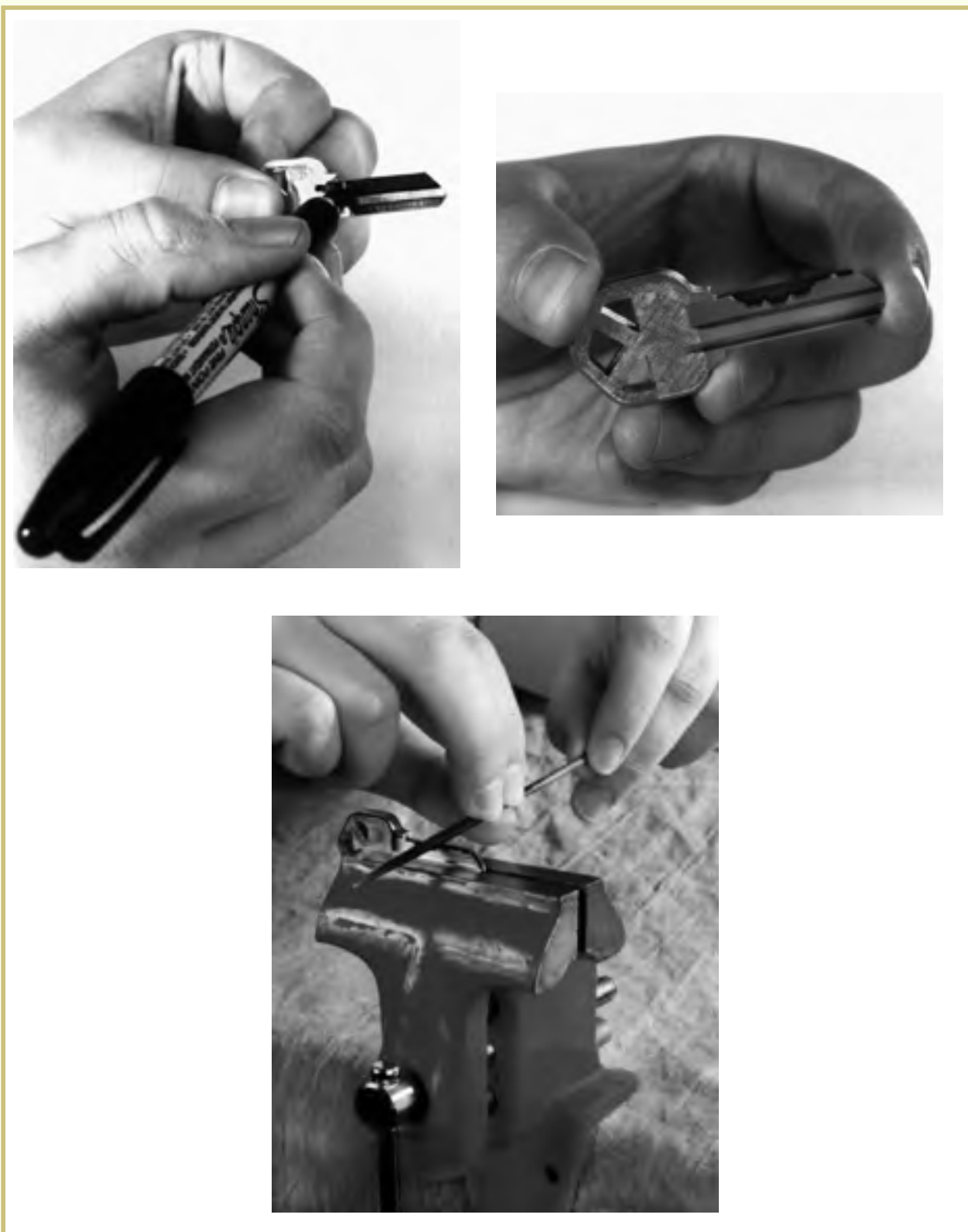
FIGURE 11—The marking-pen system for marking a key blank is illustrated here.
