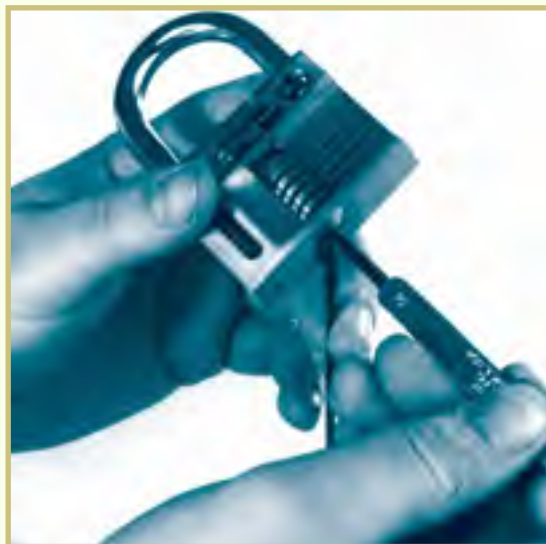
FIGURE B —To begin picking the pin tumbler lock, arrange the tools as shown here and lift the lower pins.
