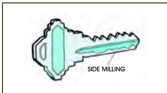
FIGURE 36—This Schlage Primus key contains two rows of bitting to operate the two mechanisms inside the lock.
