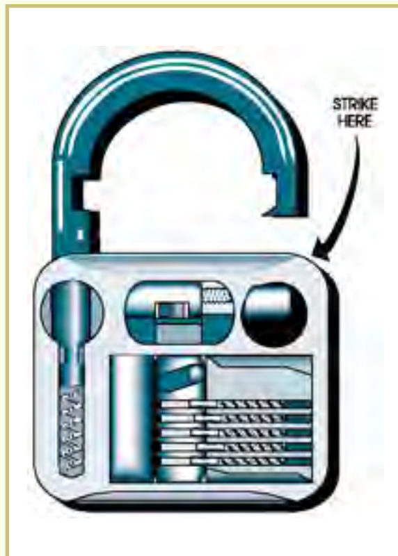
FIGURE 37 —A padlock can often be opened by hitting the padlock in the location shown here.
