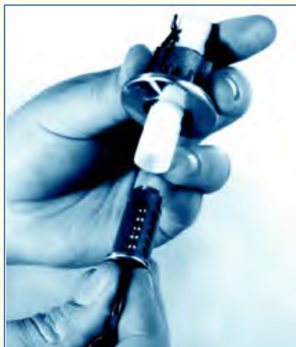
FIGURE 48 —Withdraw the plug and replace it with the plug follower at the same time.
