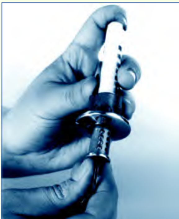
FIGURE 47 —Place the plug follower against the back of the cylinder, and make sure it's touching the back of the plug.
