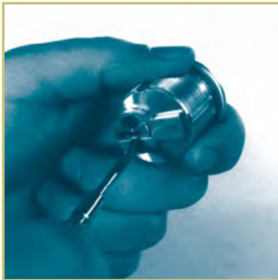
FIGURE G —Remove the retainer plate as shown here.
