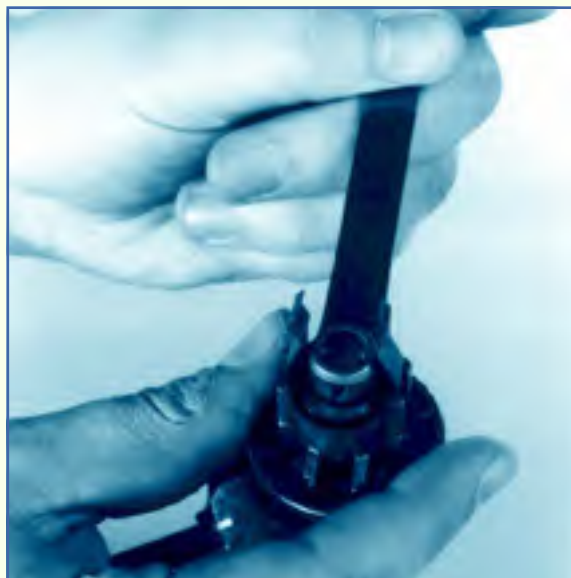
FIGURE 46 —Use the forked end of the cylinder removing tool to loosen the plug retainer clip.
