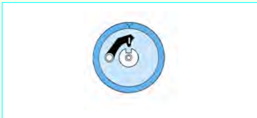
FIGURE 19 —In this lock the drop-in point is at 0 on the combination dial.
