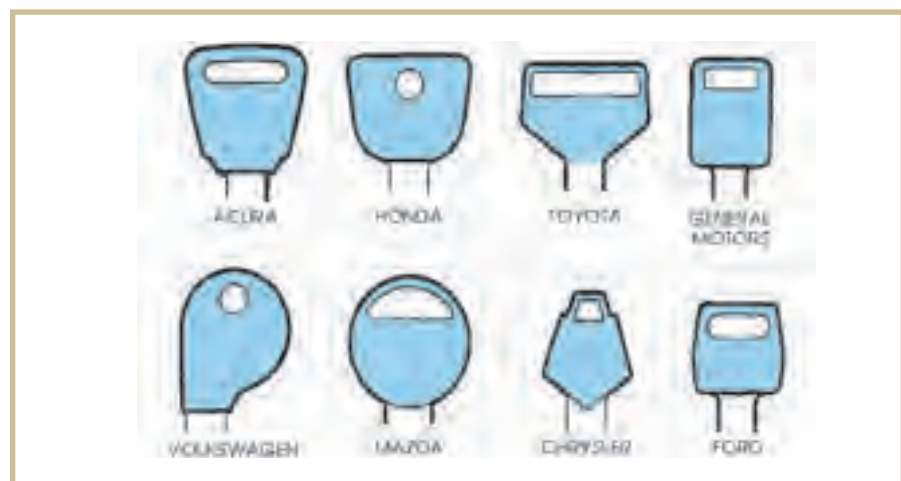
FIGURE 10 —These are some of the most common key bow shapes used by automobile manufacturers.
