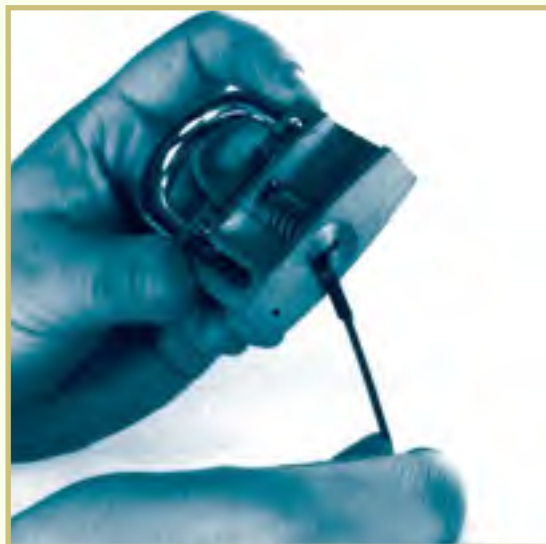
FIGURE A —Place the tension wrench into the keyway as shown here.
