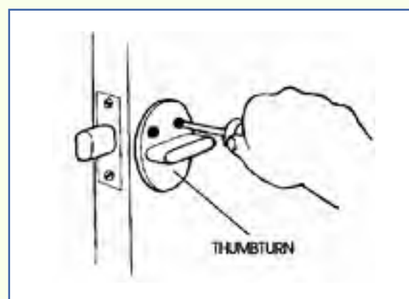
FIGURE 62 —Install the interior thumbturn.
