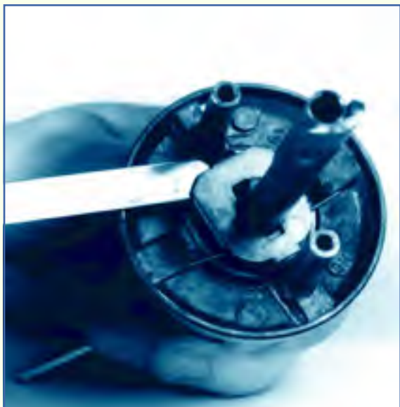
FIGURE 41 —Insert the rounded end of the tool under the clip housing as shown here, and press in on the retainer clip.
