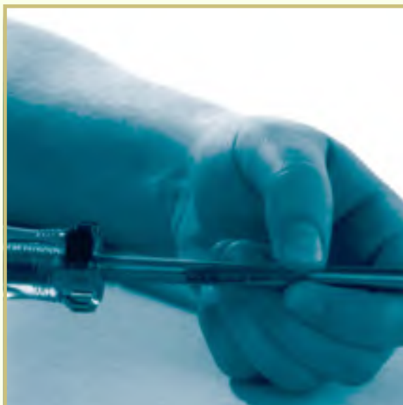
FIGURE 14 —Shim stock can be formed around a screwdriver handle.
