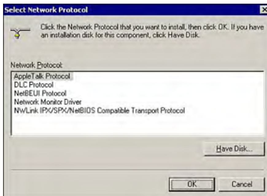
Figure 7.5. Selecting the protocol to be installed.
