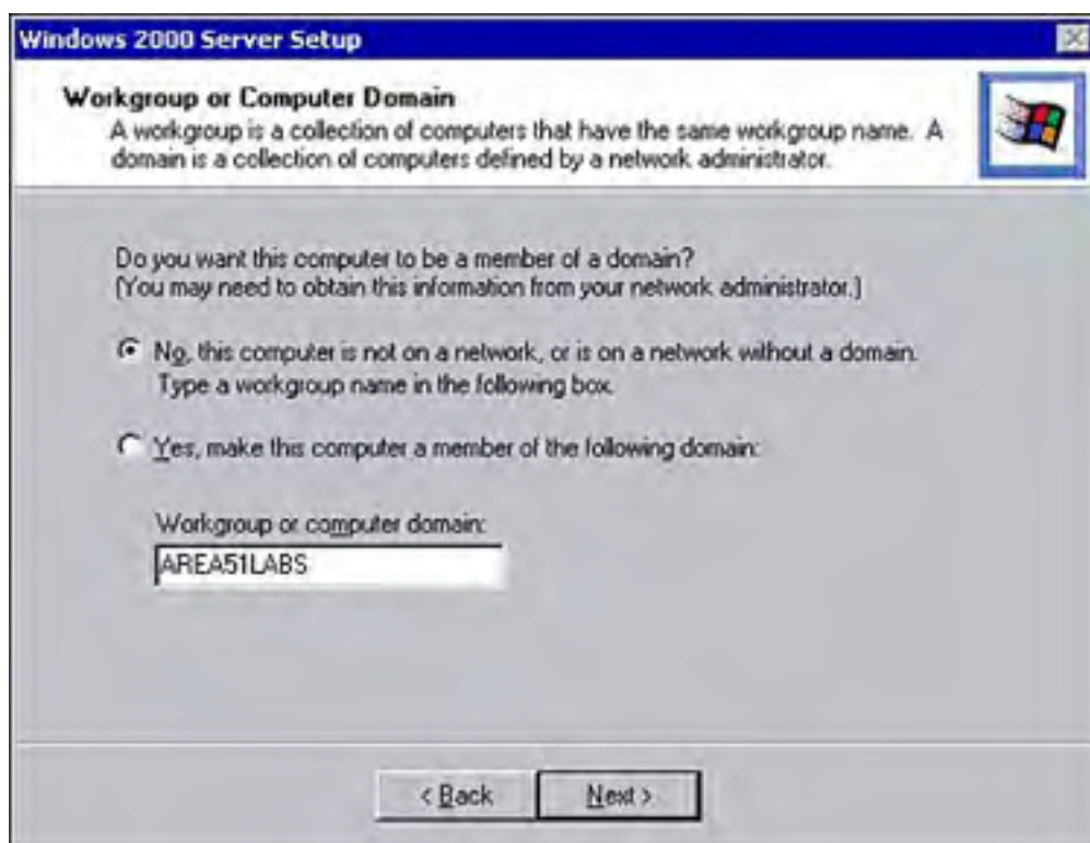
Figure 2.9. Choose the kind of network membership this server will have (Domain or Workgroup).
