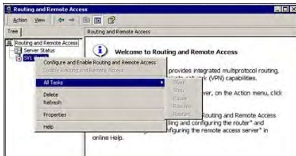
Figure 7.21. Enabling RRAS from the MMC.
