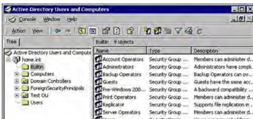
Figure 8.1. The Active Directory Users and Computers snap-in is used to create and manage users, groups, and other objects.
