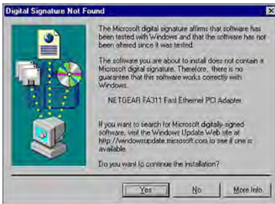
Figure 4.4. A warning dialog box appears when trying to install an unsigned driver.
