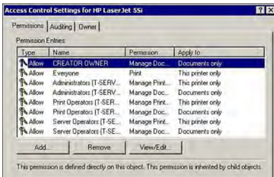
Figure 3.2. The Access Control Settings dialog box is used to manage Advanced security settings for printers in Windows 2000.
