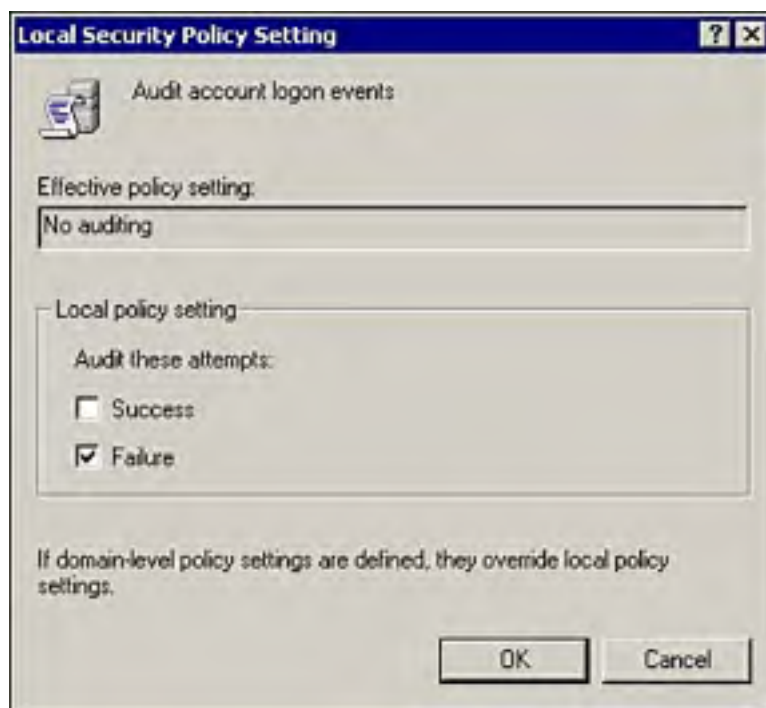
Figure 8.10. The Local Security Settings MMC, showing how to configure audit settings.
