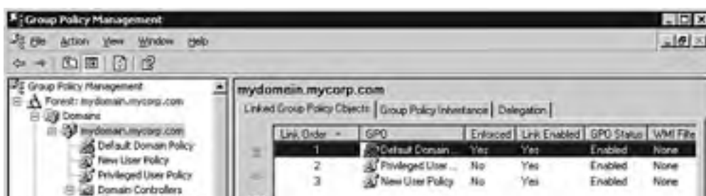
Figure 3.14. The Group Policy Management Console showing all linked GPOs and their evaluation order for the mydomain.myserver.com domain.
