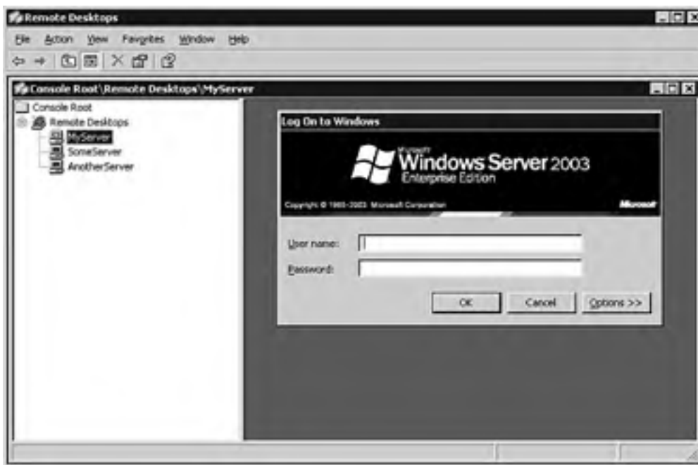
Figure 3.1. An example of the new Remote Desktops MMC snap-in that provides multi-console functionality similar to the earlier Terminal Services client of Windows 2000.
