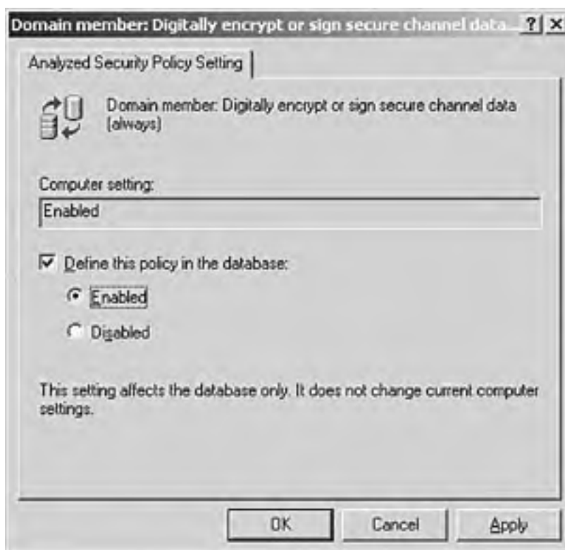
Figure 7.4. The Analyzed Security Policy Setting tab showing the Digitally Encrypt or Sign Secure Data Channel enabled on the local system computer.
