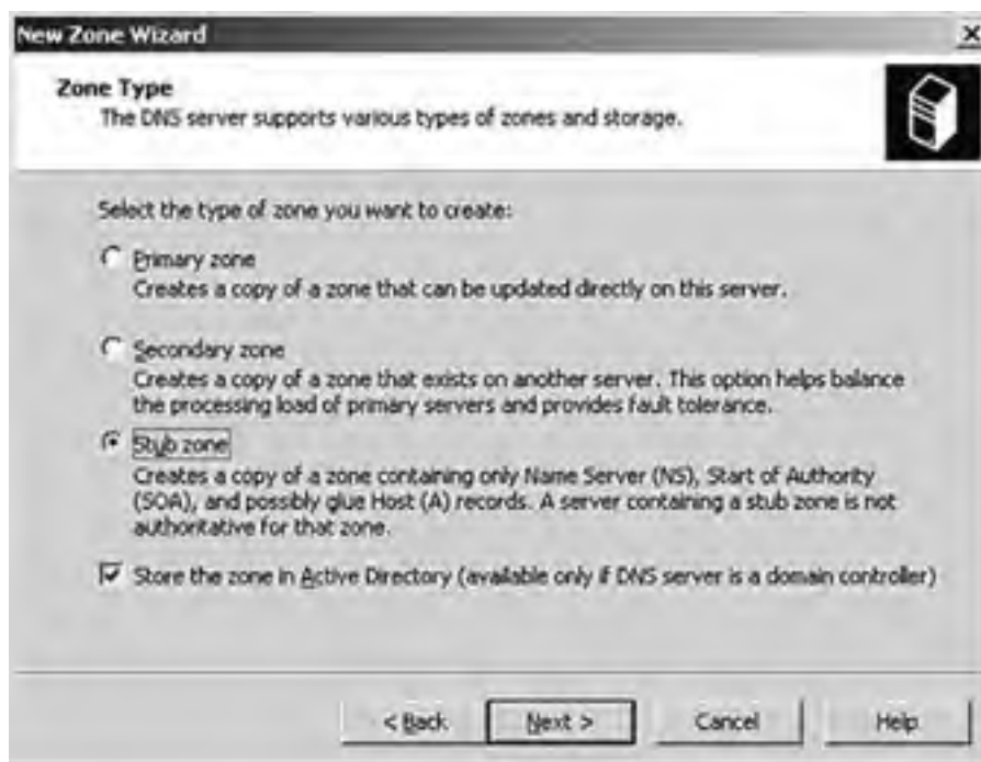
Figure 6.8. Zone Type dialog box showing Stub Zone selected.
