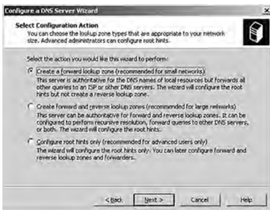
Figure 6.4. Select Configuration Action dialog box showing Create a Forward Lookup Zone selected.
