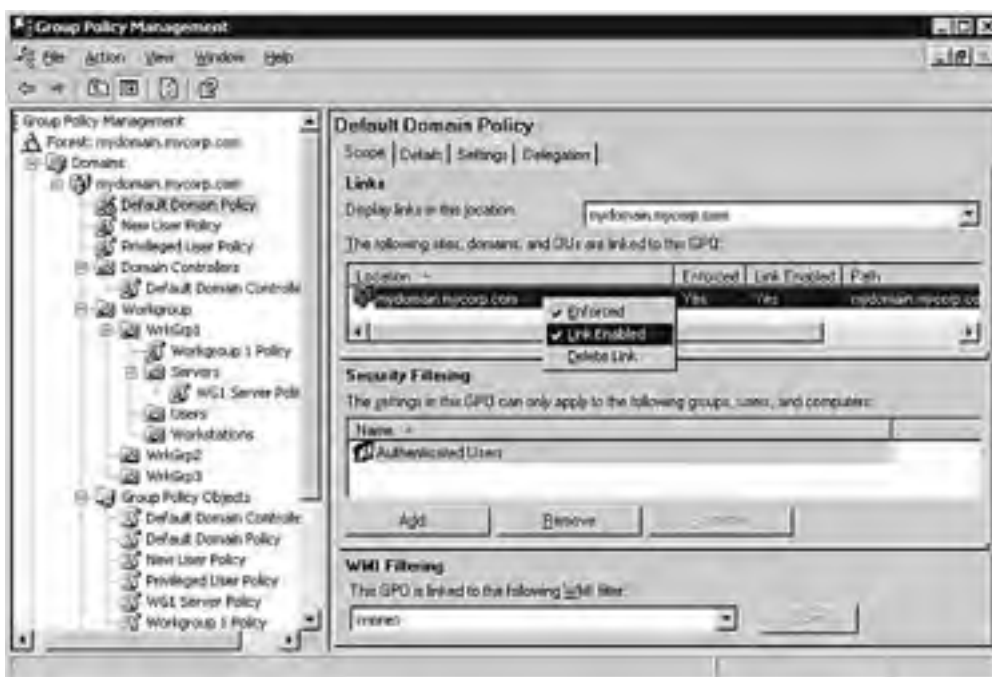
Figure 3.9. The Group Policy Management Console showing a current manipulation of the enforcement status of the Default Domain Policy link to the mydomain.mycorp.com domain.
