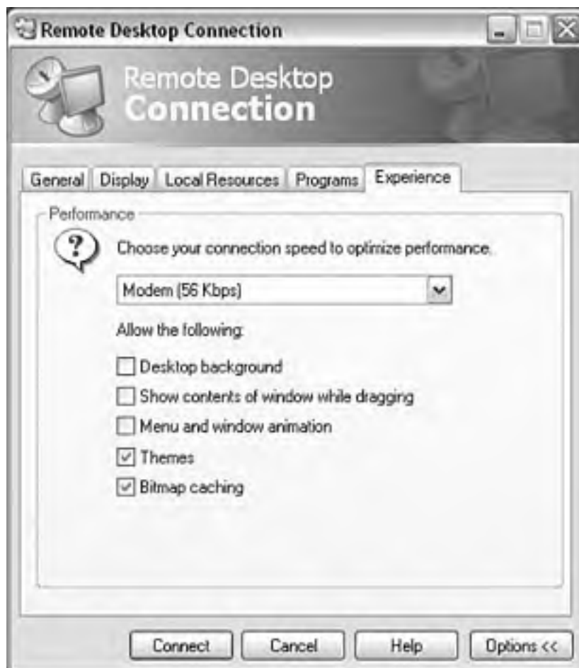
Figure 4.8. You can configure the proper connection settings for the remote connection via the Experience tab of the Remote Desktop Connection dialog box.
