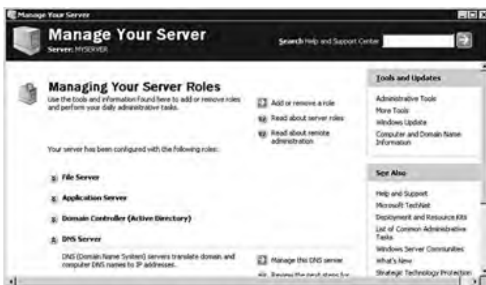
Figure 2.4. The Manage Your Server Wizard showing configured server roles for file server, application server, domain controller, and DNS server functionality.
