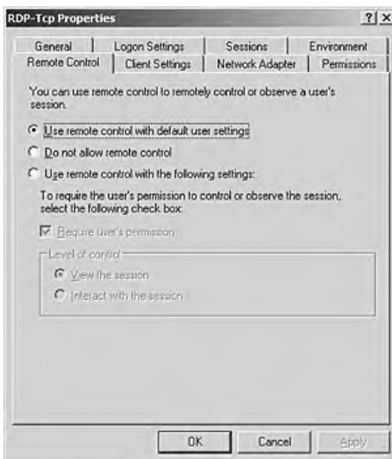
Figure 4.7. You can configure client remote session settings via the RDP-TCP Properties dialog box.
