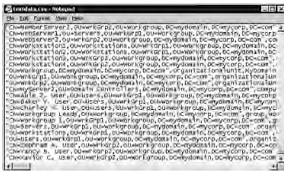
Figure 2.6. Sample .csv file (testdata.csv) that includes Active Directory object data generated by use of the csvde utility.
