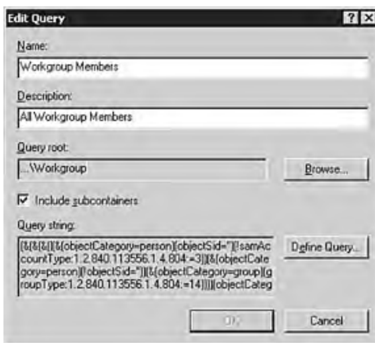
Figure 2.13. A saved query specifying criteria for accounts in the Workgroup OU container and all subcontainers.
