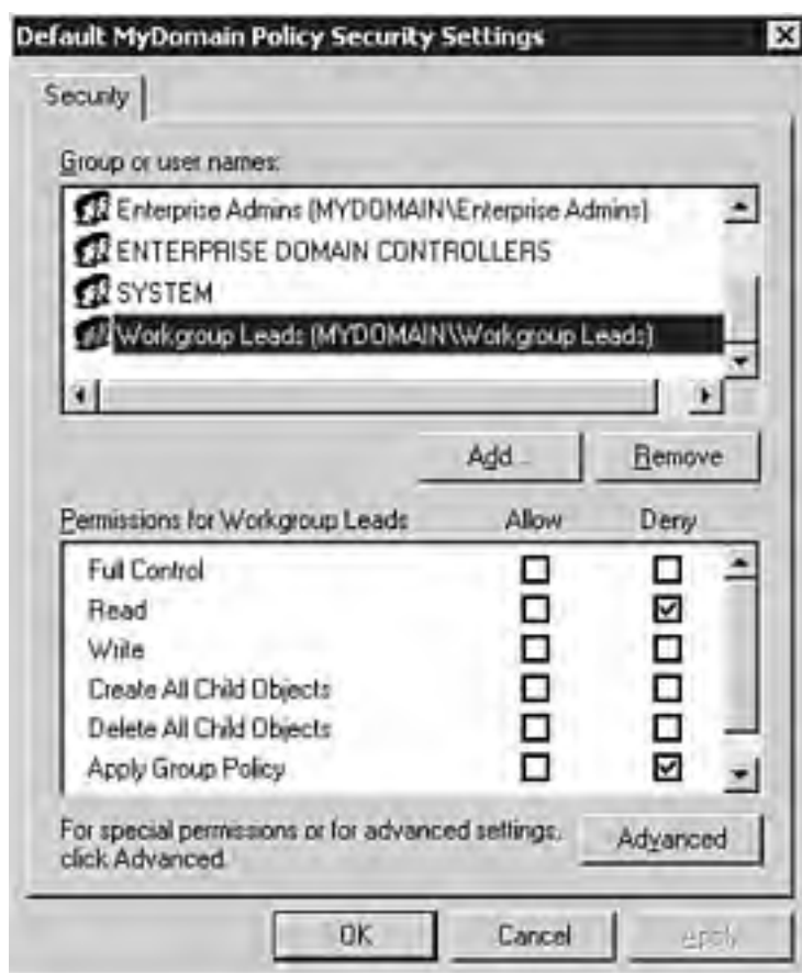
Figure 3.13. Restricting the Read and Apply Group Policy rights of the Workgroup Leads group with regard to the Default MyDomain Policy.
