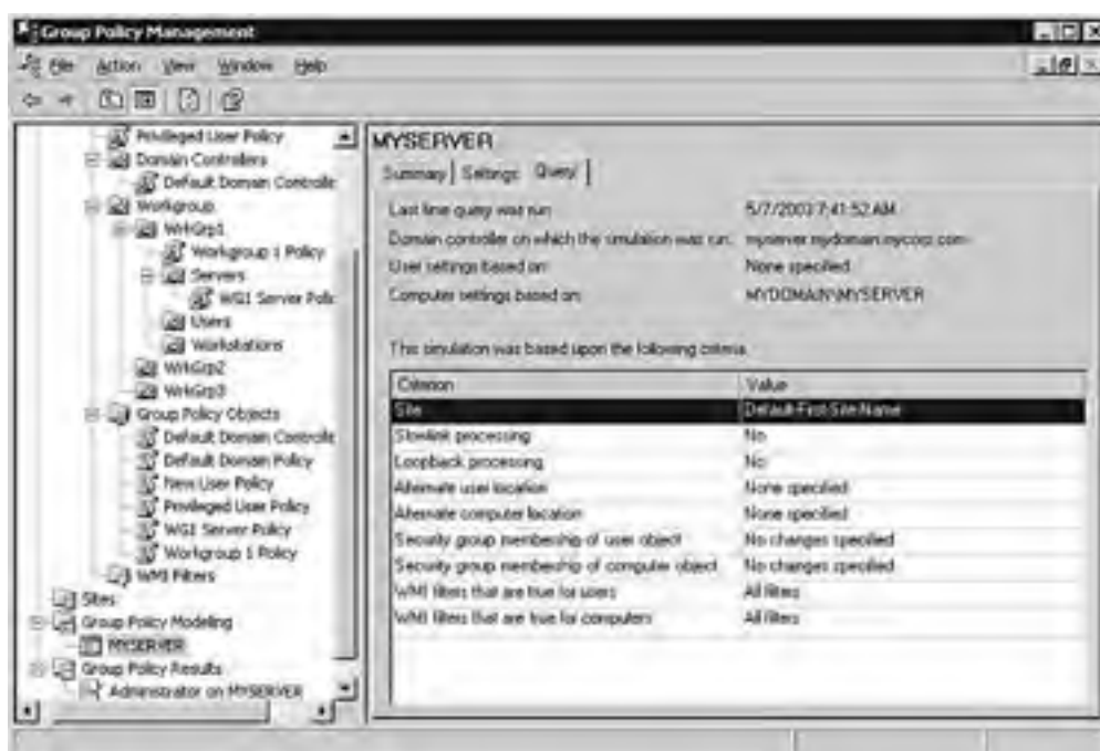
Figure 3.18. The Group Policy Management Console showing the query settings for an evaluation of GPO application.
