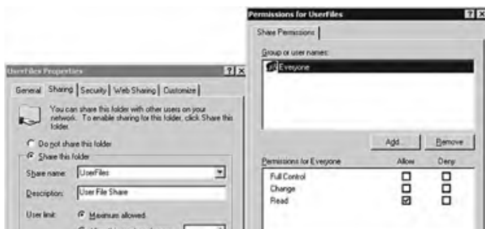
Figure 3.3. The Sharing and Share Permissions dialog boxes for a newly created share named UserFiles.
