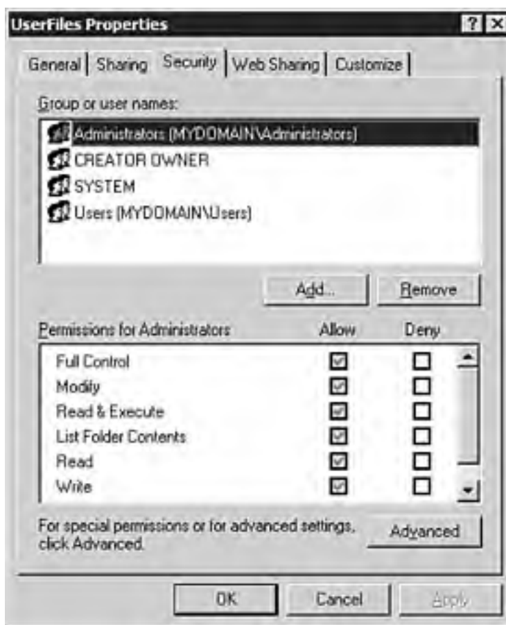
Figure 3.4. The Security tab for a newly created share whose target is the UserFiles folder.
