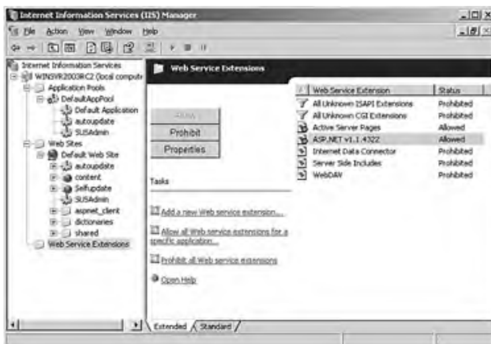
Figure 4.9. You can verify the status of ASP.NET Web Server Extensions via IIS Manager.
