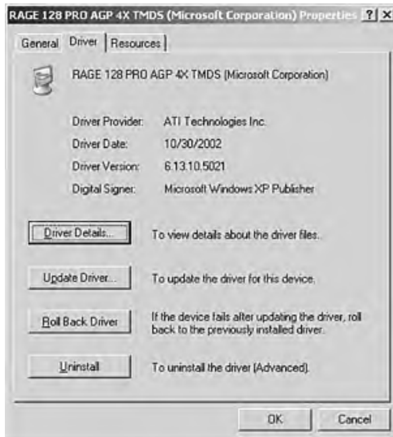
Figure 5.6. Click the Roll Back Driver button to use a previous driver.
