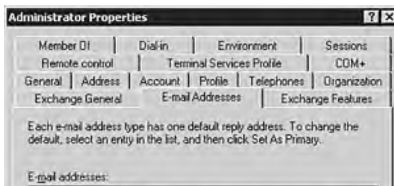
Figure 2.2. The Properties dialog box for the Administrator account opened within the Active Directory Users and Computers MMC snap-in to show the addition of mail-related items caused by the installation of Microsoft's Exchange Server.
