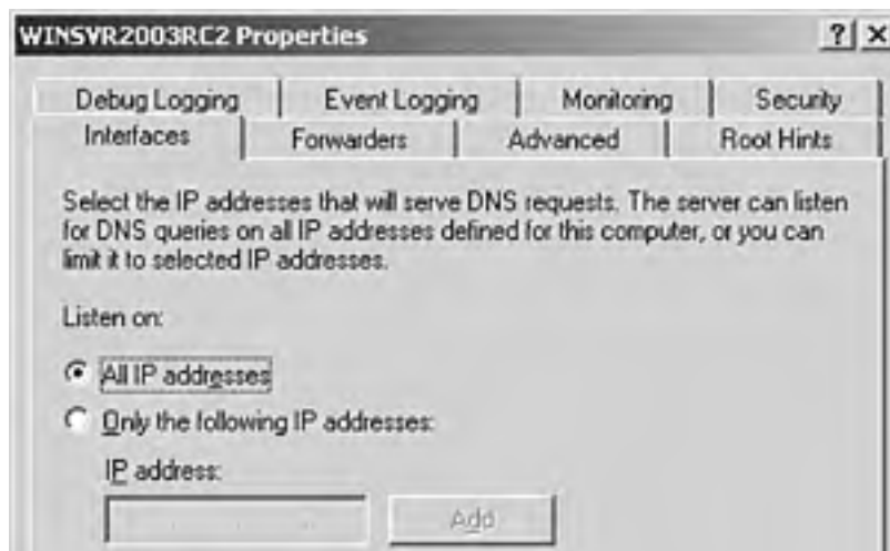
Figure 6.10. DNS Server Properties dialog box showing the Interfaces tab.
