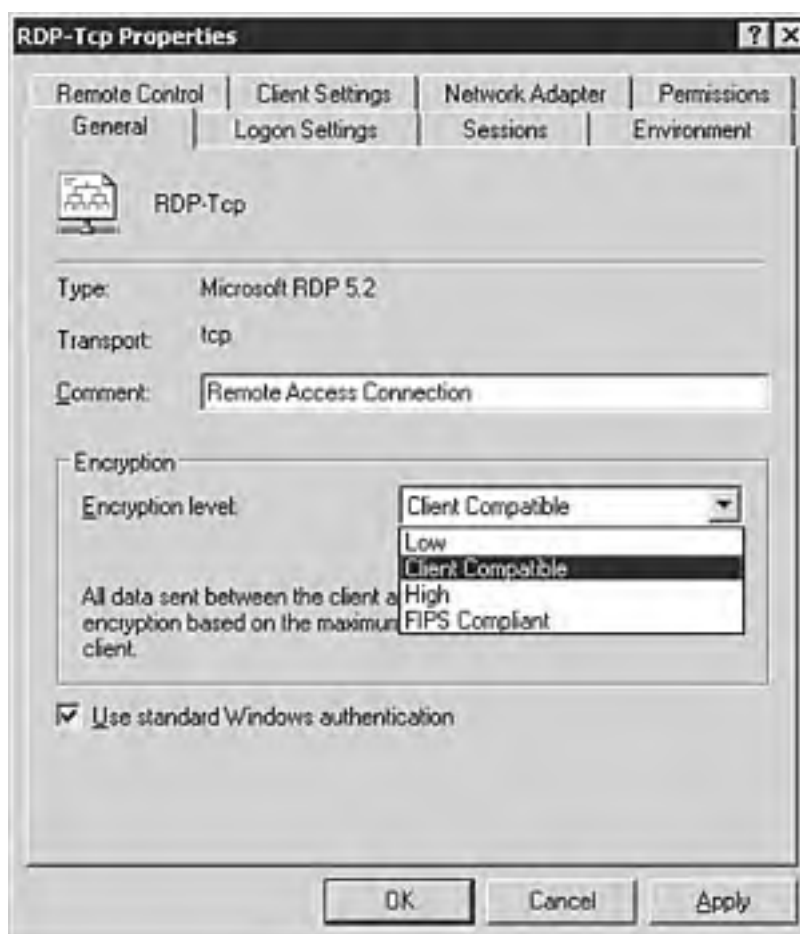
Figure 3.28. Terminal Server configuration within the Terminal Server Configuration MMC snap-in.
