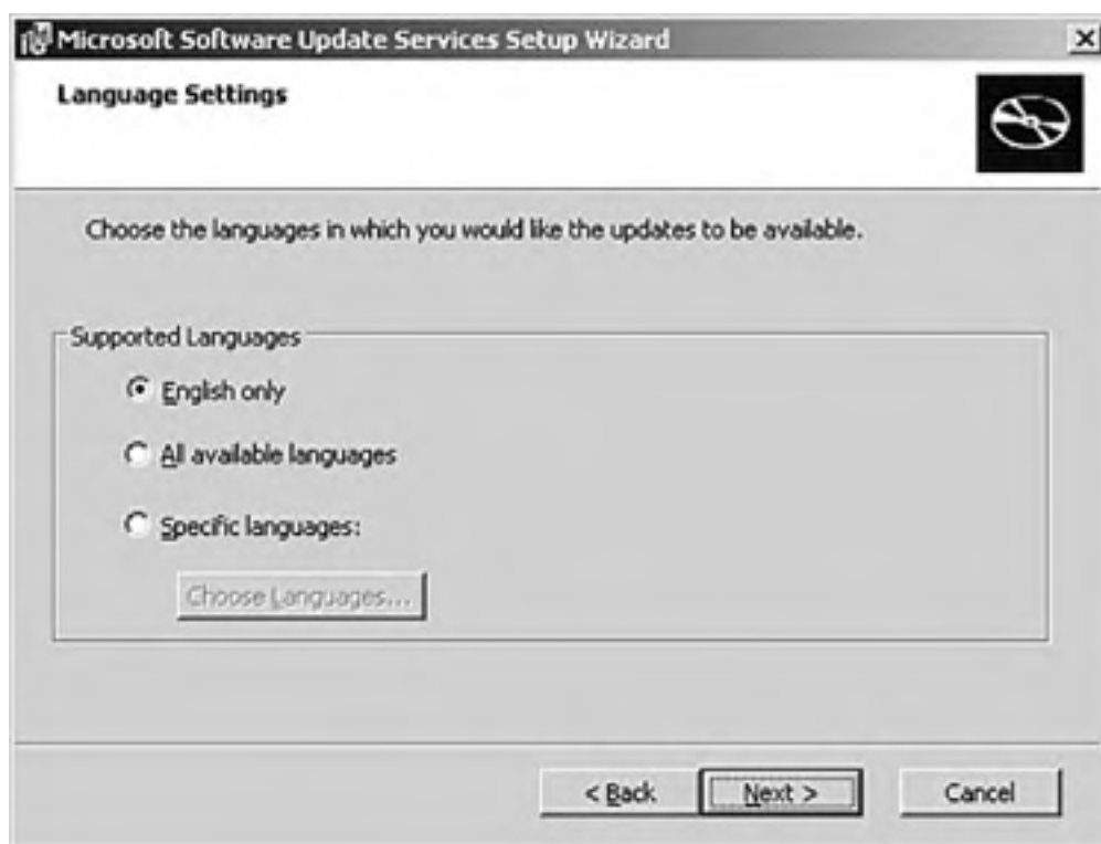
Figure 4.1. You can conserve disk space by specifying a language on the Language Settings screen.
