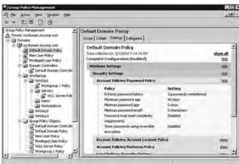
Figure 3.11. The Group Policy Management Console showing a report of the current Default MyDomain Policy GPO settings.
