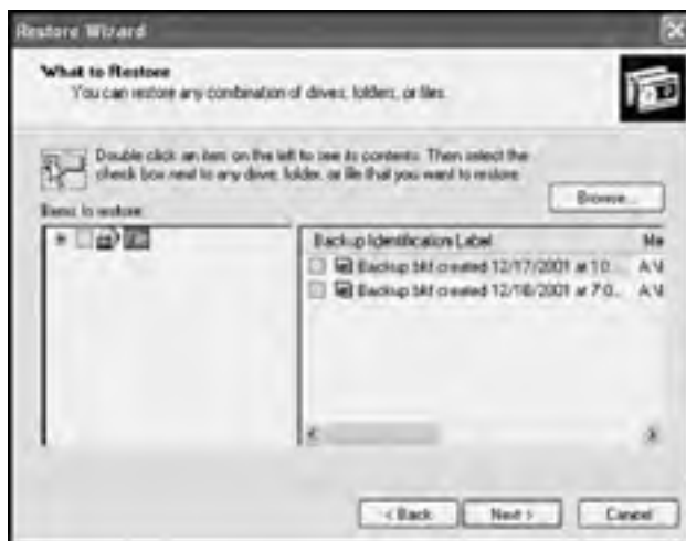
Figure B.12: Specifying the location of the backup containing the files and folders to be restored
