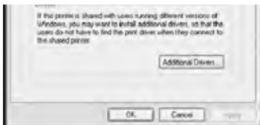
Figure 5.26: The Sharing property sheet determines whether or not the printer is shared with other computers on a local area network
