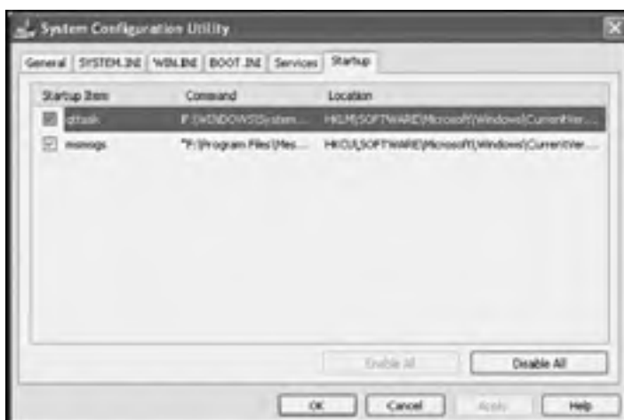
Figure 12.18: Controlling which Windows XP applications are started during system startup
