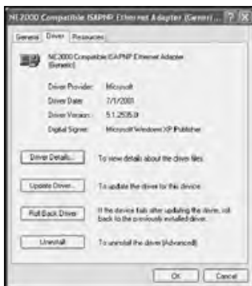
Figure 1.10: Windows XP automatically saves a copy of a device's software driver before performing a driver update
