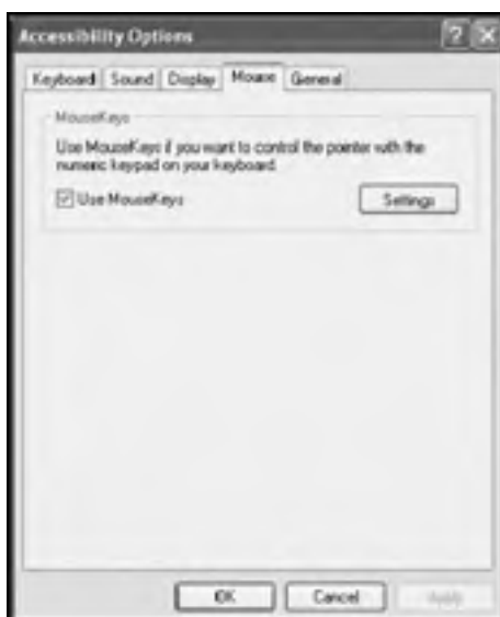
Figure 8.19: The Mouse property sheet on the Accessibility Options dialog provides access to settings that allow the keyboard to be substituted for the mouse
