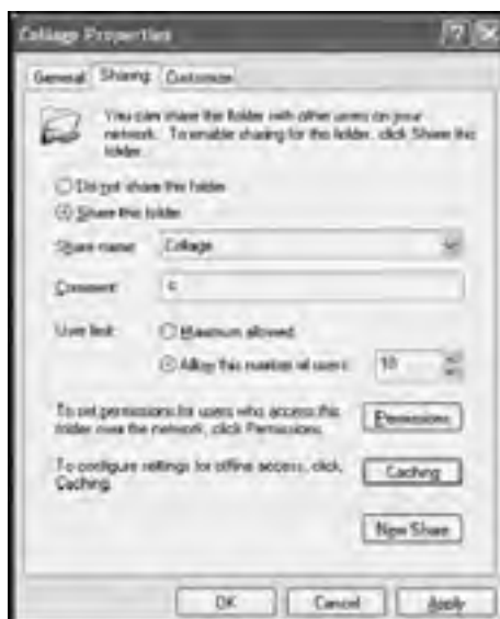
Figure 19.13: Setting up a shared disk drive when simple file sharing is disabled
