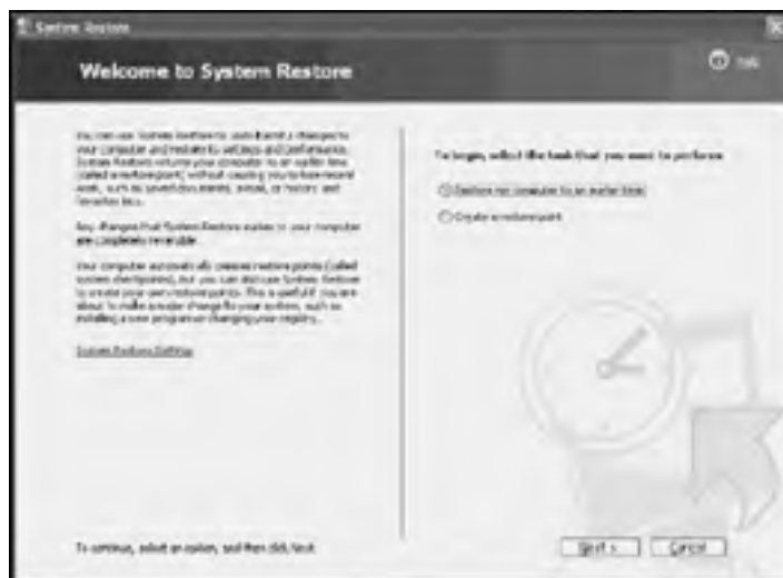
Figure 1.11: The Windows XP System Restore utility lets you recover from harmful changes made to system settings
