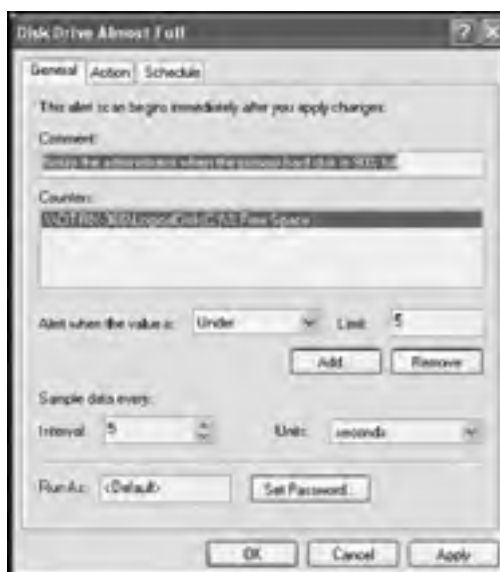
Figure 13.21: Creating an alert that reports on when a hard drive begins to fill up
