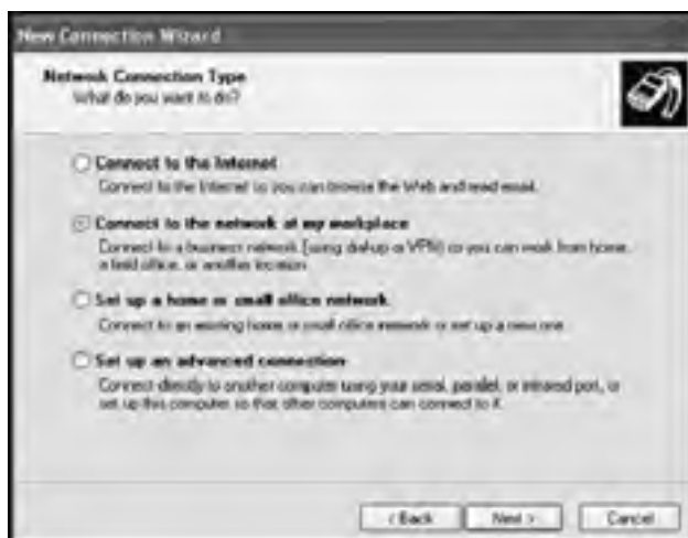
Figure 15.6: Setting up a dial-up connection to connect to a corporate dial-up server
