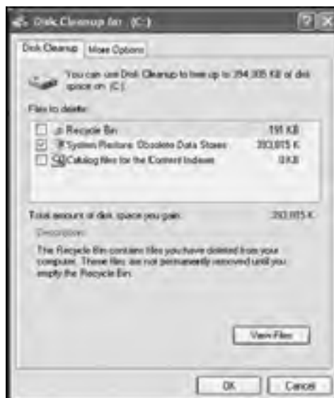
Figure 13.8: Use the Disk Cleanup utility to free up disk space by removing unnecessary files from the computer
