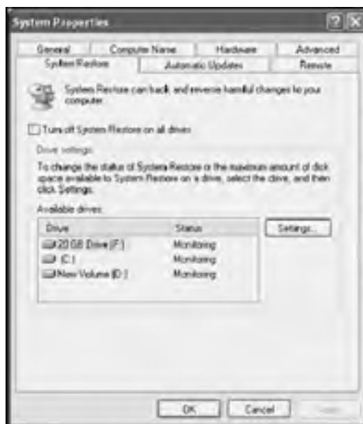
Figure 3.21: Configuring which drives are tracked and restored by the System Restore process
