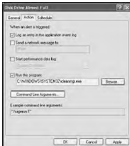
Figure 13.22: Specify what actions are performed when a counter's threshold specified in an alert is exceeded
