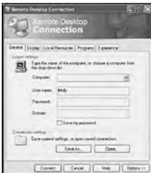
Figure 15.21: Using the General property sheet, the user can specify a different username and password and save Remote Desktop settings
