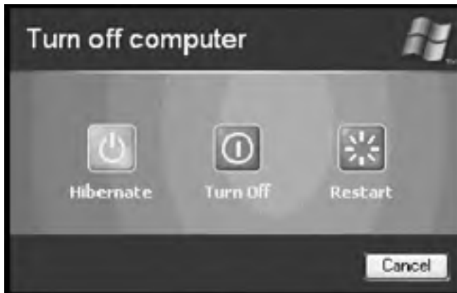
Figure 1.26: Shutting down a Windows XP Professional system that uses the Windows Welcome Screen
