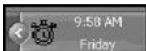
Figure 8.14: The Show FilterKey status on screen option displays a graphical stopwatch, indicating that FilterKey settings are being used
