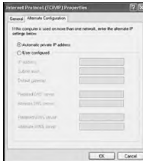
Figure 16.9: Configuring Windows XP to use an automatic private IP address as its alternate configuration
