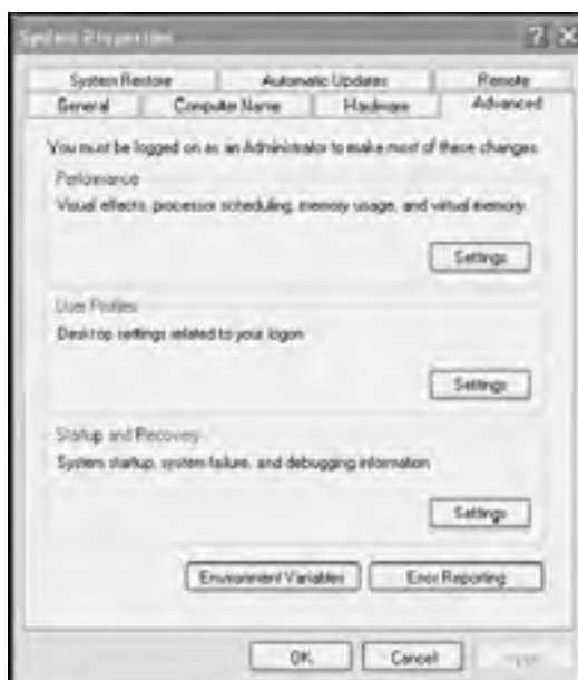
Figure 3.25: The option for configuring error reporting is found on the Advanced property sheet of the System Properties dialog
