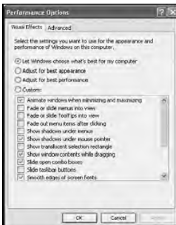
Figure 13.2: Windows XP's performance settings control visual affects as well as processor, memory, and virtual memory settings
