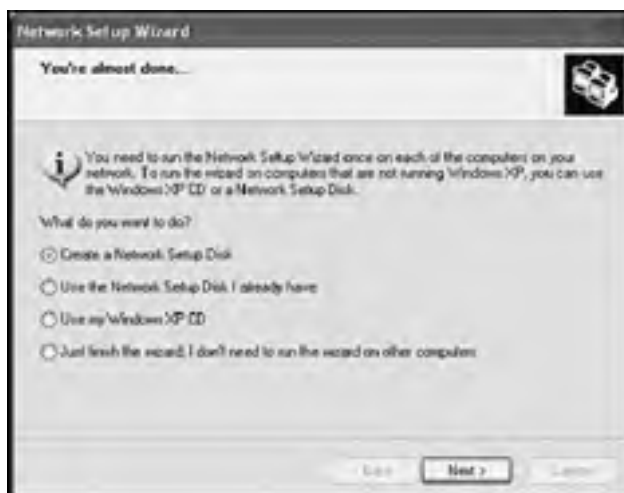
Figure 18.10: The Network Setup Wizard can be used to create a setup disk for configuring non Windows XP computers on a workgroup network
