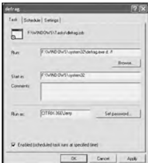
Figure 4.21: Refining the execution of a scheduled task by adding command line arguments
