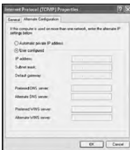
Figure 15.26: Configuring alternate TCP/IP settings that are to be used when mobile users connect to a network that uses statically assigned TCP/IP settings
