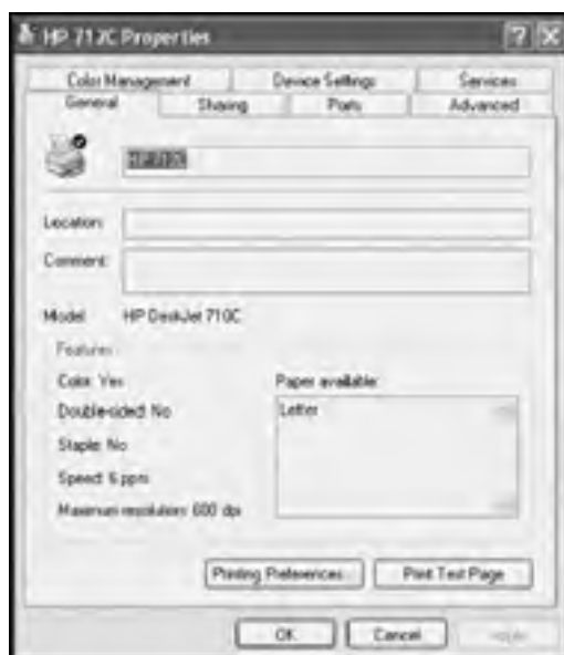
Figure 5.25: The General property sheet displays information about basic printer features and provides the ability to change the print device's name, location, and comment information
