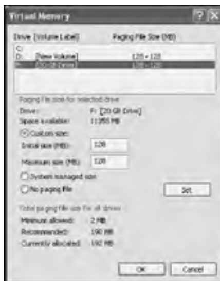
Figure 13.5: Spreading virtual memory out over two disk drives to improve system performance
