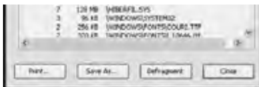
Figure 11.17: The Disk Defragmenter snap-in can provide a detailed text report of its analysis of the hard disk drive
