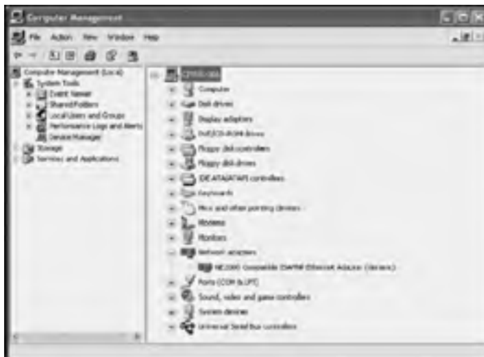
Figure 10.17: The Device Manager extension allows administrators to view and configure all the hardware devices installed on a computer
