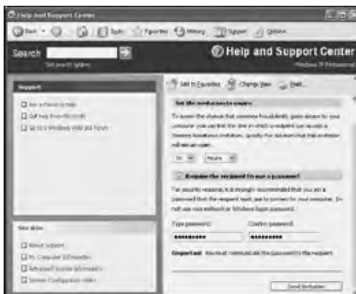
Figure 3.14: To provide additional security, instruct users to limit invitation expiration periods and to assign a password to every invitation
