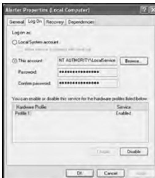
Figure 10.23: Associating a user account with a service to ensure that it has the security permissions that it requires to execute
