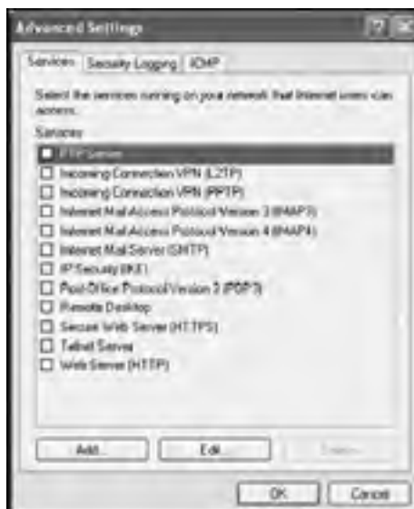
Figure 17.16: Enabling specific services so that their associated ports and protocols are permitted to pass through ICF
