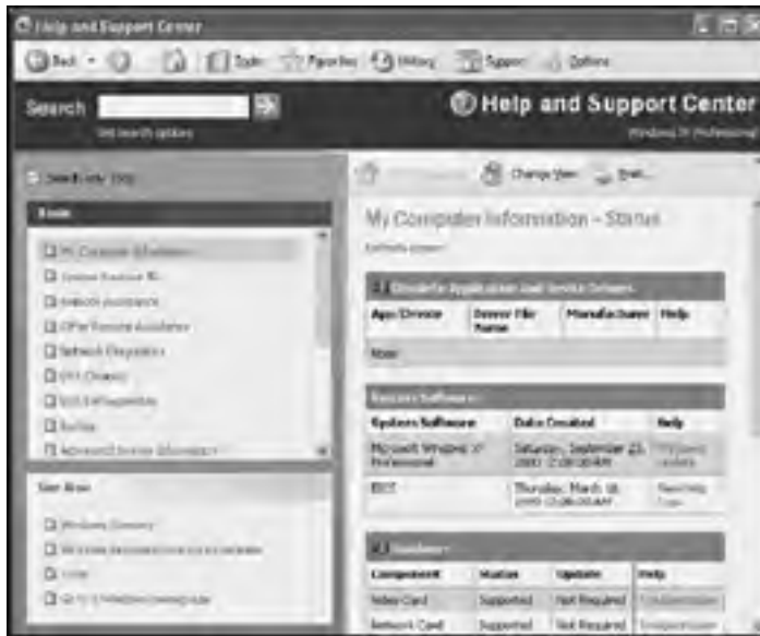
Figure 3.22: Viewing detailed information about the hardware and software installed on a computer running Windows XP Professional
