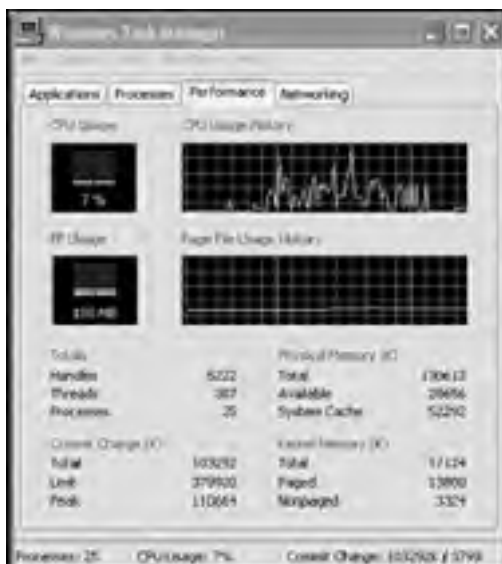
Figure 13.14: Using the Task Manager to monitor system performance and view detailed memory statistics
