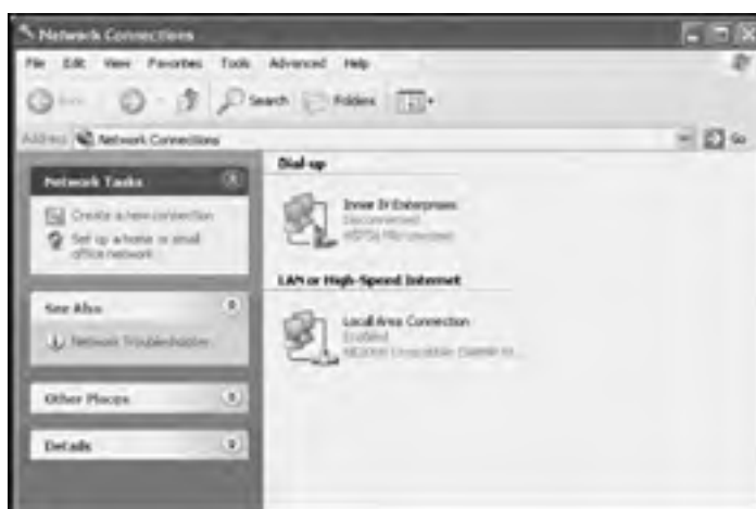
Figure 15.8: Windows XP Professional stores icons representing dial-up connections in the Network Connections folder
