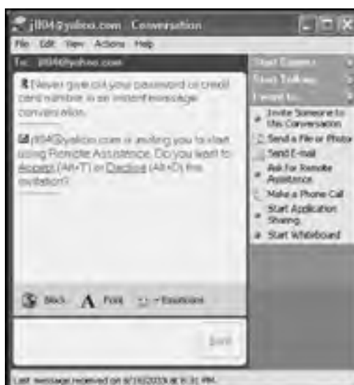
Figure 3.12: The helper receives the Remote Assistance invitation and clicks on Accept to initiate a Remote Assistance session
