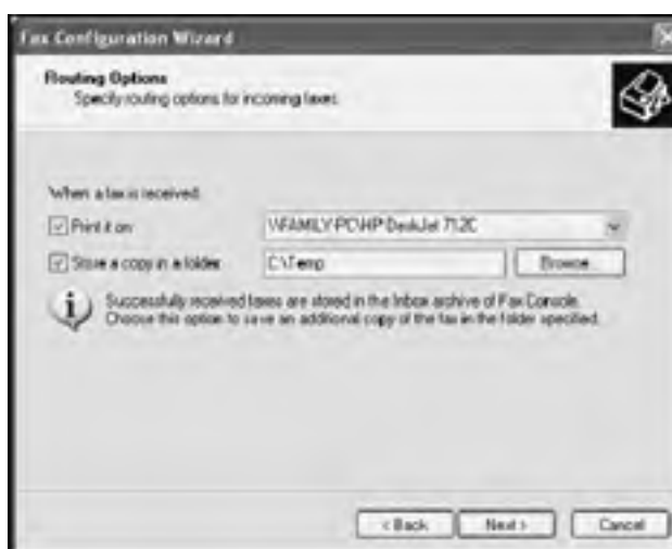
Figure 5.6: Tell the Fax Configuration Wizard what to do when an incoming fax is received
