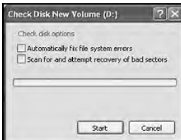
Figure 11.13: The chkdsk utility can perform a scan of the file system and check the disk for bad sectors
