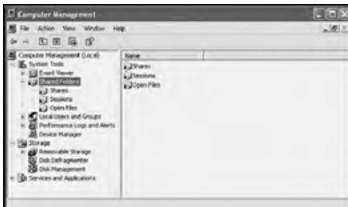
Figure 19.18: The Shared Folders extension or snap-in provides the ability to monitor local and remote connections to shared drives and folders
