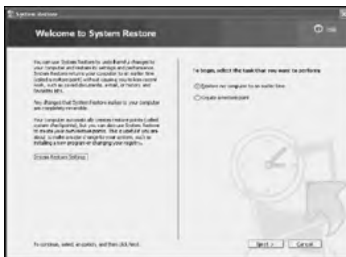
Figure 3.20: System Restore provides a means of restoring critical system files to a previous state
