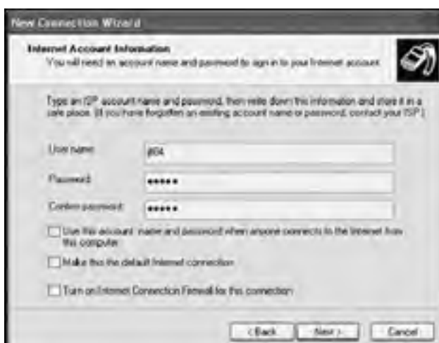
Figure 17.10: Supply the user name and password assigned by the ISP for the Internet account
