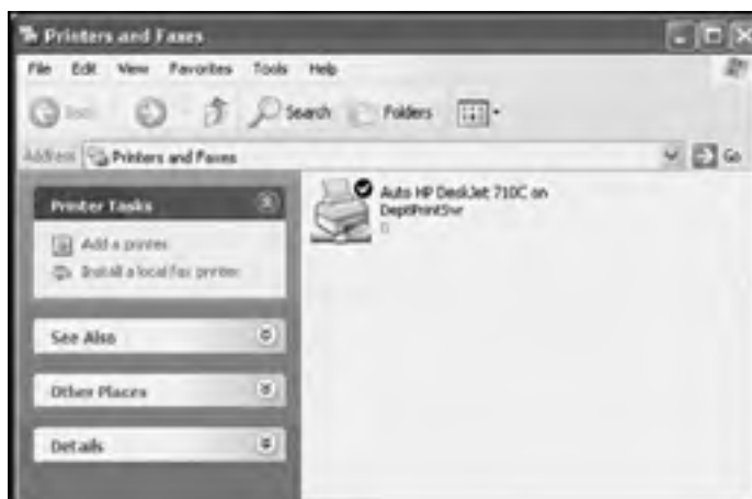
Figure 19.1: Windows XP professional can automatically detect shared printers on the local subnet
