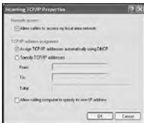
Figure 15.11: Configuring local area network access and TCP/IP settings for an incoming dial-up connection
