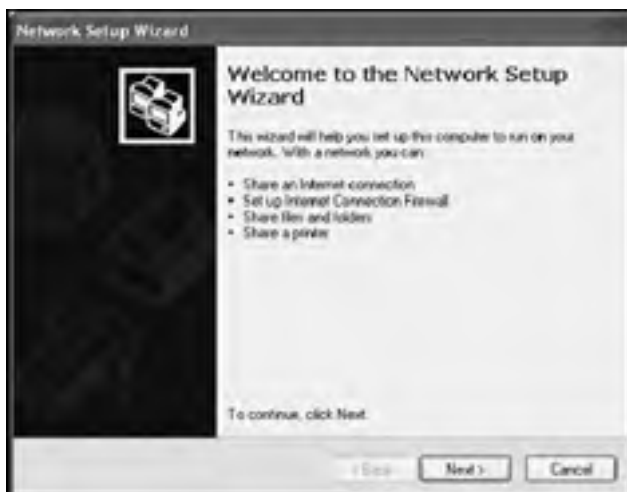
Figure 1.19: The Network Setup Wizard facilitates the setup of small networks and in the configuration of file and printer sharing
