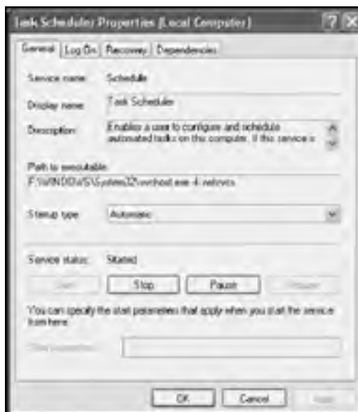
Figure 4.12: The General property sheet on the Task Scheduler Properties dialog can be used to change task startup type and to control task execution
