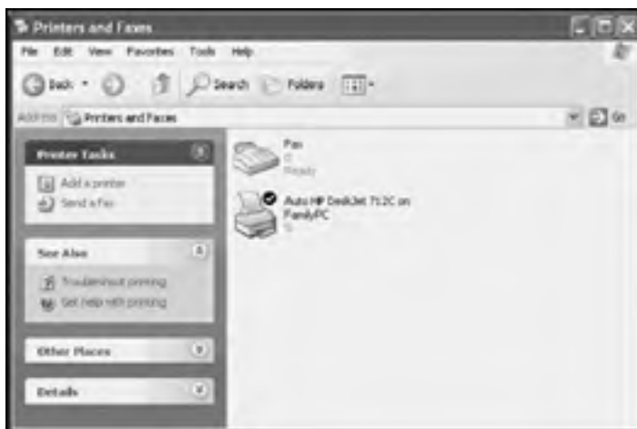
Figure 5.32: On small networks and local subnets, Windows XP Professional automatically detects and sets up a connection with most network print devices
