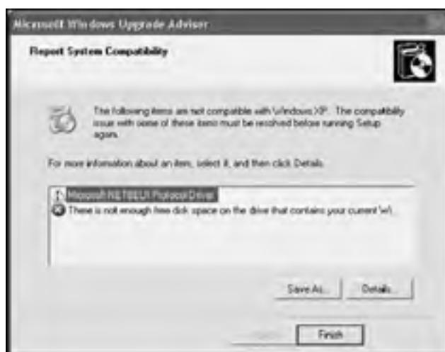
Figure 2.3: The Upgrade Advisor generates a report of all incompatible hardware and software found on the computer
