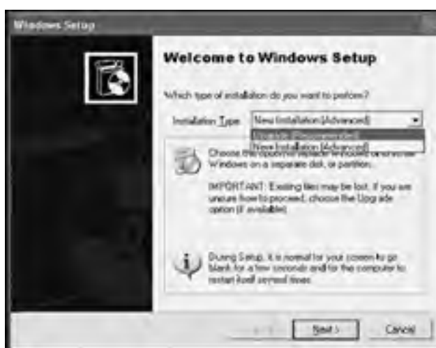
Figure 2.5: The Windows XP Professional install program lets you perform an upgrade or a new installation
