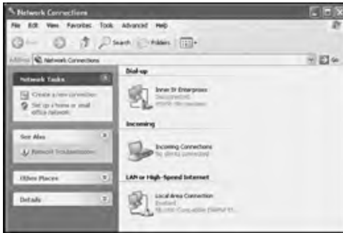
Figure 15.12: The Incoming Connections icon represents the dial-up server connection and can be used to see if anyone is currently using the connection
