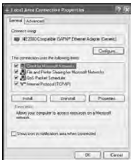
Figure 18.3: Examining installed local area network software components
