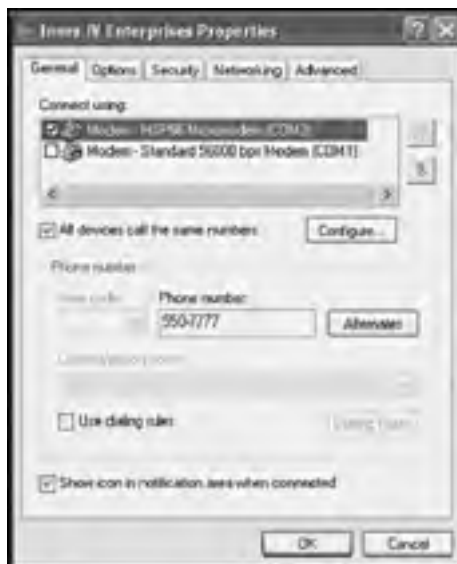
Figure 15.10: Configuring a dial-up connection to use multiple modems to establish a multilink connection
