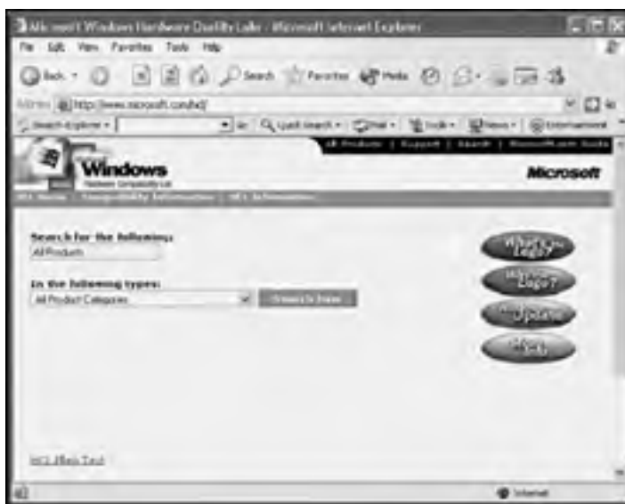
Figure 2.1: Use the HCL to verify the compatibility of hardware installed on a computer before attempting to install Windows XP Professional
