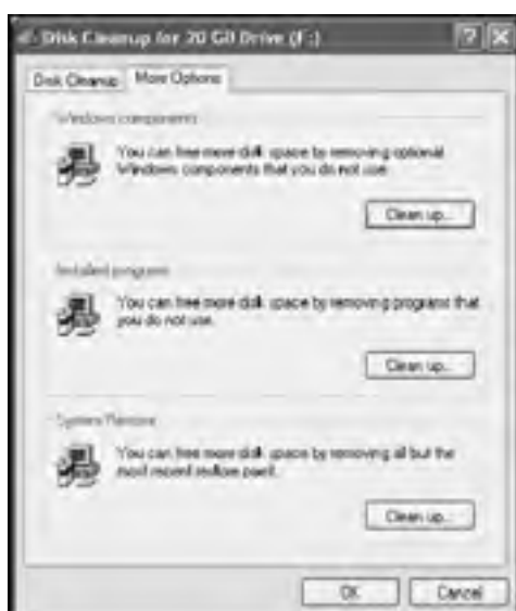
Figure 11.22: Disk Cleanup can be used to access the components of the Add/Remove Programs utility that allows administrators to uninstall Windows components or applications
