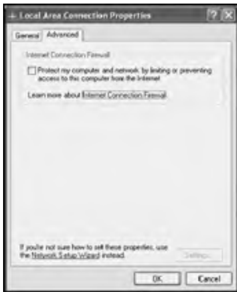
Figure 1.15: ICF protects a computer that is directly connected to the Internet from external intrusion and attack
