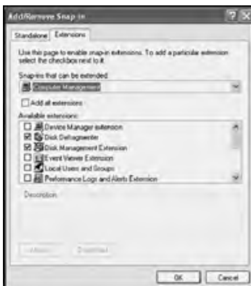
Figure 10.7: Select the extensions that are to appear in a custom console containing the Computer Management snap-in
