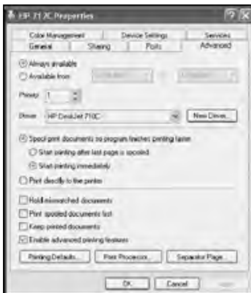
Figure 5.29: The Advanced property sheets allows administrators to configure print device availability and priority settings
