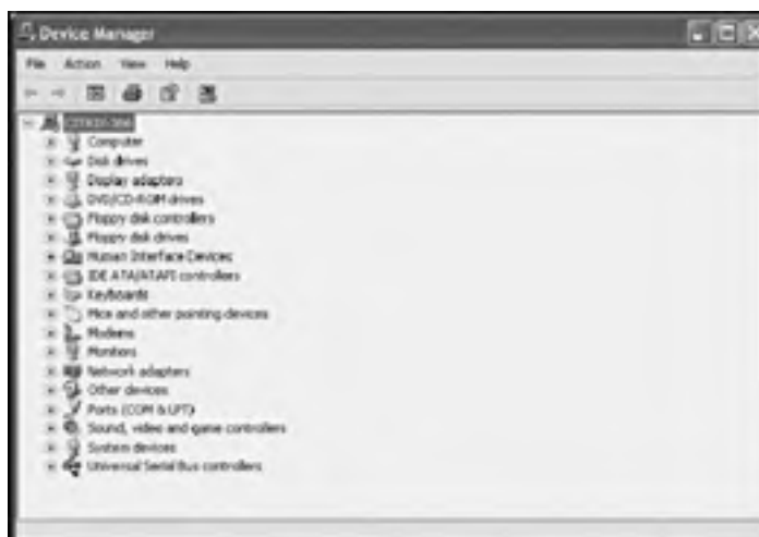
Figure 2.14: Device Manager provides a graphical view of all the hardware installed on a computer
