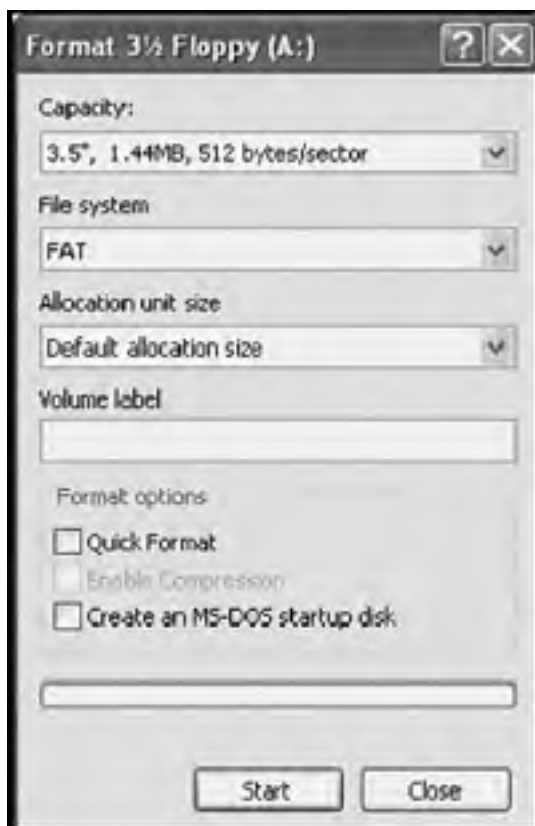
Figure B.8: Creating a Windows XP startup disk for systems that use FAT or FAT32
