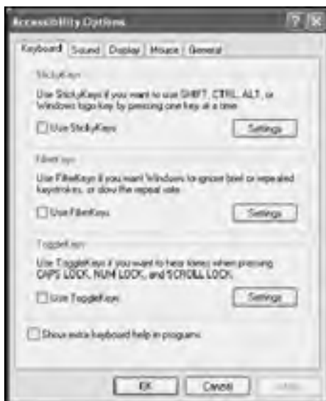
Figure 8.10: The Keyboard property sheet on the Accessibility Options dialog provides access to an assortment of keyboard configuration settings
