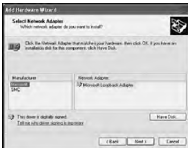
Figure 18.2: Selecting the manufacturer of the network adapter and the type of card being installed
