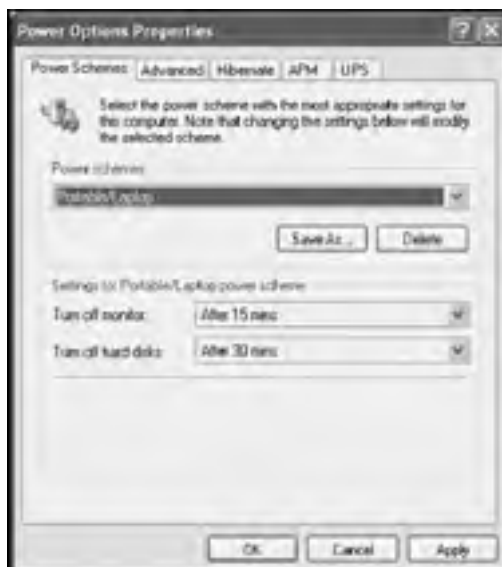
Figure 13.11: Power schemes provide control over the way that Windows XP Professional manages power consumption
