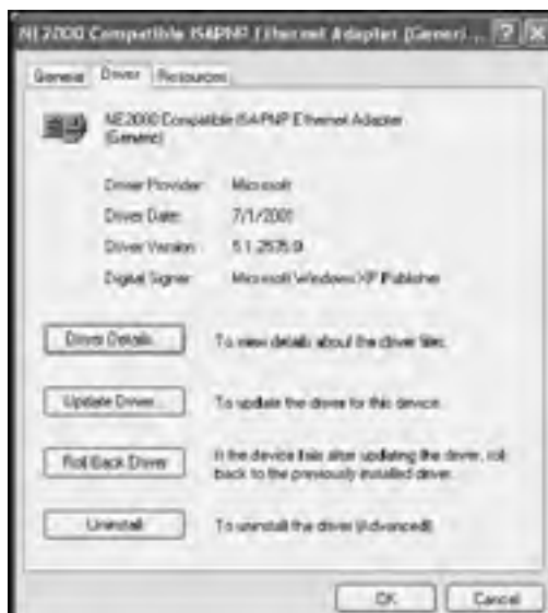
Figure 2.18: The Driver property sheet provides detailed control over a device's software driver
