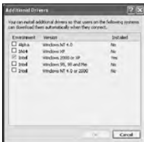
Figure 5.27: By loading drivers for other operating systems, administrators make the setup of network printer connections easier
