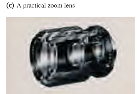
34.43 A simple zoom lens uses a converging lens and a diverging lens in tandem. (a) When the two lenses are close together, the combination behaves like a single lens of long focal length. (b) If the two lenses are moved farther apart, the combination behaves like a short-focal-length lens. (c) A typical zoom lens for a single-lens reflex camera, containing twelve elements arranged in four groups.
