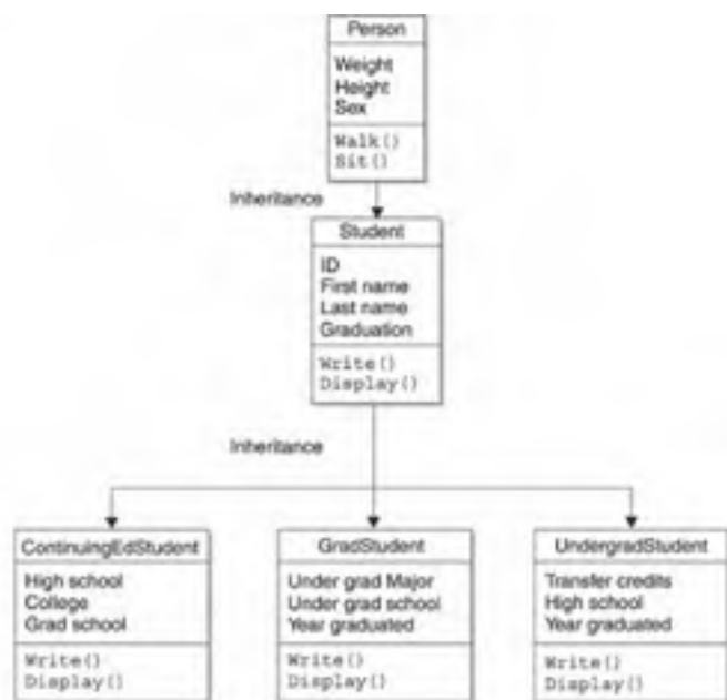
Figure 5-4: Use level inheritance when there is a relationship between two or more parent classes. Here a relationship between Student and Person exists because a student is a person.
