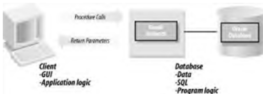
Figure 8-2. Two-tier system with stored procedures
