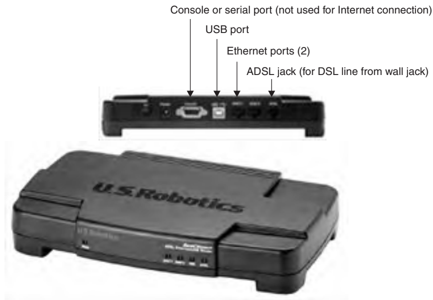
Figure 11-3 External DSL modem: Ethernet, USB, and serial ports
