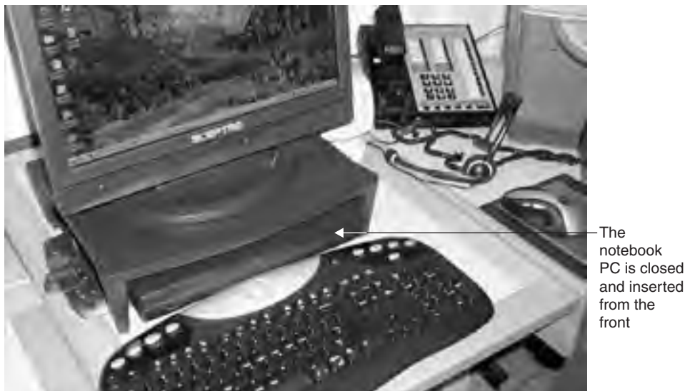
Figure 7-2 Notebook PC docked in a port replicator
