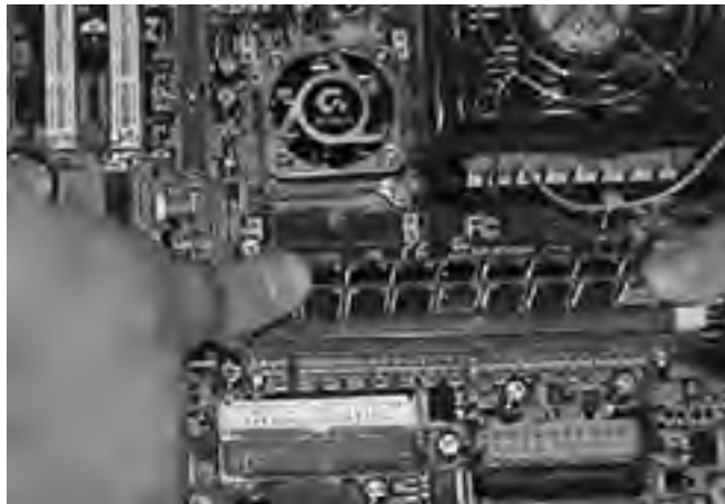
Figure 10-4 Inserting a 512MB RAM module in a DIMM slot
