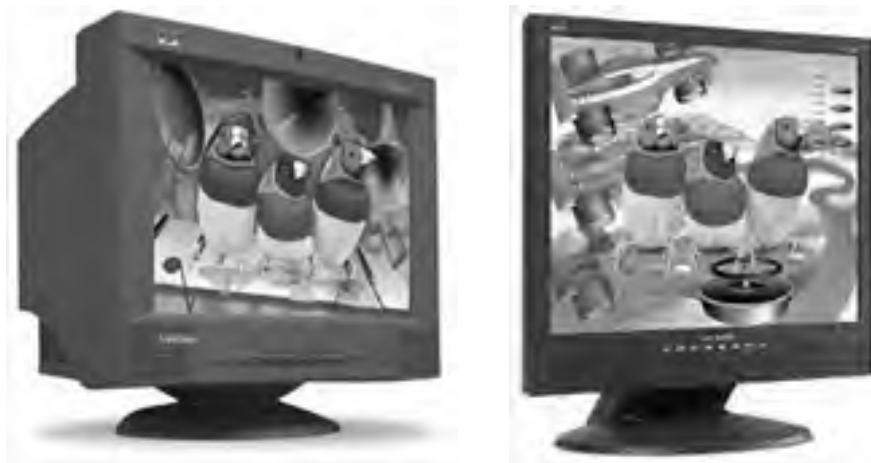
Figure 4-1 A CRT monitor (left) and an LCD flat panel monitor (right)
