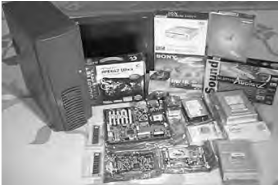
Figure 8-3 The components for a home-built PC
