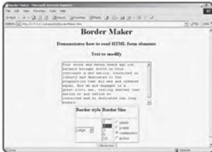
Figure 2.13: The borderMaker HTML page uses a text area, two list boxes, and a select group.
