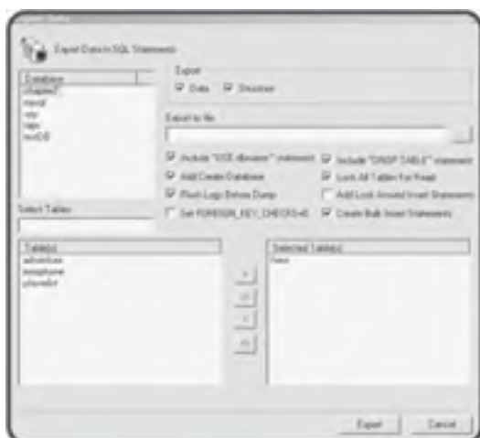
Figure 7.18: From this dialog box you can generate code that will manufacture replicas of any database created or viewed with SQLyog.
