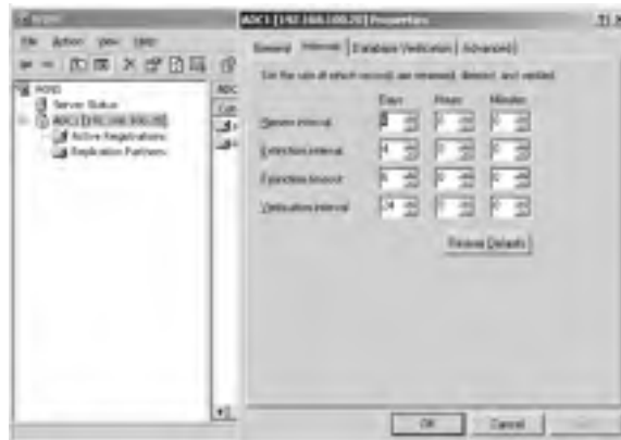
Figure 6.35 Interval Settings for Registration Renewal, Removal, and Verification
