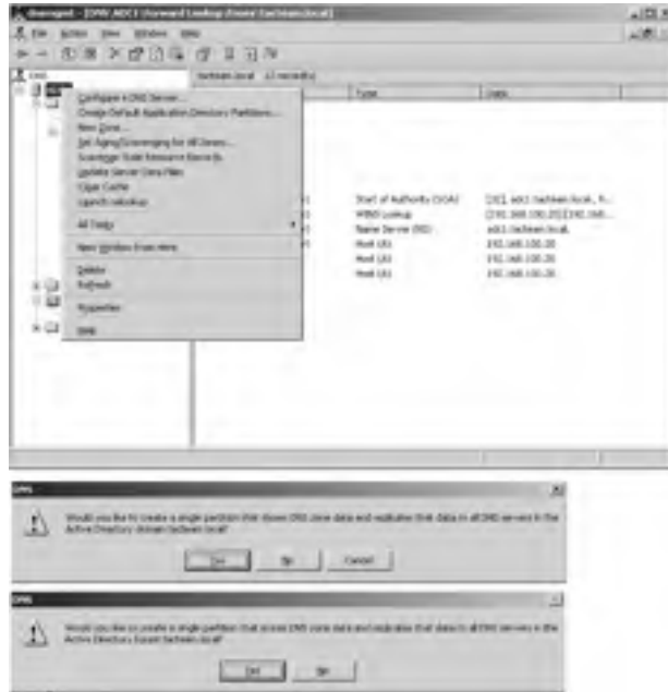
Figure 6.9 Creating the application directory partition using the DNS console
