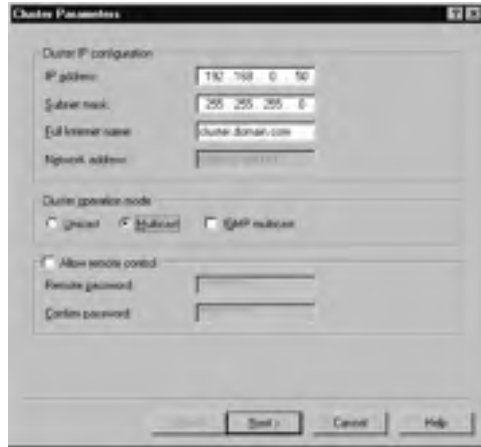
Figure 9.52 Select Multicast Cluster Operation Mode
