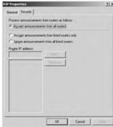
Figure 4.37 The Security Tab of the RIP Properties
