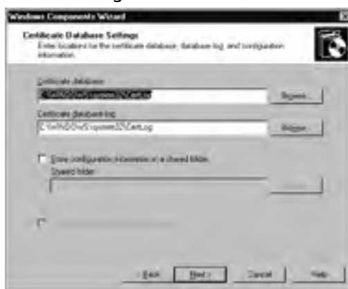
Figure 12.6 Selecting the Certificate Database Location
