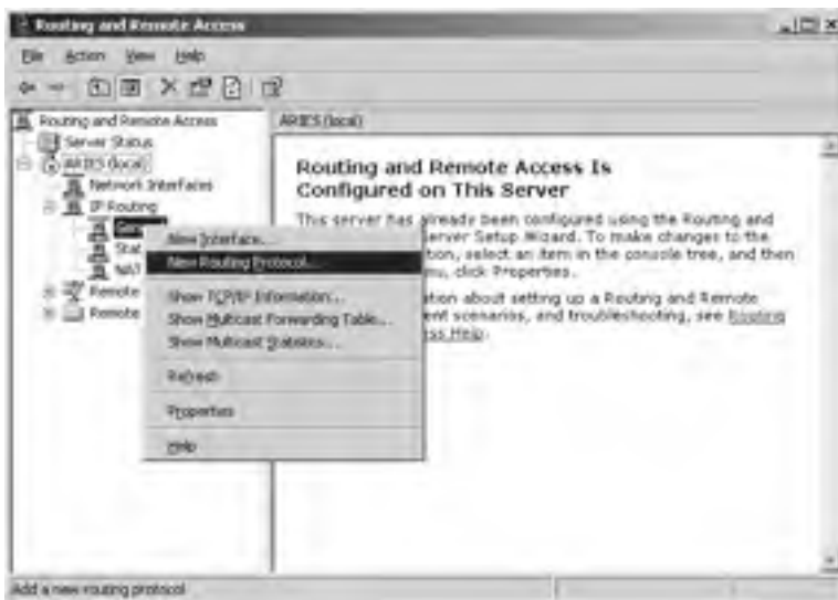
Figure 4.38 Add a New Routing Protocol
