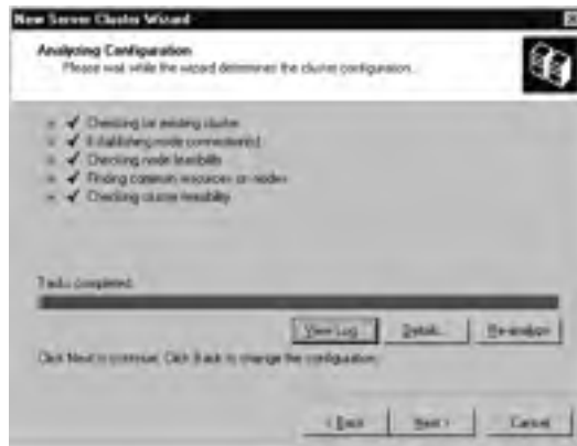
Figure 9.33 Finished Analyzing the Configuration of the Cluster Node
