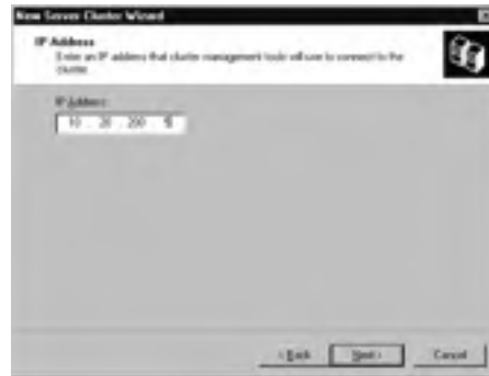
Figure 9.34 Enter the Cluster IP Address
