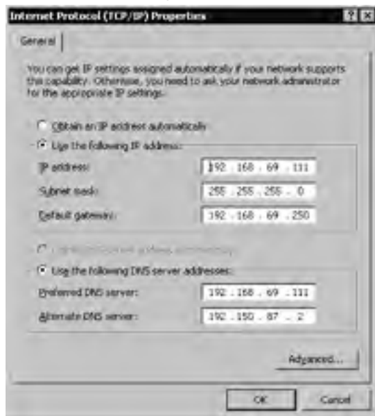
Figure 3.4 Internet Protocol (TCP/IP) Properties after Manual Configuration
