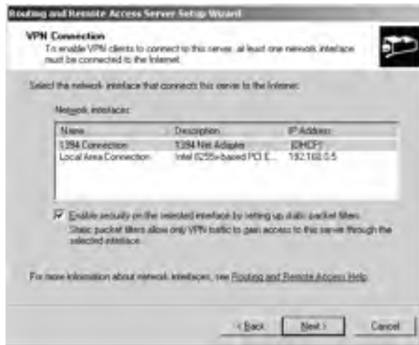
Figure 4.45 Choose the Interface Connected to the Internet
