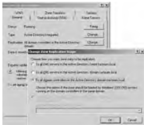
Figure 6.8 Changing Replication Scope for Windows Server 2003 Active Directory-integrated Zones
