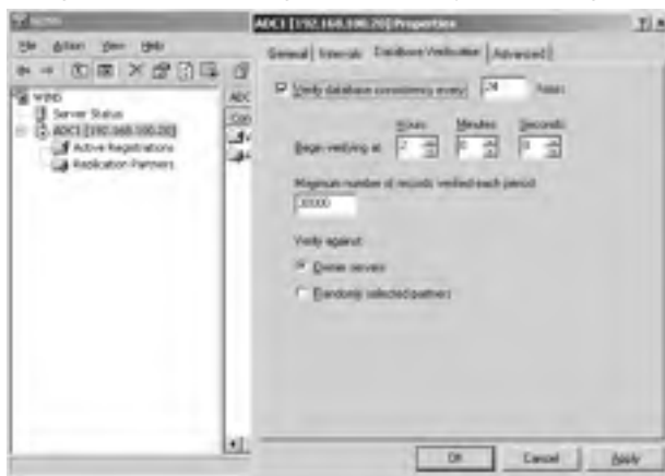
Figure 6.36 Enabling and Scheduling Consistency Checking
