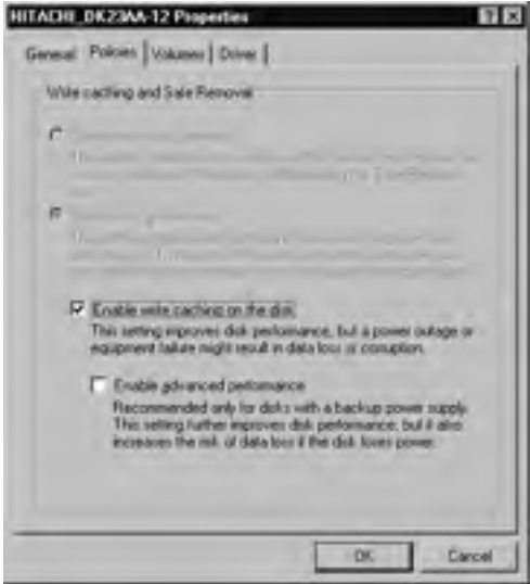
Figure 9.18 Disabling Write Caching on a Drive through Device Manager
