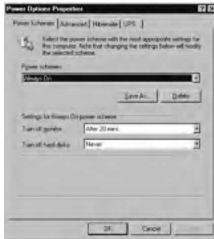
Figure 9.20 Enabling the Always On Power Scheme
