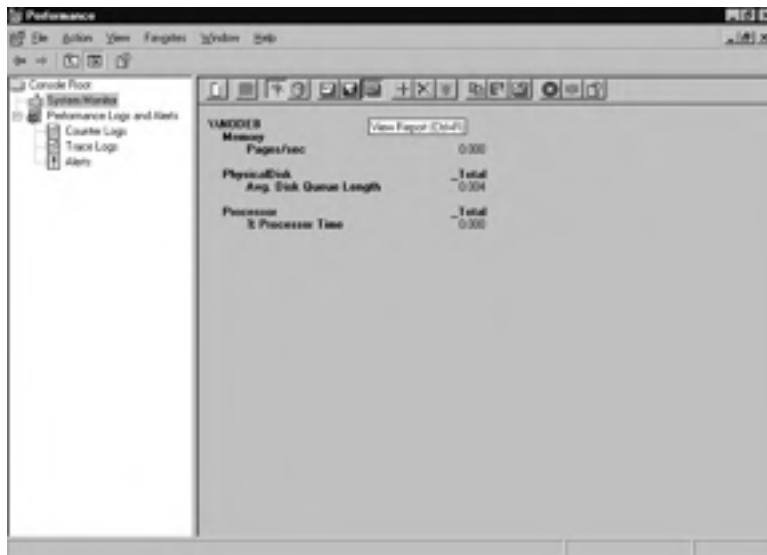
Figure 8.4 System Monitor, Report View with Default Counters
