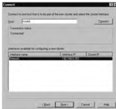
Figure 9.58 Connect to an NLB Node
