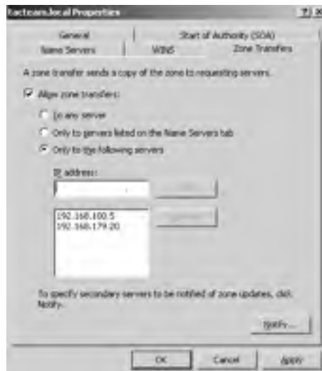
Figure 6.20 Configuring a Primary Zone with a List of Secondaries Authorized to Do Zone Transfers
