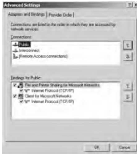
Figure 9.25 Setting the Proper Binding Order of Interfaces
