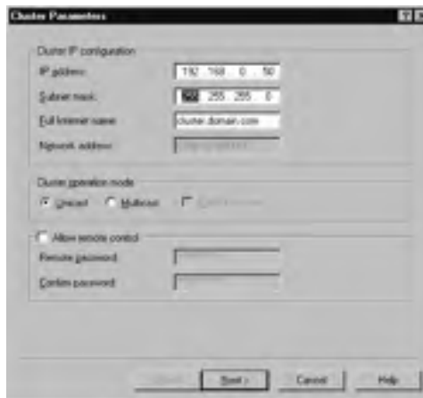
Figure 9.51 Configure Cluster Parameters
