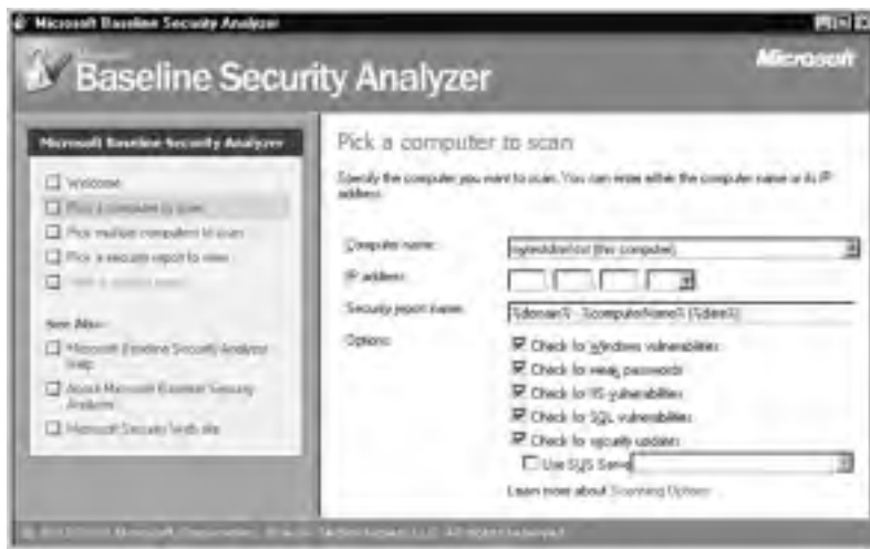
Figure 11.6 Select a Computer to Scan Using MBSA
