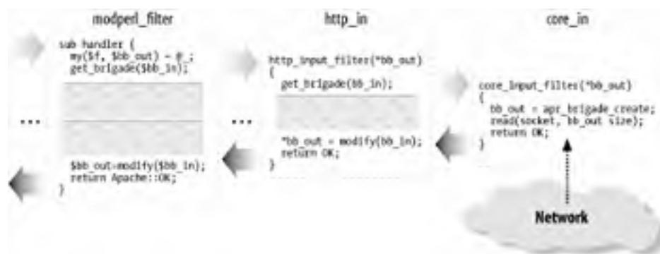
Figure 25-5. mod_perl 2.0 input filter program control and data flow
