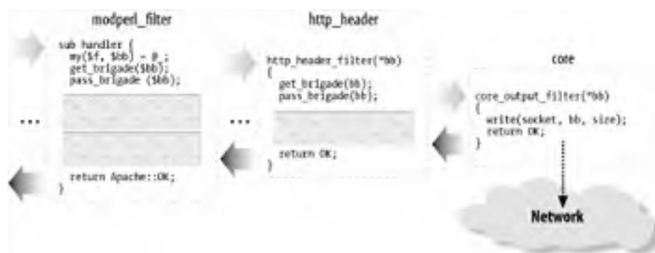
Figure 25-6. mod_perl 2.0 output filter program control and data flow
