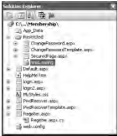
Figure 21-3. The folder and file structure of a web application with a secured area
