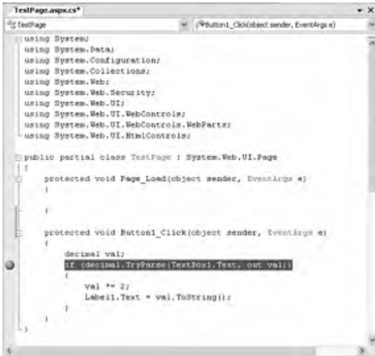
Figure 2-22. Setting a breakpoint
