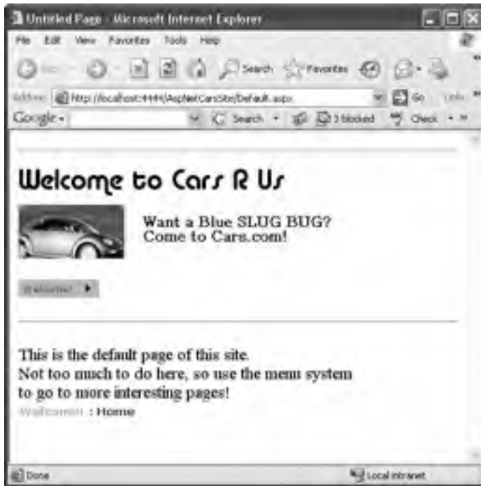
Figure 26-12. At runtime, master files and content pages render back a single <form>.
