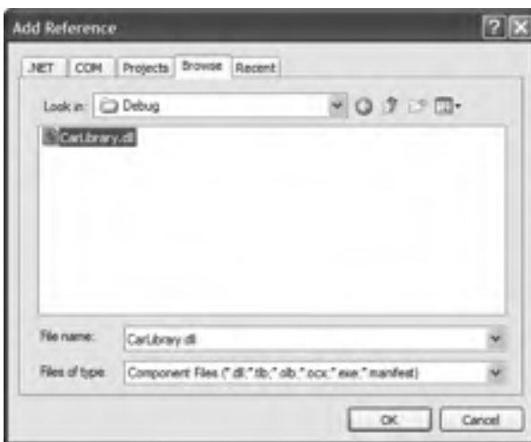
Figure 13-23. Correct! You must reference shared assemblies by navigating to the project's \bin\Debug directory using Visual Studio 2005.
