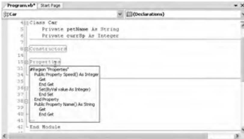
Figure 11-1. Code regions allow you to define a set of collapsible code statements.
