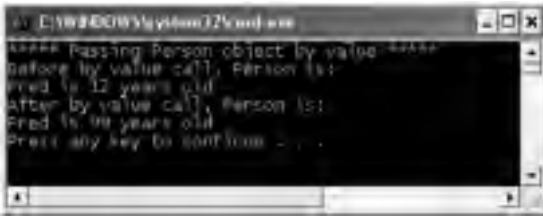
Figure 11-6. Passing reference types by value “locks” which object the reference points to.
