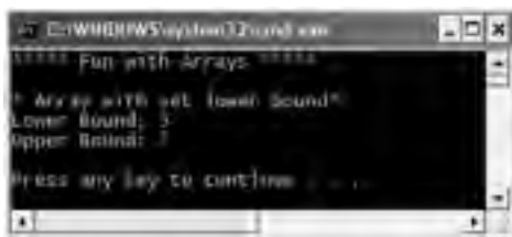
Figure 4-5. Creating an array with a lower bound of 5 using VB 2005
