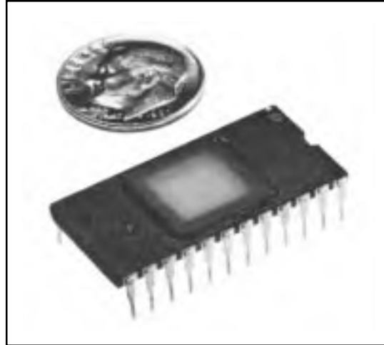
Figure 5-3. A 4K by 8 bits EPROM memory chip.
