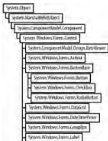
Figure 7-1. Control class hierarchy
