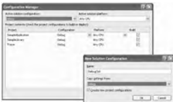
Figure 4-15: The Configuration Manager main window (left) and the dialog box that lets you define a new solution and project configuration (right)
