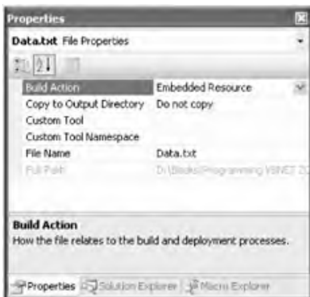
Figure 17-10: The properties of a file, which include the action to be performed at build time (can be None, Compile, Content, or Embedded Resource)
