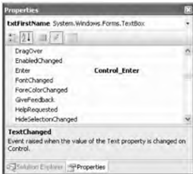
Figure 7-1: The Event tab in the Properties window, which displays all the events that the currently selected control exposes
