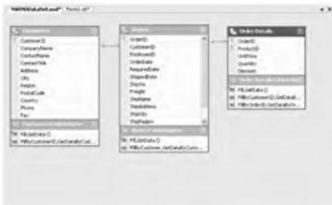
Figure 19-6: For each DataTable in the DataSet, you can define one or more custom commands, such as FillByCustomerID .
