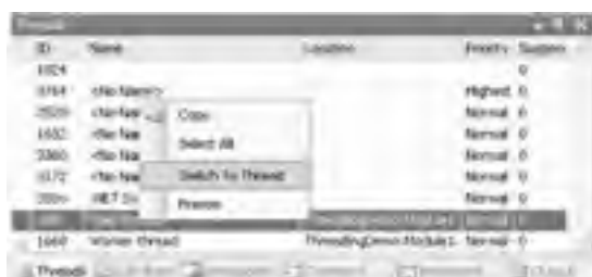
Figure 20-4: The Threads window, which lists all threads and lets you freeze and restart them
