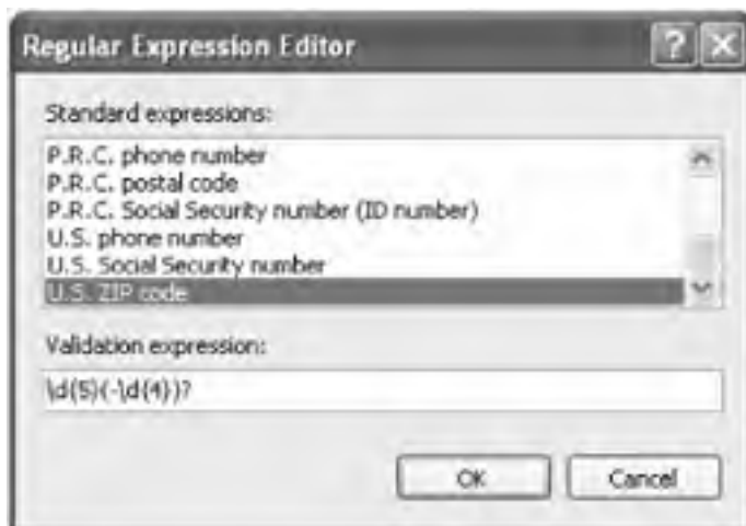
Figure 14-2: Setting the ValidationExpression property of a RegularExpressionValidator ASP.NET control by selecting one of the common regular expressions you find in the Regular Expression Editor dialog box
