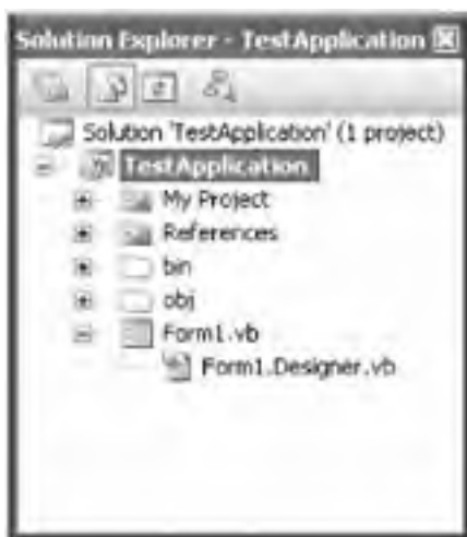
Figure 2-2: Source files containing automatically generated code, which appear in the Solution Explorer only if you select the Show All Files option on the toolbar
