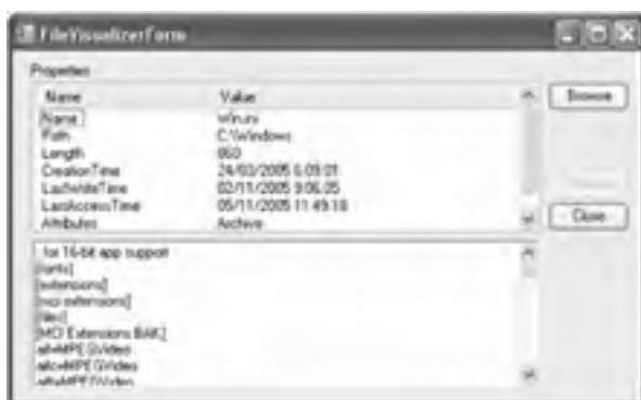
Figure 5-7: The custom file visualizer displays a file's properties and contents and even enables you to browse other files.
