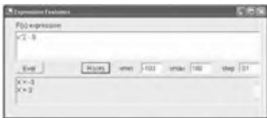
Figure 18-3: The demo application, which uses on-the-fly compilation to evaluate functions and find the roots of any equation that uses the X variable
