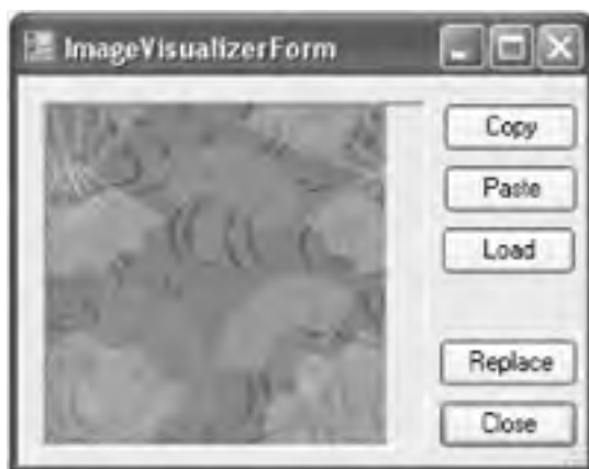
Figure 5-8: The custom image visualizer, which lets you copy and paste the image, select a different image from disk, and return a different bitmap object to the project being debugged
