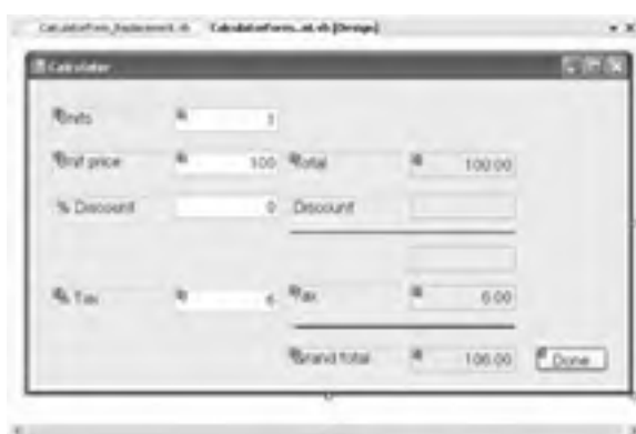
Figure 19-3: The new SamplePlugin project, which extends the CalculatorForm to account for a discount percentage
