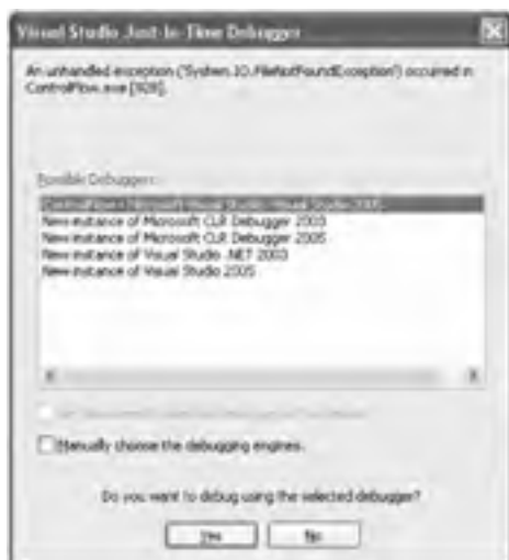
Figure 3-1: The dialog box that appears when an unhandled exception is thrown and one or more .NET debuggers are installed on the computer
