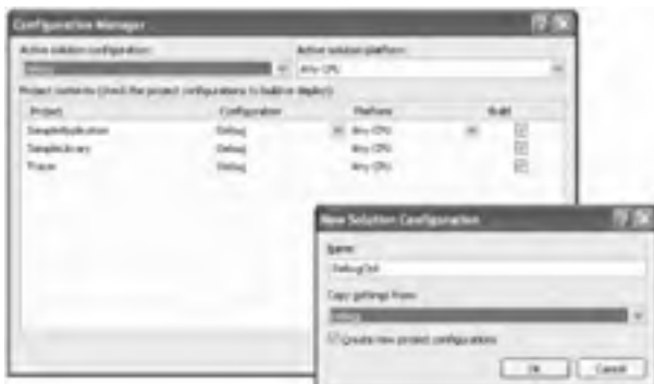
Figure 4-15: The Configuration Manager main window (left) and the dialog box that lets you define a new solution and project configuration (right)
