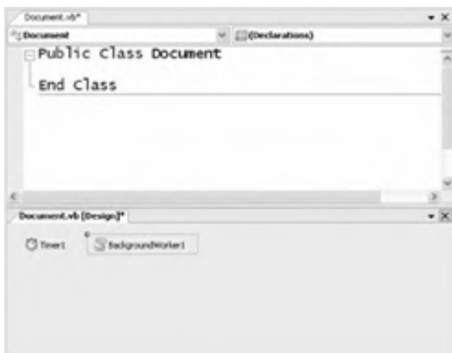
Figure 17-3: A component has a code editor and a designer surface; you can display both at the same time by using the New Horizontal Tab Group command on the Window menu.
