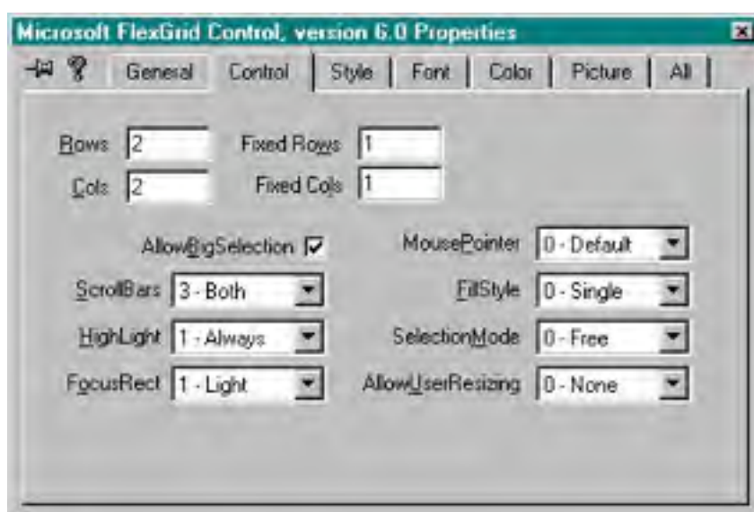
Figure 30-7. Microsoft Visual C++ inserting the Microsoft FlexGrid 6.0 property pages into its own dialog box for editing resource properties.
