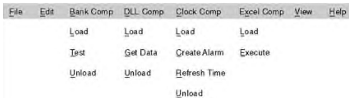
Figure 25-7. A sample menu structure for a standard SDI application.
