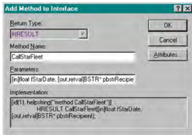
Figure 29-5. Adding a method to an interface.
