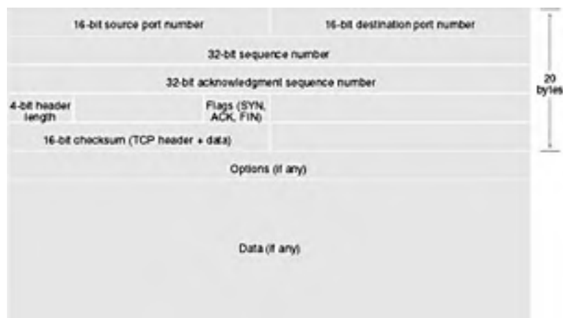
Figure 34-6. A simple layout of a TCP segment.
