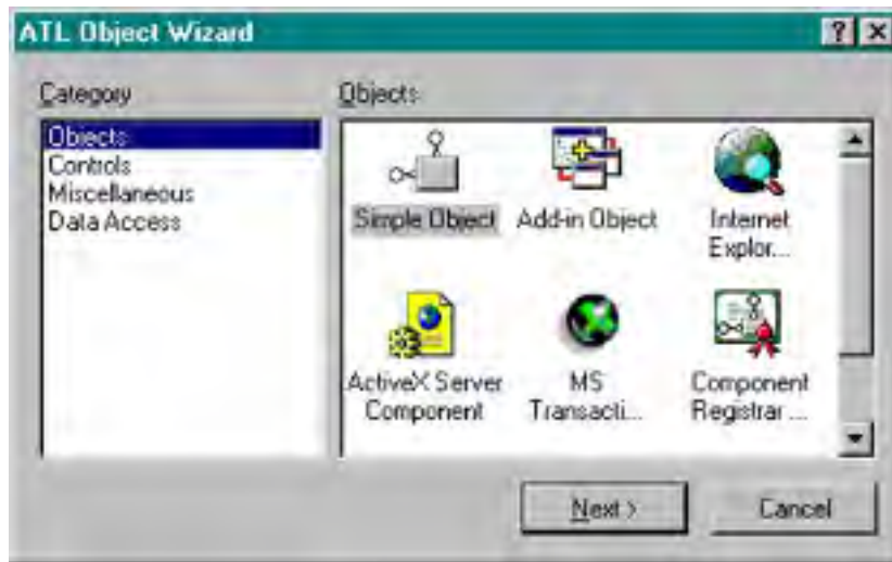
Figure 29-3. Using the ATL Object Wizard to insert a new ATL-based COM class into the project.
