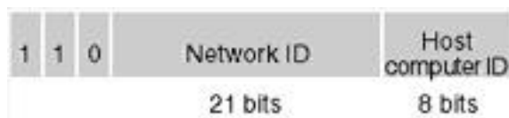
Figure 34-5. The layout of a Class C IP address.
