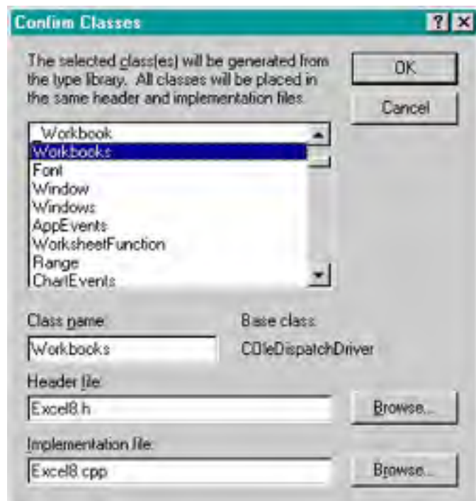
Figure 25-11. ClassWizard can create C++ classes for the Excel objects listed in Excel8.olb .
