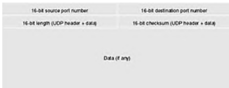
Figure 34-3. A simple UDP layout.
