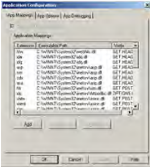
Figure 34-6: The Application Configuration property sheet within IIS showing the list of file-to-ISAPI DLL mappings.
