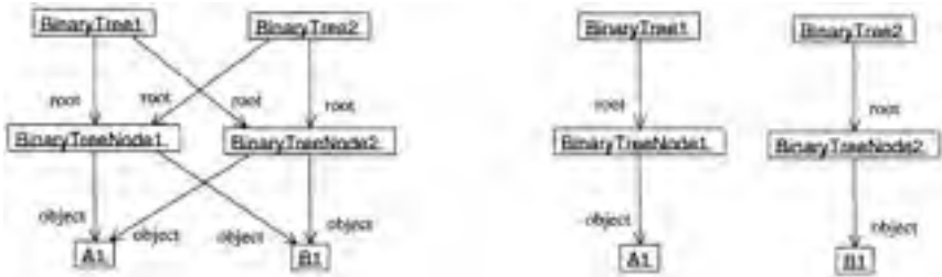
Fig. 4.7. Object diagram computed by an object insensitive analysis (left) and by an object sensitive analysis (right).
