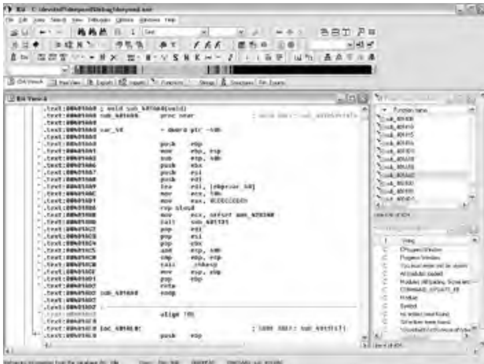
Figure 4.2 A typical IDA Pro screen, showing code disassembly, a function list, and a string list.
