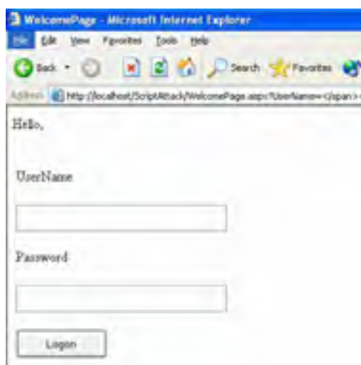
Figure 6-1: The user name and password fields injected by the attacker's user name
