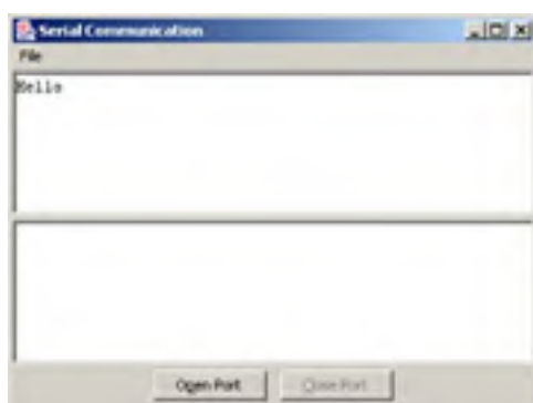
Figure 5-5: Sending Data Using the Serial Communication Application
