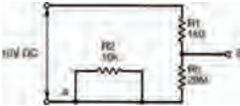
Figure 10.2 Equivalent diagram of a single transistor switch, with the transistor base (point A in Figure 10.1) connected to logic 0
