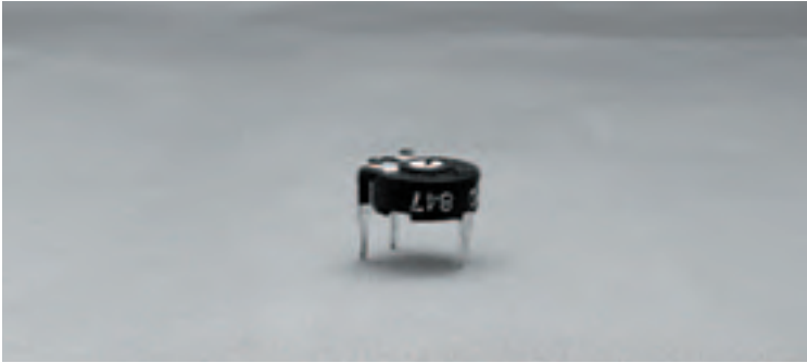
Photo 6.1 A horizontal preset resistor
