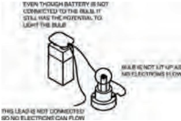
Figure 1.4 Even when the battery is disconnected and electrons do not flow, the battery still has a potential difference
