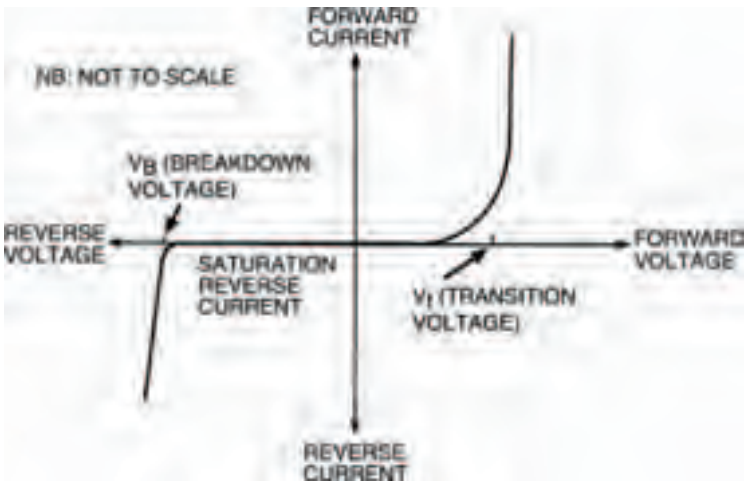
Figure 6.14 Plotting the reverse bias characteristics for an ordinary diode is not practical, so we give you the characteristic curve here
