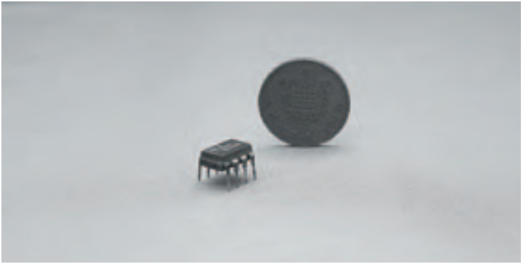
Photo 5.5 The 555, an 8 pin DIL timer IC, beside a UK one penny piece
