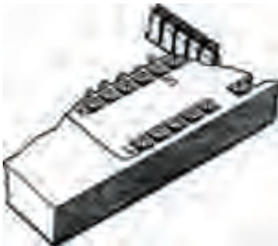
Figure 2.1 The interior of a breadboard, showing the contacts
