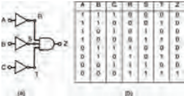
Figure 10.47 A three input AND gate converted to a NOR gate with NOT gates
