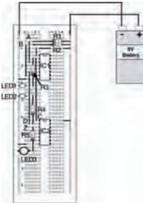
Figure 10.44 A breadboard layout for the circuit in Figure 10.43
