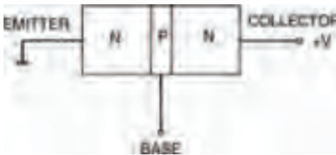
Figure 8.4 Connected up, the emitter is at 0V and the collector is positive
