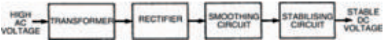
Figure 7.15 A block diagram of a power supply using the circuit stages we have described
