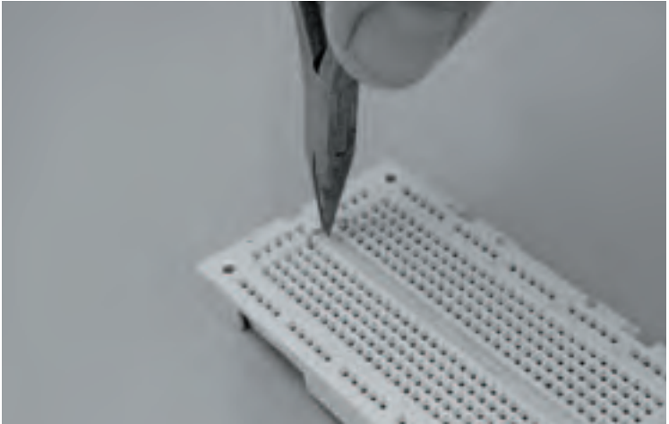
Photo 5.3 The wire link you have made should drop neatly into the breadboard
