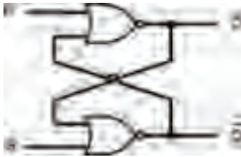
Figure 11.3 An SR-type bistable circuit, comprising two cross-coupled NOR gates
