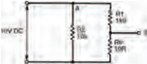
Figure 10.3 Equivalent diagram of a single transistor switch, with point A connected to logic 1
