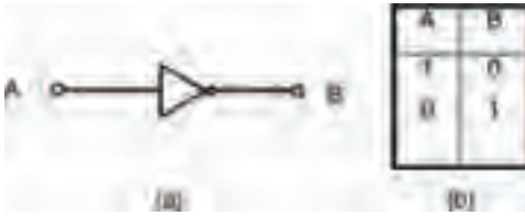
Figure 10.9 (a) the symbol for an inverter or NOT gate; (b) its truth table
