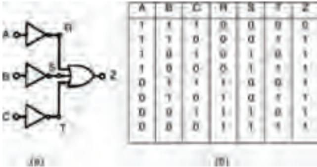
Figure 10.42 (a) a NAND gate, made from OR and NOT gates; (b) its truth table, to prove this
