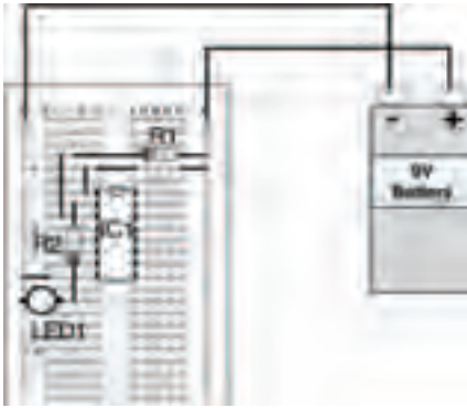
Figure 10.7 Possible breadboard layout of the circuit in Figure 10.6
