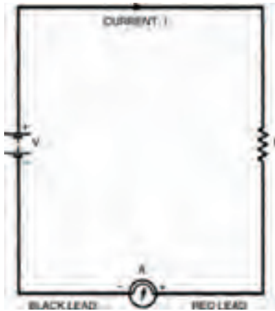
Figure 3.7 The meter connected to a different part of the circuit. The effect is the same as long as the red lead is correctly connected
