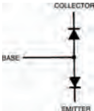
Figure 8.2 A symbol for a transistor considered as two diodes, back to back
