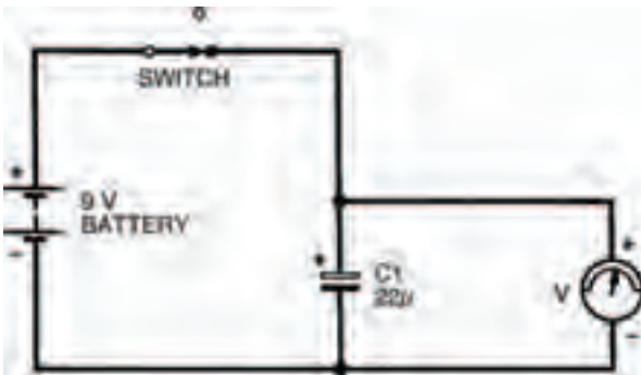
Figure 4.11 An experimental circuit to demonstrate how a capacitor stores voltage (or charge)
