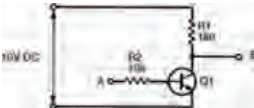
Figure 10.1 A simple transistor used as a switch, to form a simple digital circuit
