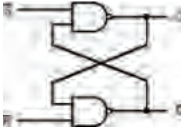
Figure 11.5 An SR-type bistable circuit comprising two cross-coupled NAND gates — note the inverted inputs when compared with Figure 11.3
