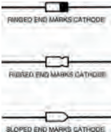
Figure 6.2 Some typical diode body shapes
