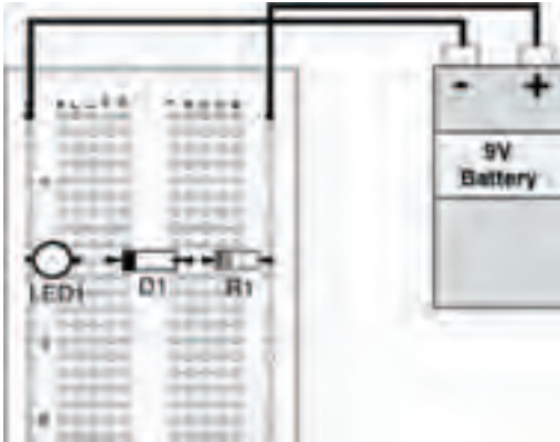
Figure 6.4 A breadboard layout for the circuit in Figure 6.3
