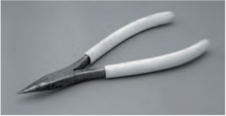
Photo 1.2 Snipe-nosed pliers – ideal for electronics work and another essential tool
