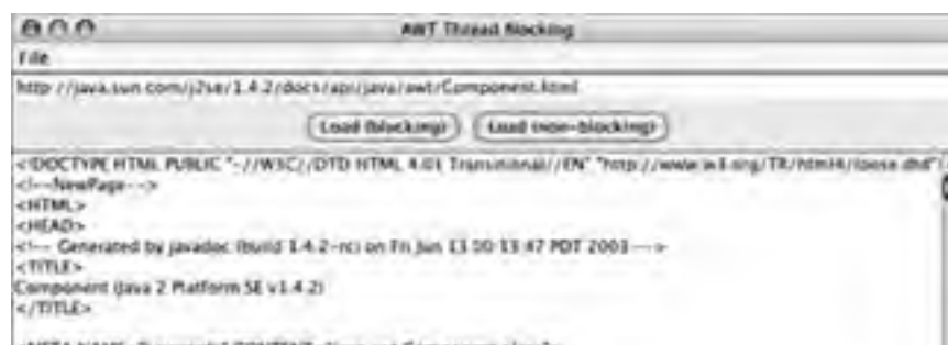
Figure 12-7. Blocking and not blocking AWT event dispatch by loading a URL into a JTextArea
