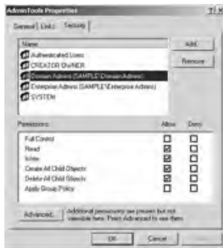
FIGURE 5.6 The Security tab of the GPO's Properties dialog box, with default settings
