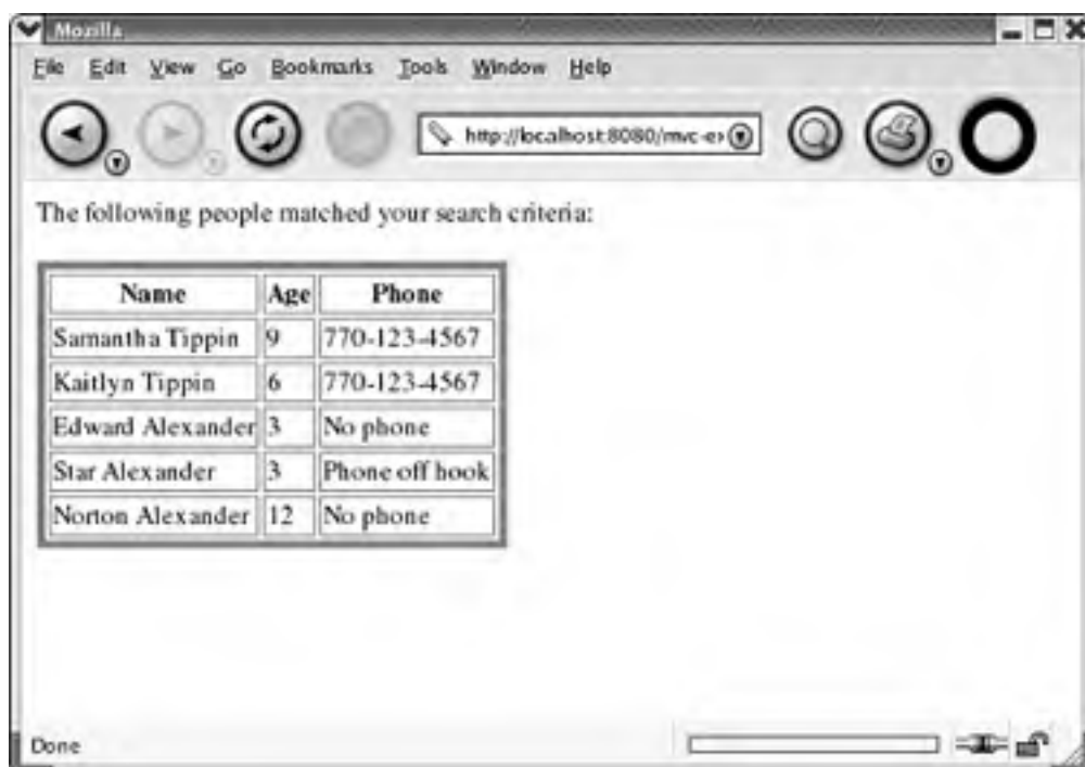
Figure 20.4. The View page is responsible for displaying the data retrieved from the model.
