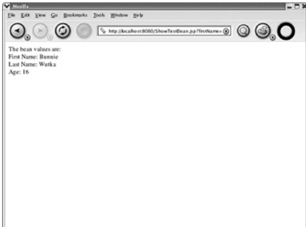
Figure 14.2. The jsp:setProperty action makes it easy to set several bean properties from request parameters.
