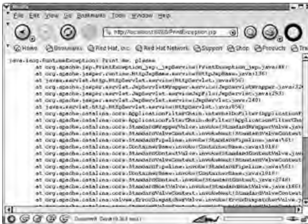
Figure 8.1. You can create a PrintWriter to print a stack trace to the browser.
