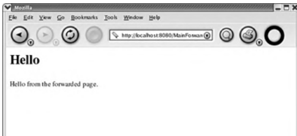
Figure 10.4. When a JSP forwards to another JSP, the output from the original JSP is lost.
