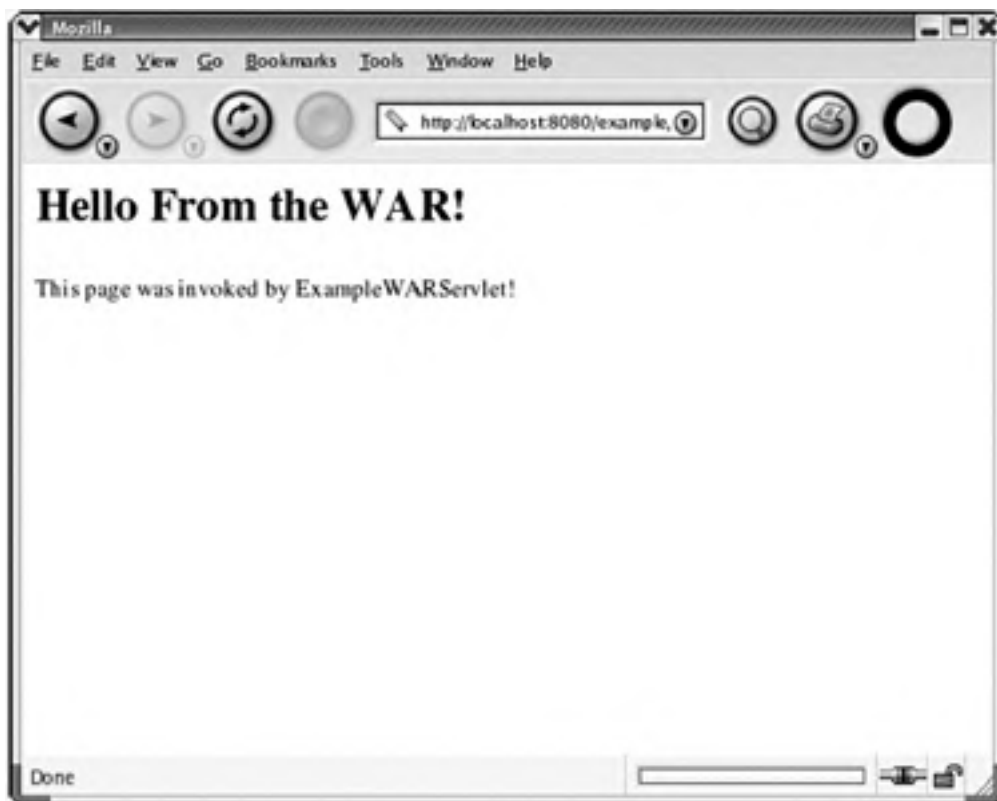
Figure B.1. Tomcat automatically assigns the application name based on the WAR filename.
