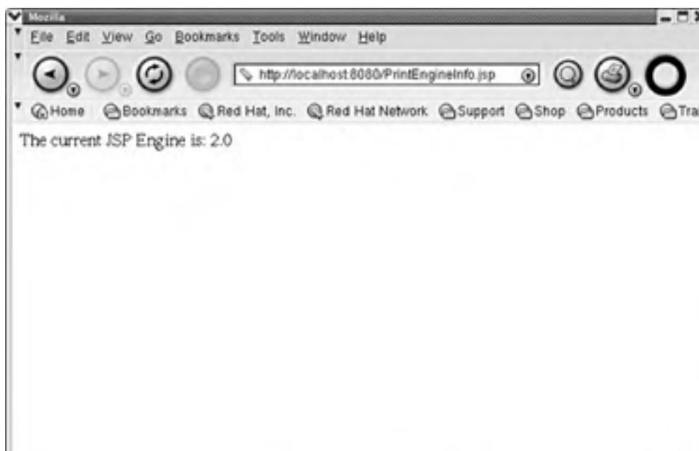
Figure 8.3. You can get the supported JSP version number from the JSP engine.
