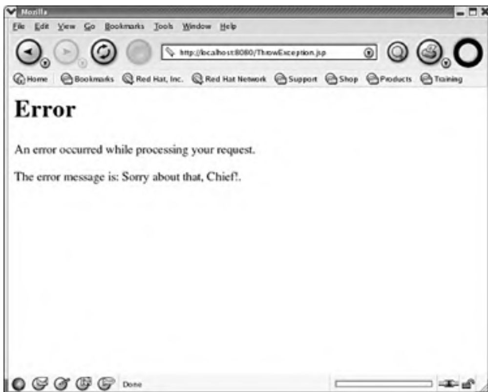
Figure 9.2. The JSP engine clears the output buffer, if possible, before displaying an error page.
