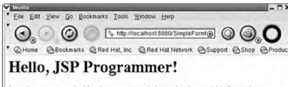
Figure 3.2. A JSP can read form input and embed the form data in its output.
