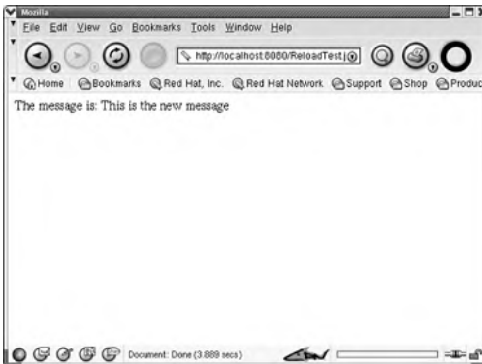
Figure 5.3. When the JSP engine is restarted, it picks up the changed ReloadedClass class.
