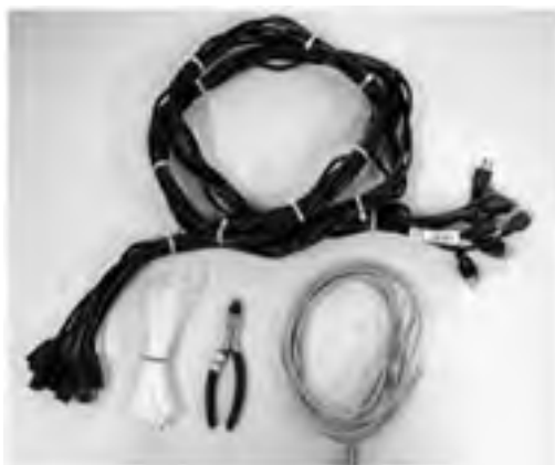
Figure 6.1: Cable bundles. Wire ties make 8 power cables into a neat and manageable group
