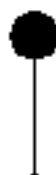
Figure 3-2 The solid circle is called an initial node —or activity diagram starting point—and the directed arrow is called a control flow .
