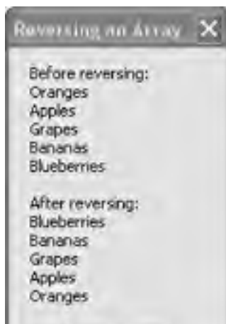
Figure 8-3. Reversing the contents of an array with the shared Array.Reverse() method
