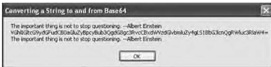
Figure 5-51. A sample string converted to Base64 and back again
