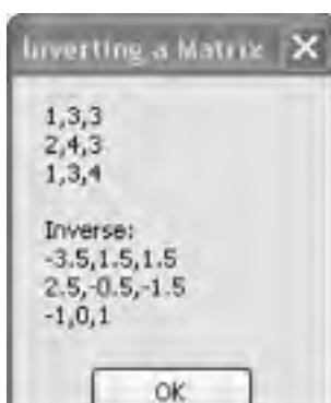
Figure 6-32. Finding the inverse of a square matrix with the MatrixHelper.Inverse() function
