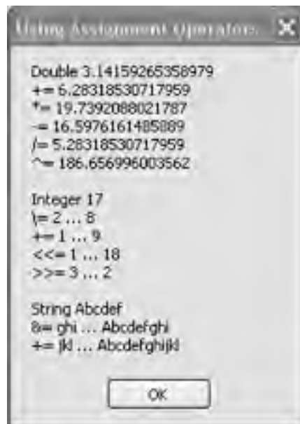
Figure 6-1. The compact assignment operators in action
