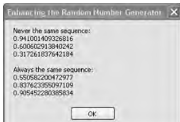
Figure 6-26. Two pseudorandom sequences are generated: one that's always unique and one that always repeats
