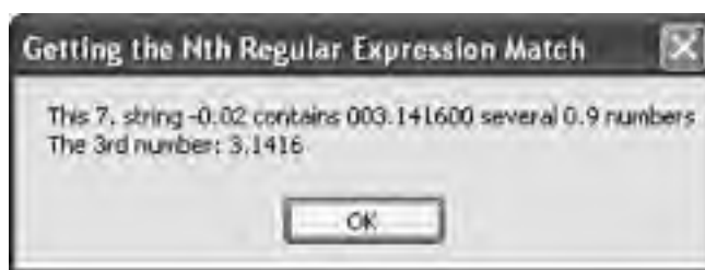
Figure 5-44. Using a regular expression to find the nth match in a string
