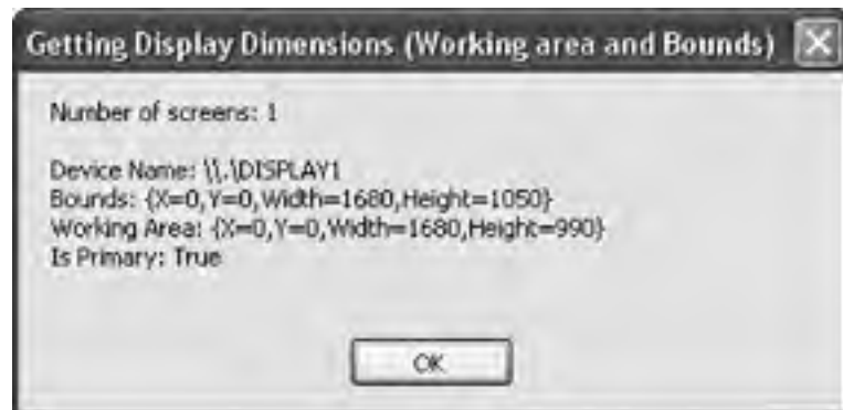
Figure 10-25. The Screen.AllScreens array provides information about any monitors on your system
