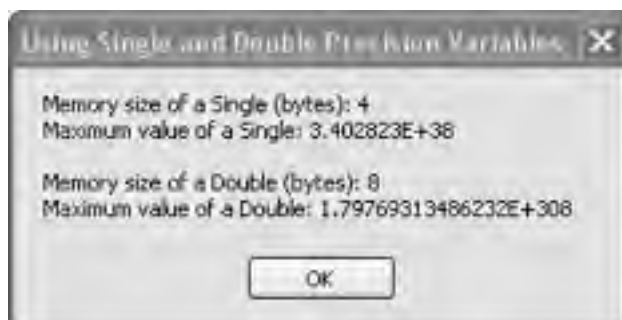
Figure 6-5. Singles and Doubles require a different amount of memory and hold different-sized numbers
