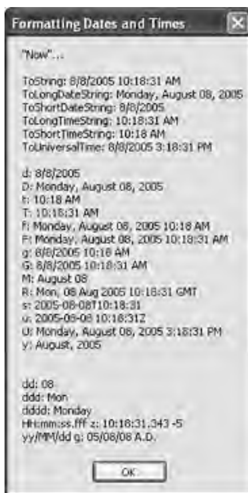
Figure 7-10. A sampling of predefined and custom formats available for formatting Date variables to strings
