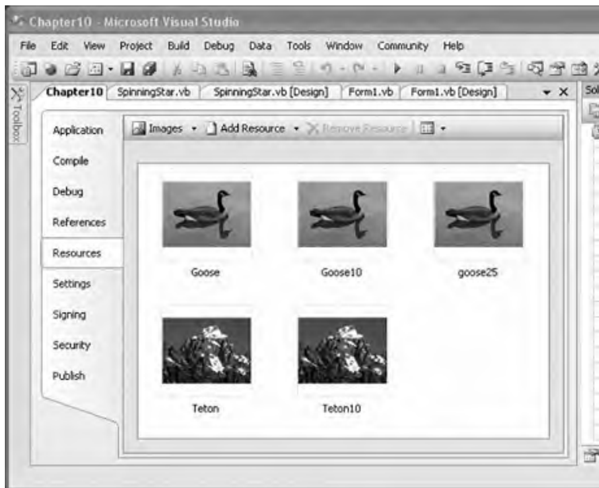
Figure 10-21. Resource-maintenance tasks are carried out on the Resources Properties window
