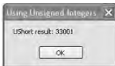
Figure 6-3. Unsigned integer variables can hold bigger numbers than signed integers, in the same amount of memory
