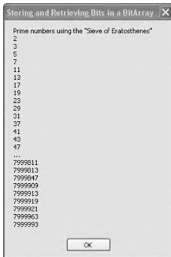
Figure 6-25. All the prime numbers between 0 and 8,000,000, calculated quickly using a BitArray
