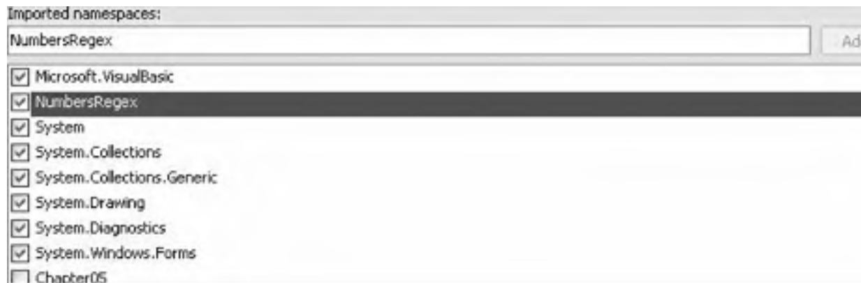
Figure 5-46. Importing a namespace via the Project Properties window
