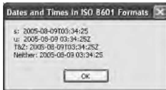
Figure 7-23. Date and time strings that closely conform to the ISO 8601 standard
