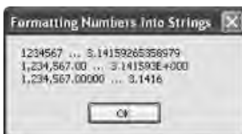
Figure 5-22. A sampling of the many ways numbers can be formatted into strings
