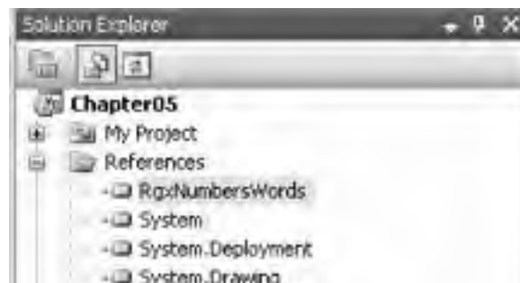
Figure 5-45. The DLL file named RgxNumbersWords added to the References list in Solution Explorer
