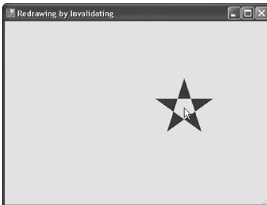
Figure 9-13. As the mouse moves the form is invalidated, causing the star to move with the cursor
