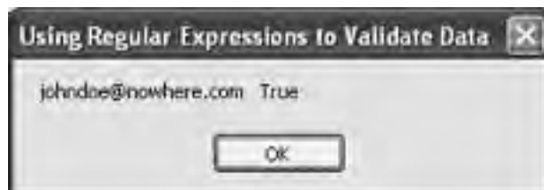
Figure 5-48. A string that passes the regular expression test for valid email addresses
