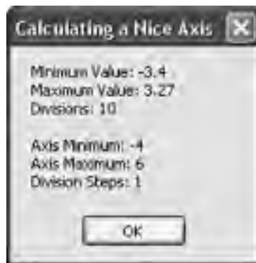
Figure 9-32. The NiceAxis() function returns end points and the division step size for a nicely scaled chart axis
