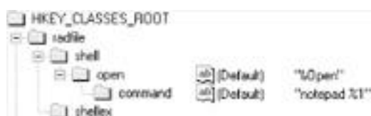
Figure 4.2. Registry entry for static "Open" context menu
