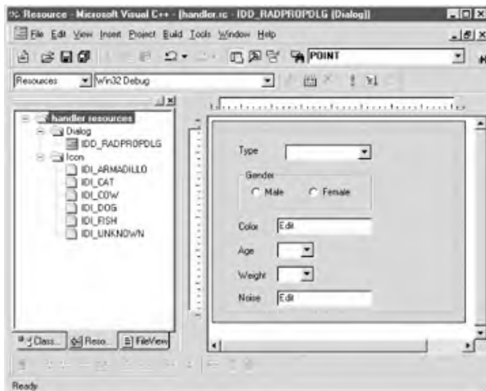
Figure 6.4. Creating a dialog template with Visual C++ resource editor
