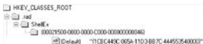
Figure 10.2. Registering InfoTip handler
