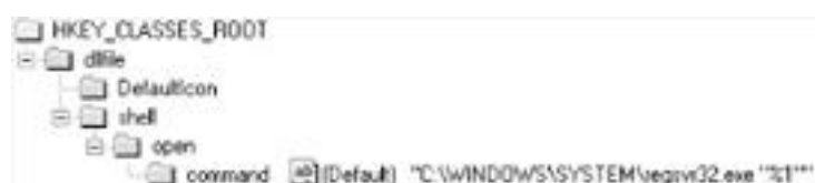
Figure 3.8. Associating regsvr32.exe with the dllfile file type
