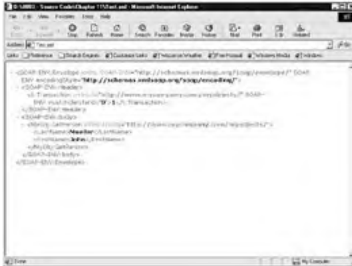
Figure 11-2: Internet Explorer versions 5.5 and above can display SOAP messages in a simple format.
