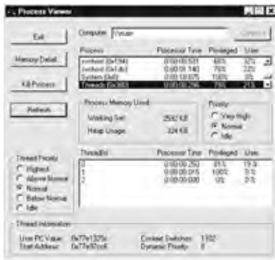
Figure 3-2: The Process Viewer shows which threads are executing and how much processor time they're using.
