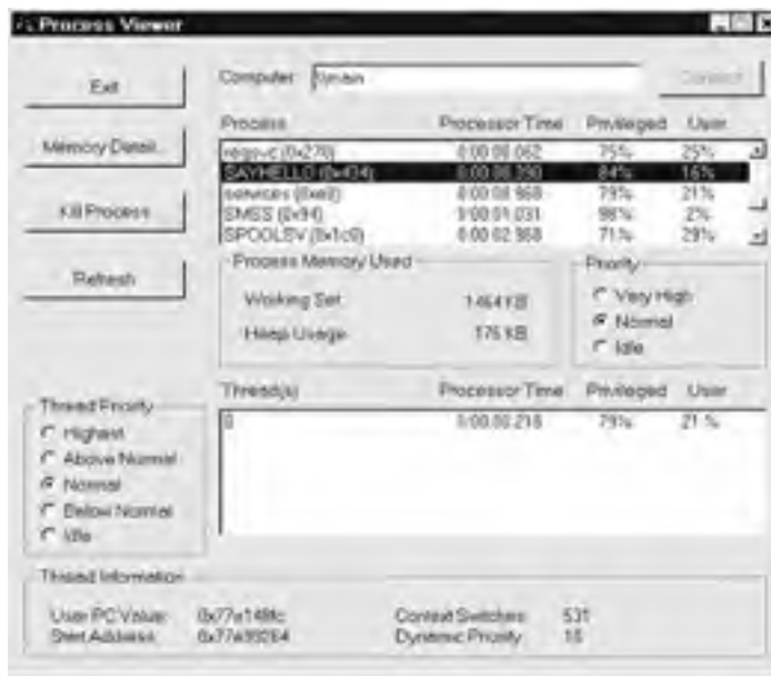
Figure 1-9: The Process Viewer allows you to see what processes are currently executing on your machine.
