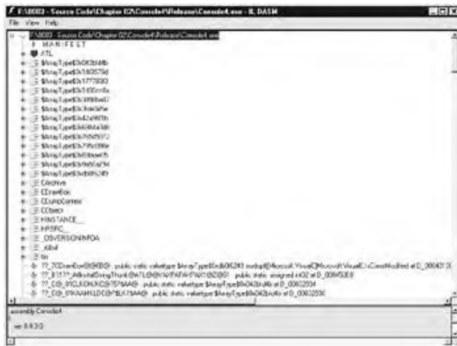
Figure 2-2: Use ILDASM to learn more about managed code in Visual C++ .NET.
