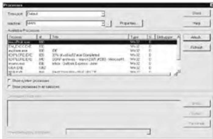
Figure 1-3: The Processes dialog box allows you to attach the debugger to an application that's already running on a local or remote machine.
