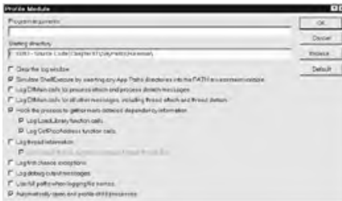
Figure 1-6: The Profile Module dialog box allows you to add a command line argument and adjust the kinds of information that Depends will track.
