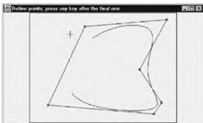
Figure 4.18: B-spline curve consisting of five curve segments
