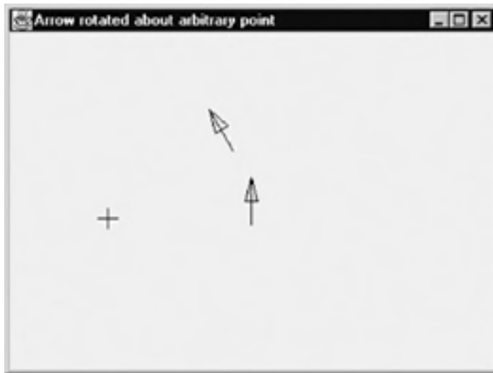
Figure 3.5: Arrow before and after rotation through 30° about a point selected by the user
