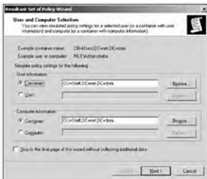
Fig. 15.5: Selecting user and computer objects for which policy settings will be simulated
