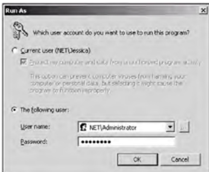
Fig. 8.1: By entering proper credentials in this window, you can start a program on behalf of another user
