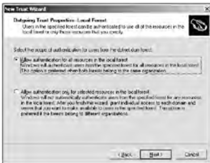
Fig. 5.17: On this page, you will select the authentication scope for users from the target forest
