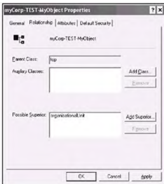
Fig. 7.34: This window allows you to add auxiliary classes to a class and to define containers (possible superiors), in which objects of that class can be created
