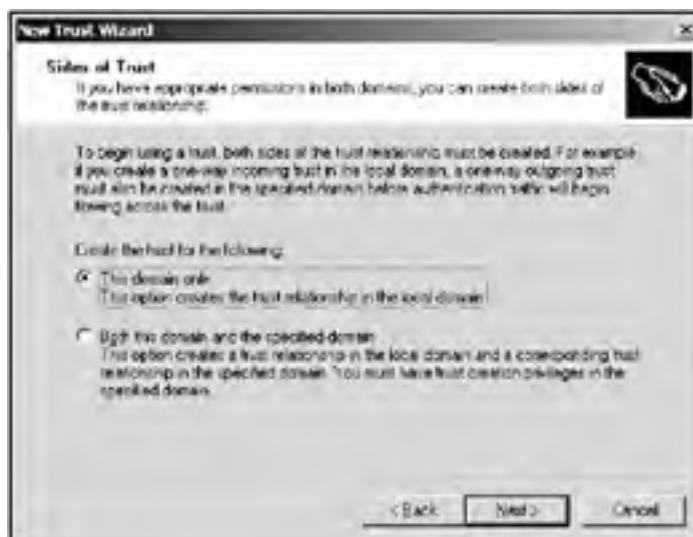
Fig. 5.14: You can create a trust in either the local domain only or both domains at the same time
