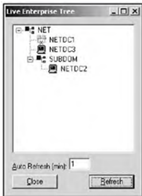
Fig. 12.10: In this window, you can see the entire domain structure (the forest) and the state of all DCs
