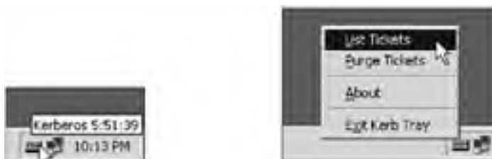
Fig. 14.1: The Kerberos Tray tool displays the time left on the initial TGT before it expires (left); the tool's context menu (right) allows you to select an operation
