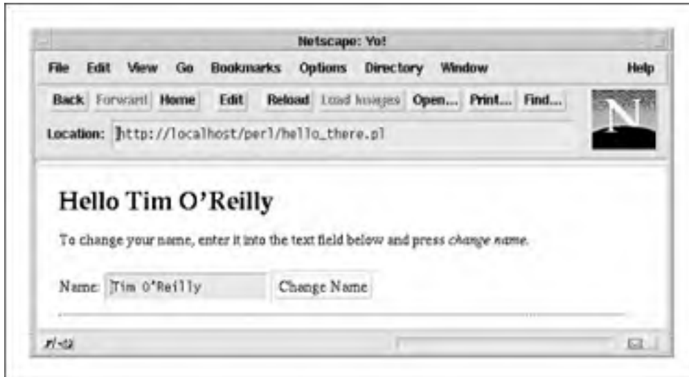
Figure 2.7. The Apache::Registry script generates a fill-out form to accept and process user input.
