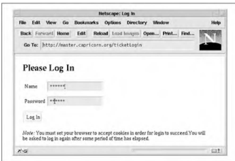
Figure 6.4. The custom login screen shown by the ticket master server prompts the user for a username and password.
