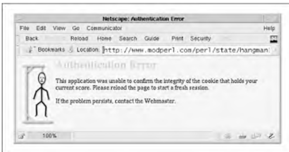
Figure 5.3. If the cookie fails to verify, the hangman3 script generates this error page.
