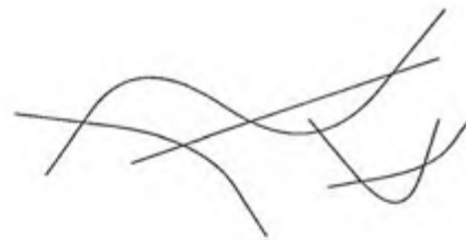
FIGURE 21.1.2 A simple arrangement of 5 bounded arcs, where s = 2 . It has 17 vertices (10 of which are arc endpoints), 19 edges, and 4 faces (one of which is unbounded).
