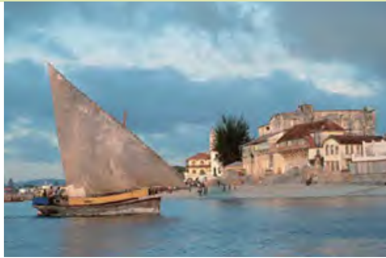
Dhow. This modern dhow in the harbor of Zanzibar displays the characteristic triangle sail. The triangle sail can make good use of the trade monsoon and thus has guided dhows on the Arabian Sea since ancient times.
