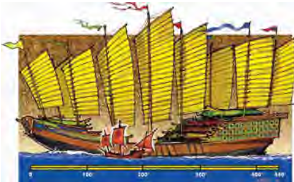
Zheng He's Ship. A testament to centuries of experience in shipbuilding and maritime activities, the largest ship in Zheng He's armada in the early fifteenth century was about five times the length of Columbus's Santa Maria (pictured next to Zheng's ship) and had nine times the capacity in terms of tonnage. It had nine staggered masts and twelve silk sails, all designed to demonstrate the grandeur of the Ming Empire.
