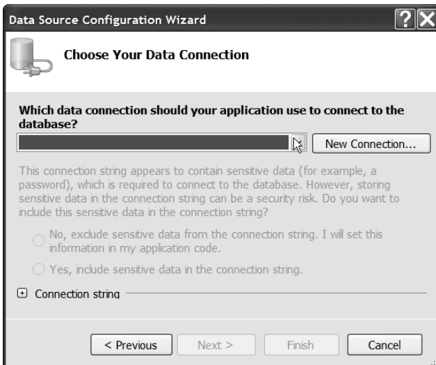
Figure 16-2. The second page lets you reuse connections you've established before or create a new one.
