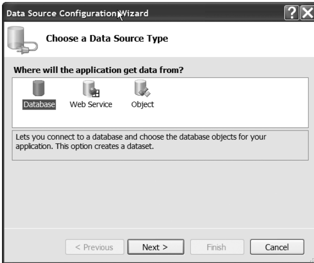
Figure 16-1. The first page of the Data Source Configuration Wizard lets you choose the type of object you want to get data from.
