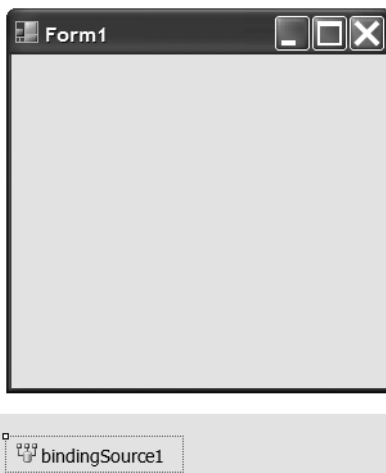
Figure 16-27. Adding a BindingSource control to the form is the first step in setting up bound controls.
