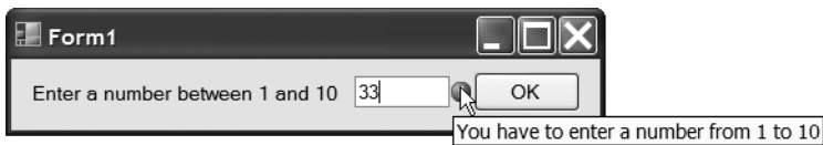
Figure 8-20. The ErrorProvider displays an error icon and a ToolTip containing the error message next to a control.
