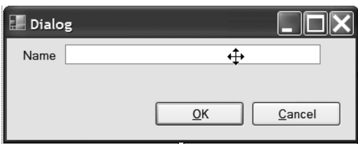
Figure 9-20. Design your dialog like this. Don't worry about giving the OK and Cancel buttons decent names, because they won't need any code.
