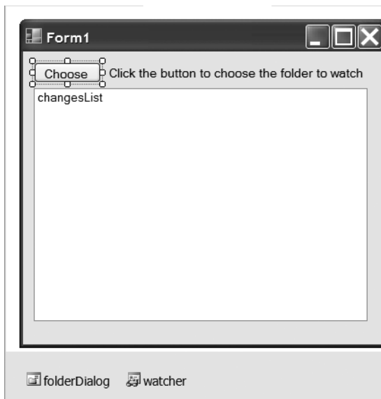
Figure 14-3. Arrange controls on your form like this. Note that FolderBrowserDialog and FileSystemWatcher are nonvisible controls and appear underneath the form in the editor.
