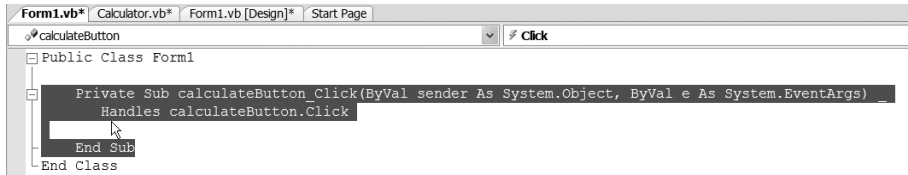
Figure 4-9. Double-clicking a control drops you into the code editor for its default, or standard, event. This event is itself a method.
