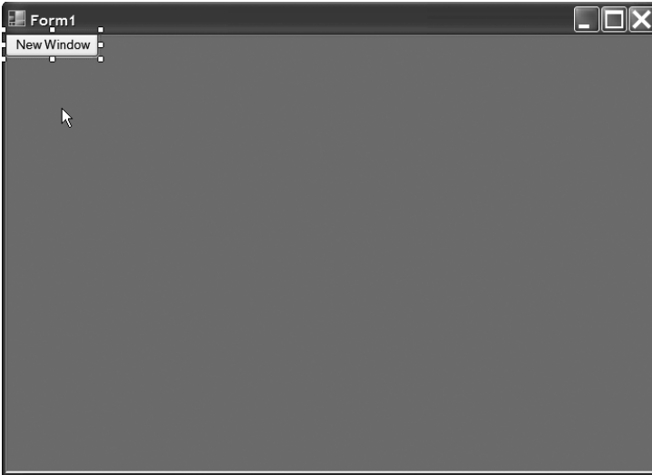
Figure 9-13. .NET lets you drop controls onto container forms, something that you couldn't do very easily before.
